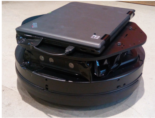
Figure 4.3: The Kobuki with the 3D camera and netbook.
