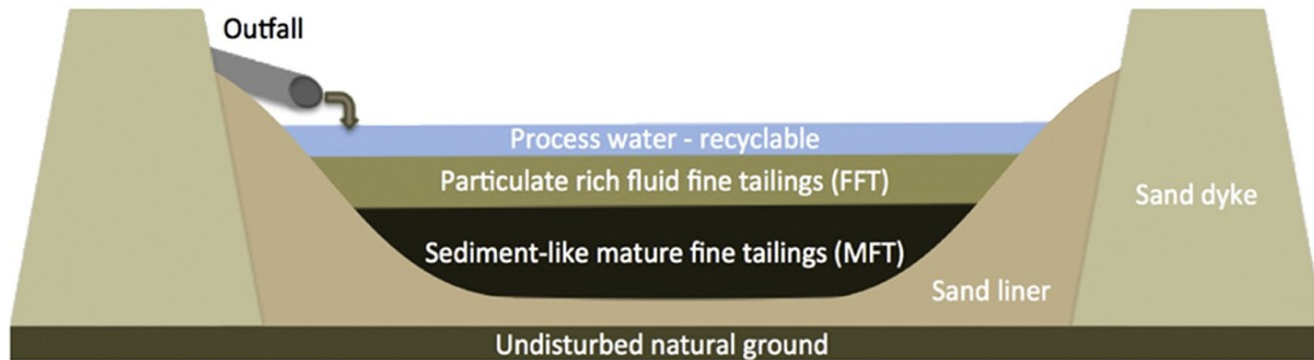
Figure 1: Profile of an Athabasca oil sands tailings pond, with coarse sand on the bottom layer, followed by mature fine tailings (MFT), fluid fine tailings (FFT), and OSPW on top, labeled in the source figure as ‘Process water – recyclable.’ Reproduced with permission from, source: Willis et al. 11 abstract image, p. 1604.
