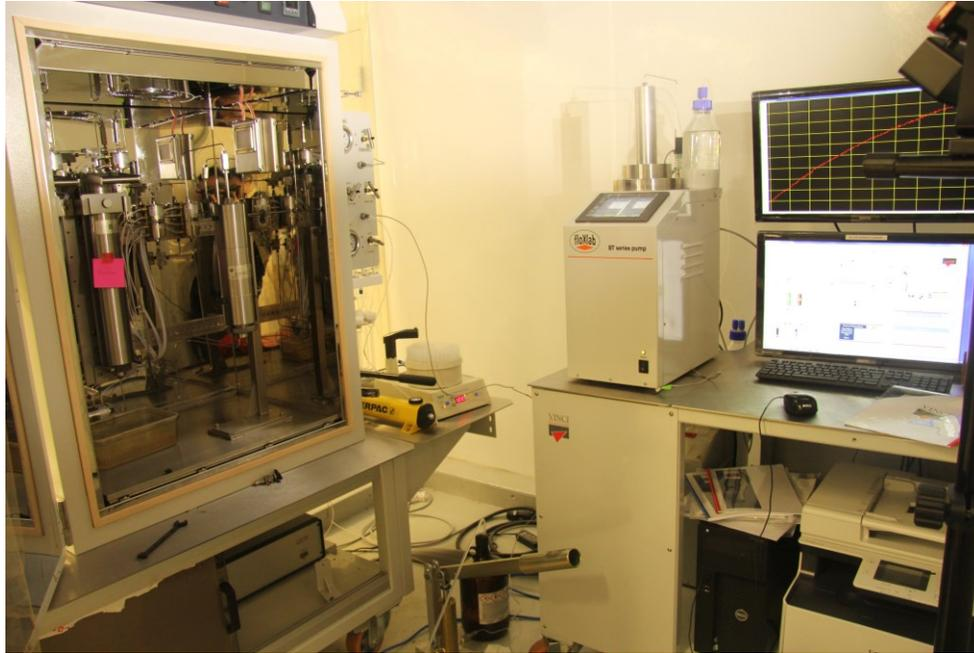
**Figure 5.1 Vinci core-flooding system**
