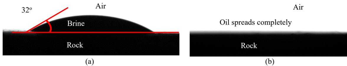
Figure 4.4 Air-liquid contact angles of (a) brine and (b) oil droplets on polished surfaces of MT-A1.
