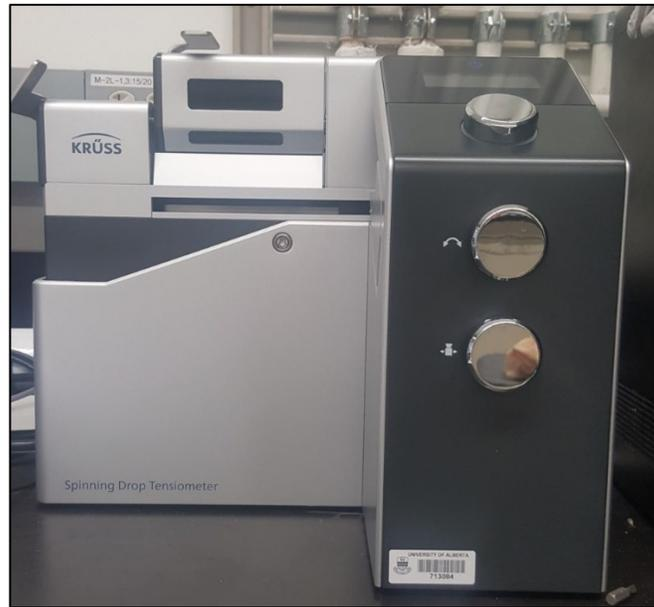
**Figure 5.5 Spinning drop tensiometer.**
