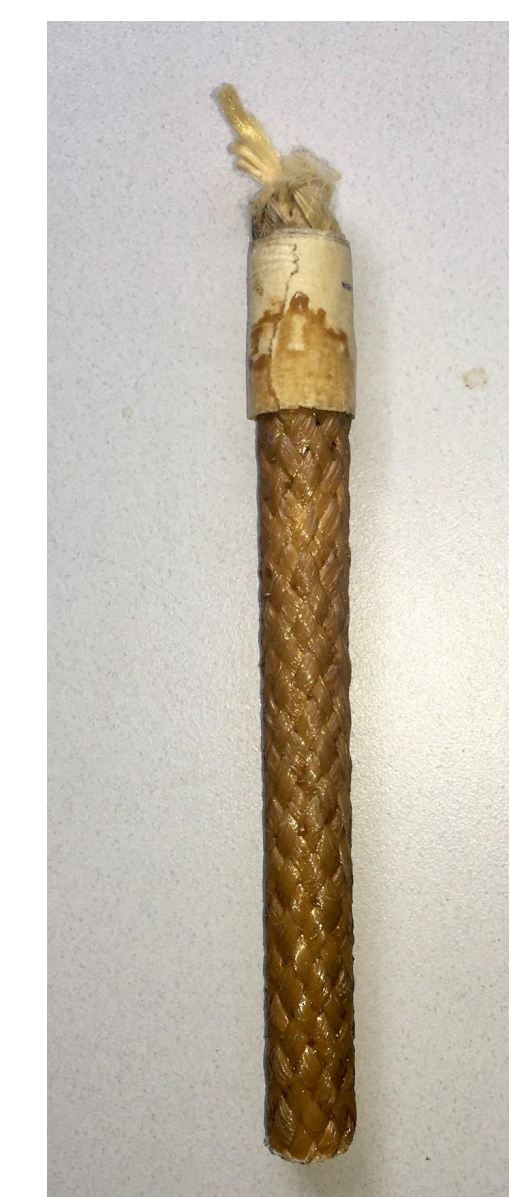
Figure 4: A sample of a cured braid of Kevlar
