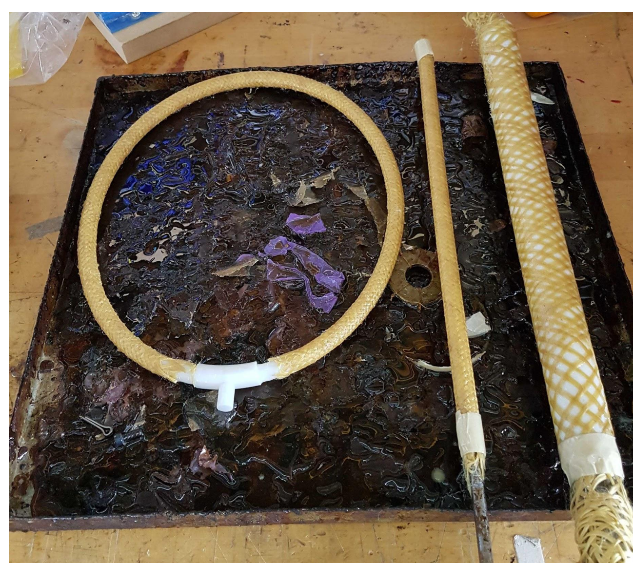
Figure 3: The resin application process of Kevlar braids on various curing mandrels
