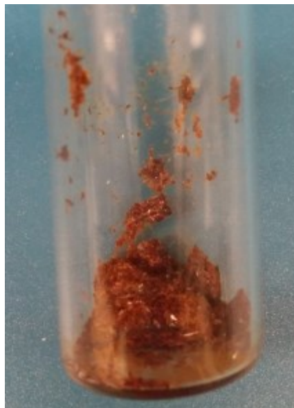
(b) Red color solid material after reaction time with DnBS and CH 3 I inside the reactor without any solvent (Set – 5)
