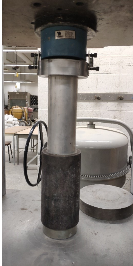
Figure E- 5 Overall setup for cement removal using loading frame
