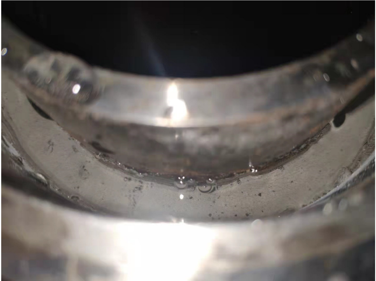
Figure 5- 9 Leakage detection result for the second cyclic pressure and constant temperature experiment
