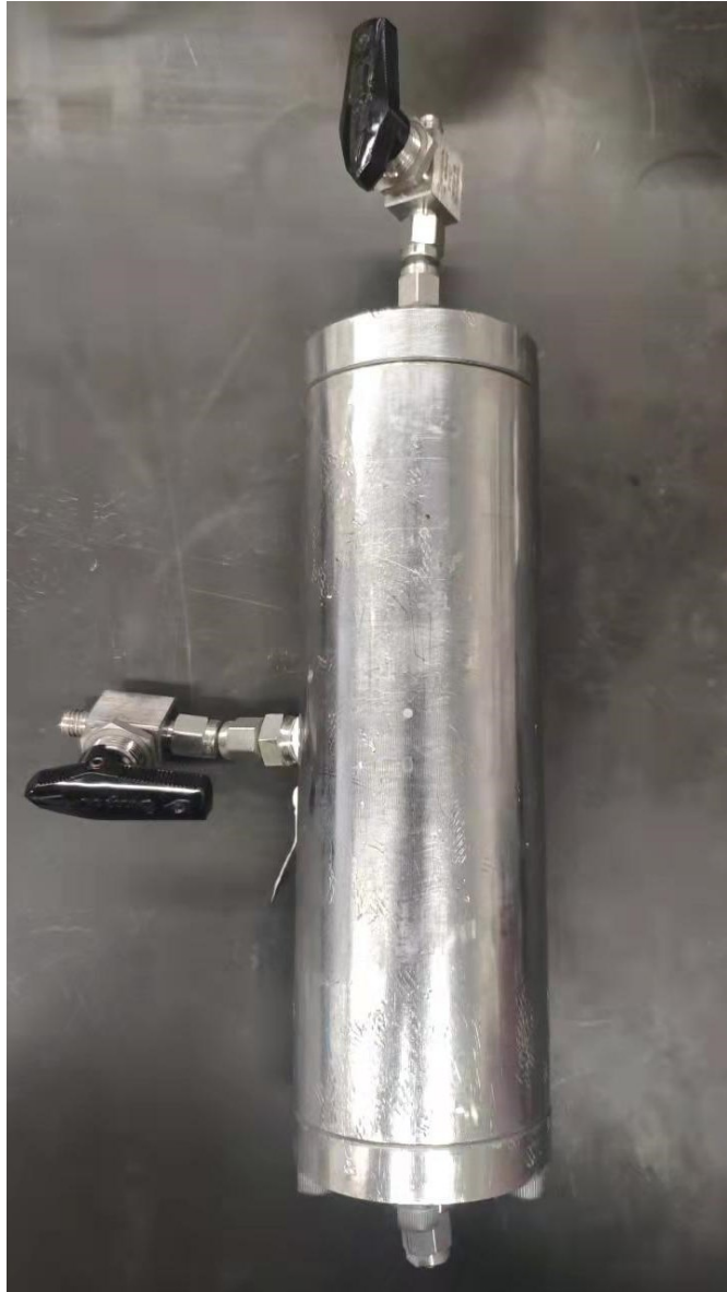
Figure A- 6 Curing cell used for the preparation of small scale samples.
