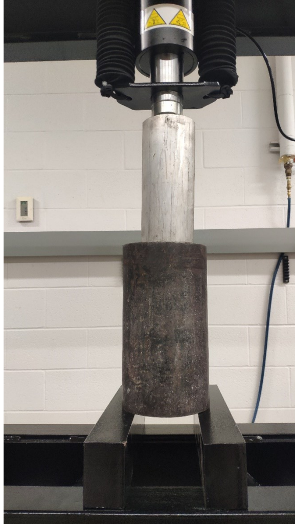
Figure E- 7 Overall setup for cement removal using the hydraulic press
