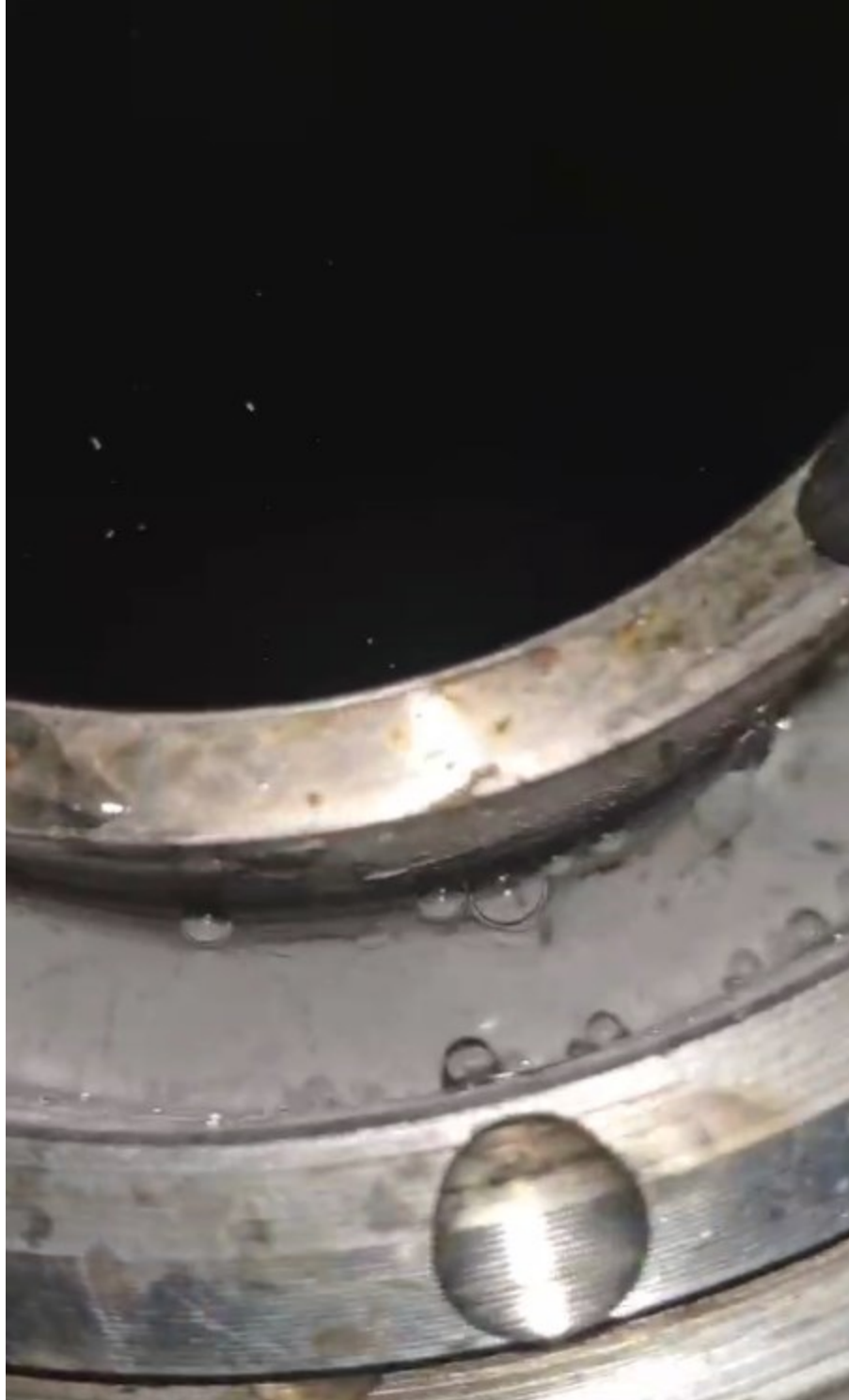
Figure 5- 10 Leakage detection result for the third cyclic pressure and constant temperature experiment
