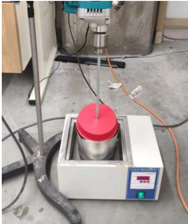
Figure E- 8 Low-speed mixing system with water bath
