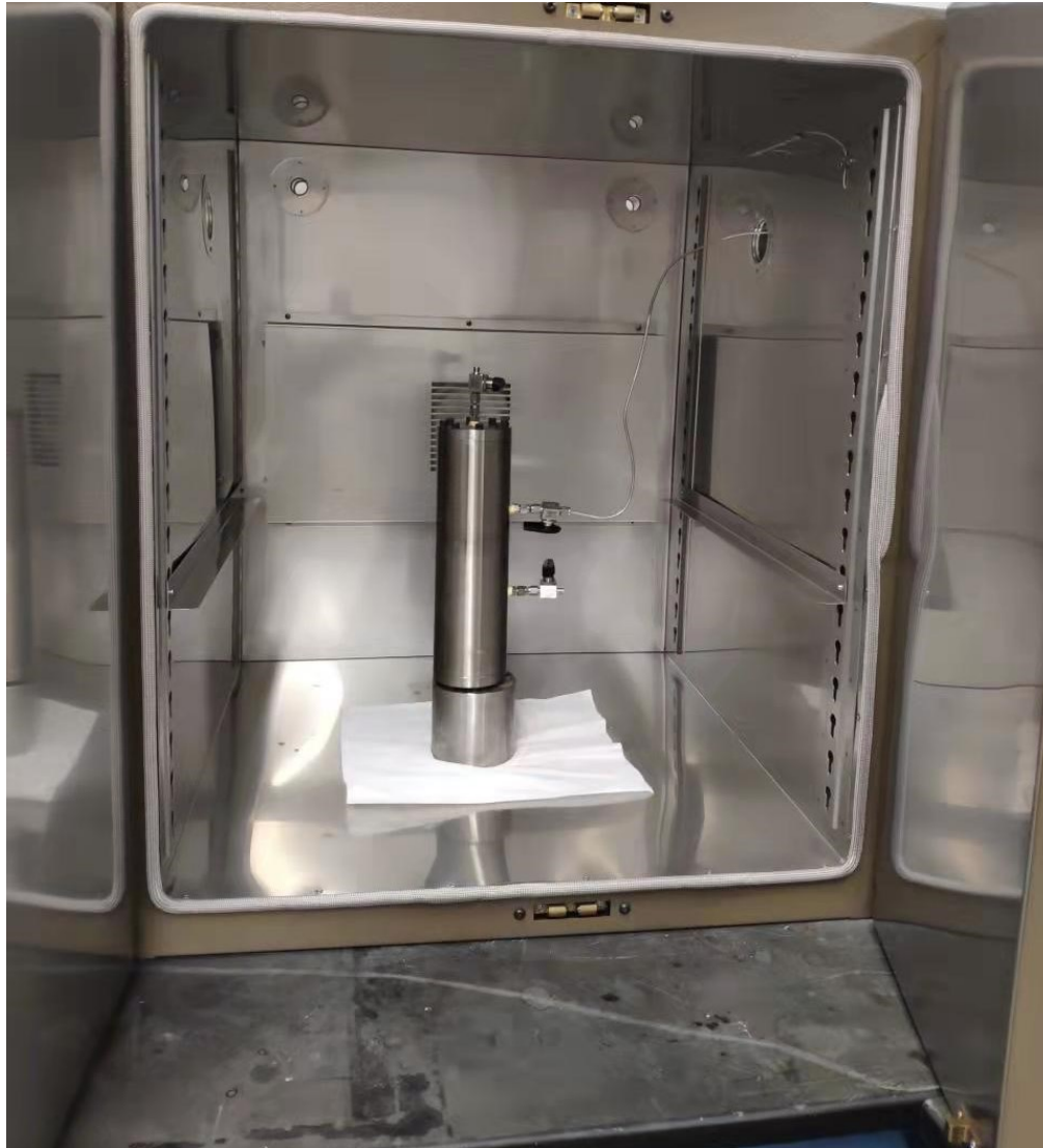
Figure A- 7 Setup before curing of small scale samples
