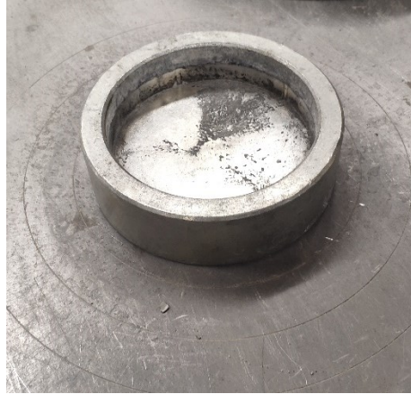
Figure E- 4 bottom holder for cement removal using loading frame
