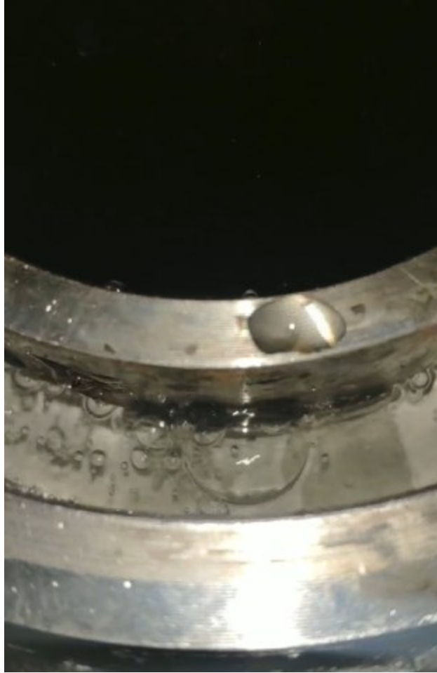
Figure 5- 8 Leakage detection result for the first cyclic pressure and constant temperature experiment
