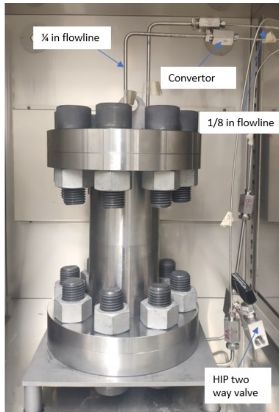
Figure E- 1 connected wellbore simulator system
