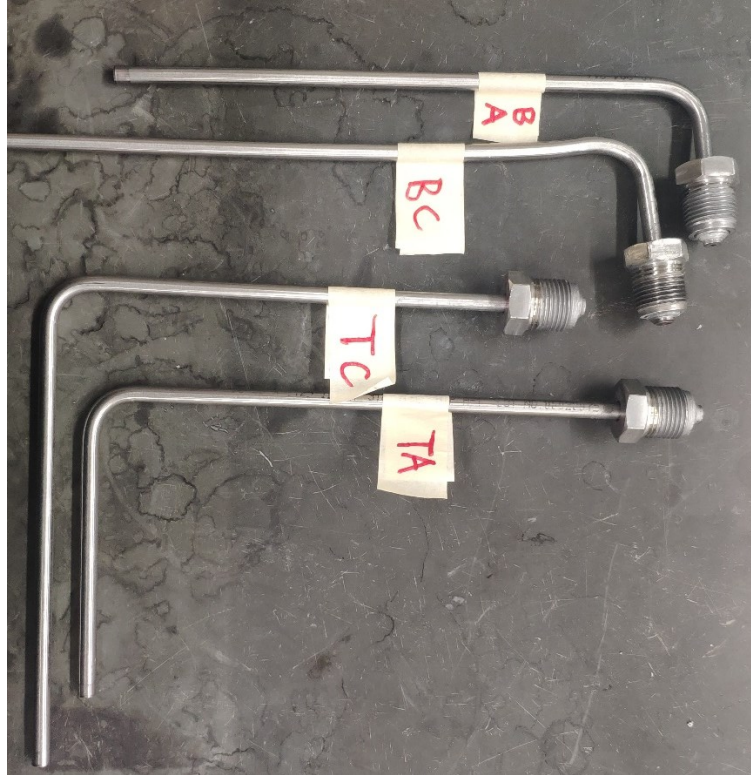
Figure C- 4 1/4 HIP connection connected with wellbore simulator main body
