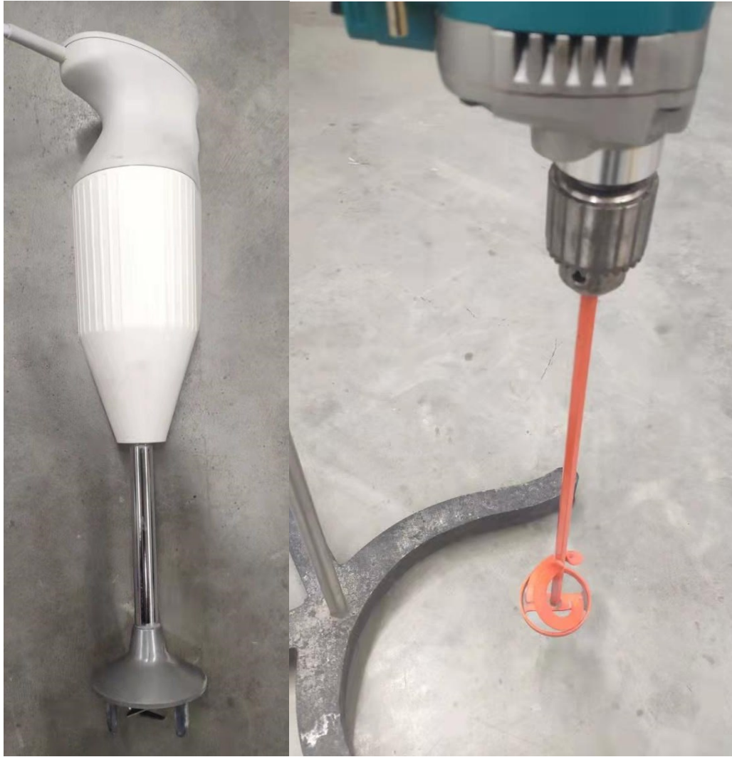
Figure 3- 3 a (left side) the high speed mixer used for small sample preparation; b (right side) the low speed mixer used for small sample preparation
