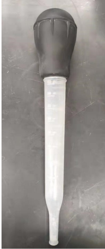
Figure A- 4 Semi transparent pipette used for injecting cement slurry to the mould for the preparation of small scale samples
