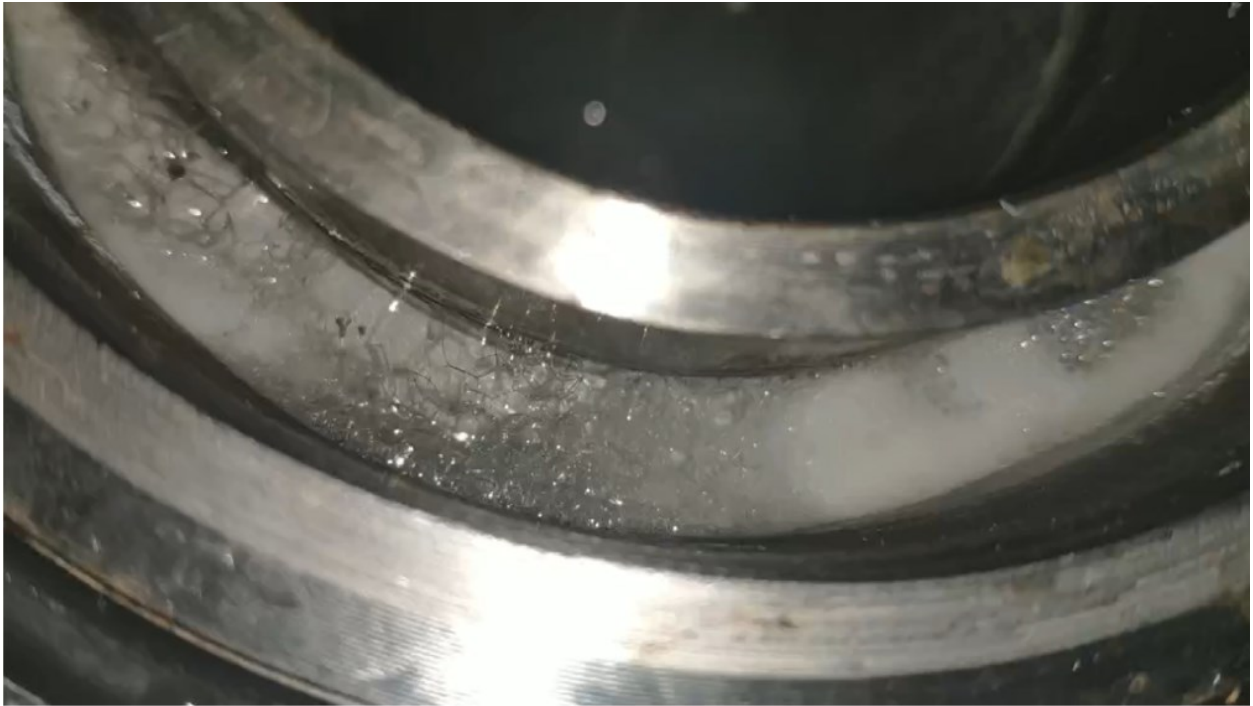
Figure 5- 5 Leakage detection result for the first constant pressure and temperature experiment
