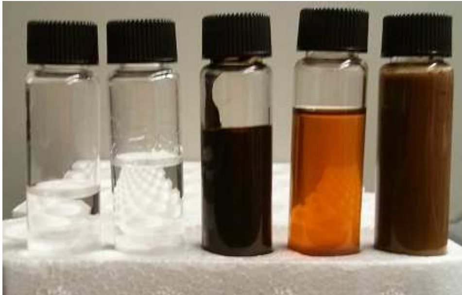
Figure 4.6: A photograph of liquids injected and collected during complete WAE flooding. From left to right: water, paraffin oil, emulsion, recovered oil, produced water.
