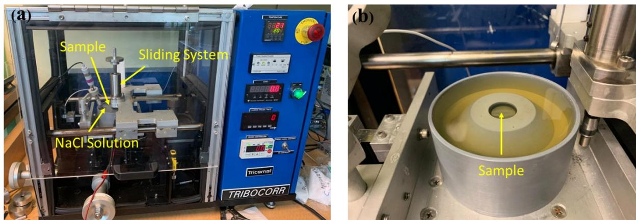
**Fig. 16.** (a) Tribocorrosion system where sliding contact immersed in NaCl aqueous solution and (b) position of the immersed sample at the end of the tribocorrosion tests.
