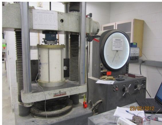
Figure 3.2: Photograph of the small compaction test equipment.
