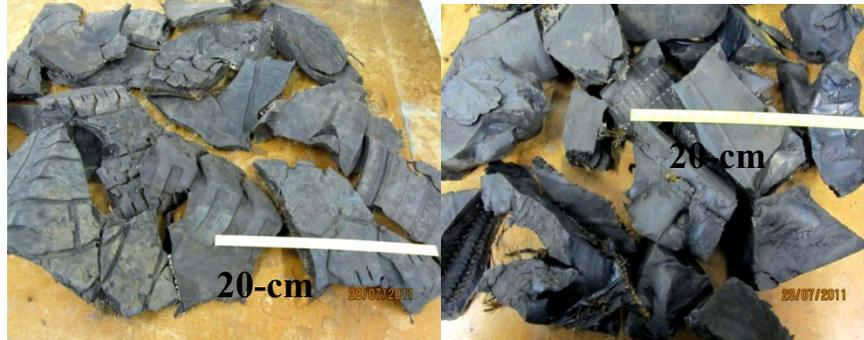
Figure 4.1: Pictures of PLTT (left) and OTR (right) used in the project.
