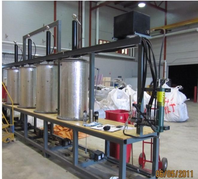
Figure 2.3: Photograph of compression apparatus at EWMCE for Testing TDA.
