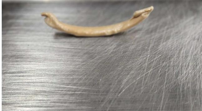
Figure 28. Part separating from the print bed due to poor bed adhesion.
