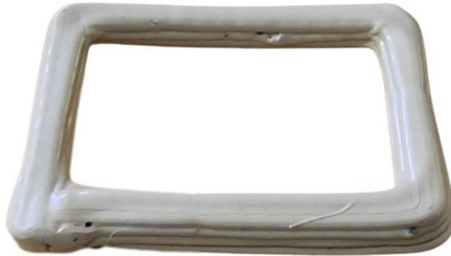
Figure 70. Rectangular geometry of 100mm x 70mm x 11mm 3D printed using PEEK.
