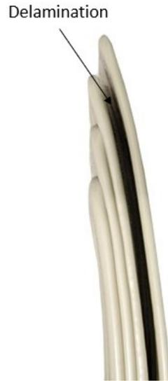
Figure 31. Delaminated layers after printing.
