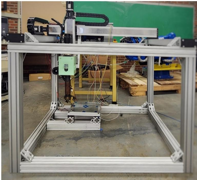
Figure 17. Three-axis cartesian gantry.
