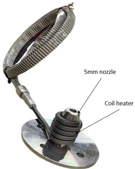
Figure 68. Coil heater assembly on 5mm nozzle
