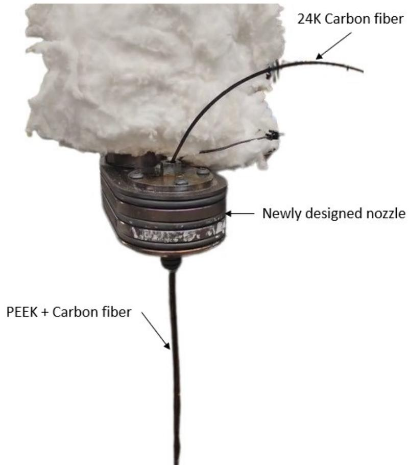
Figure 69. Extrusion trial using newly designed nozzle
