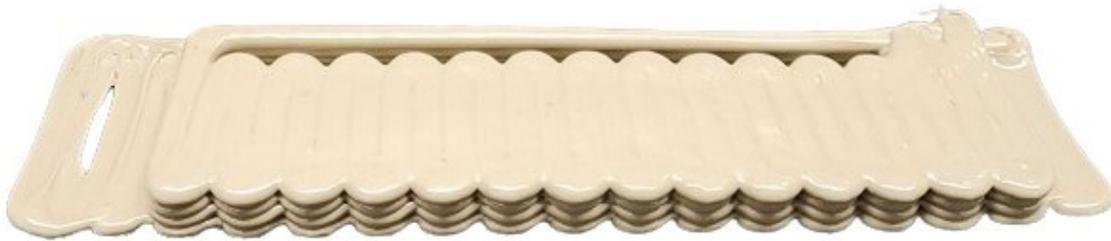
Figure 71. 3D printed PEEK block of 200mm x 70mm x 11mm.
