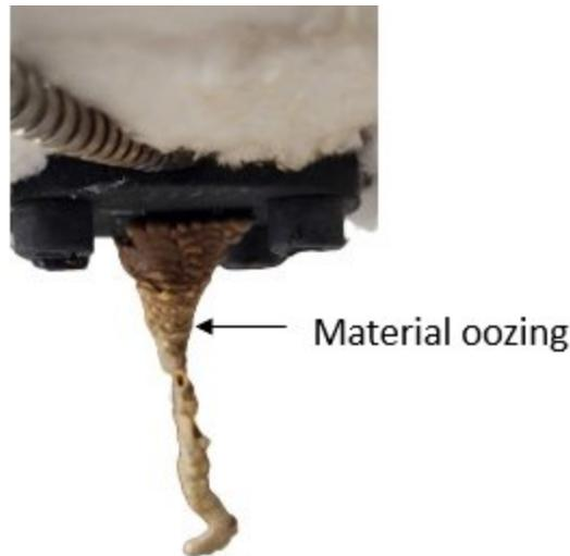
Figure 30. Material oozing from the nozzle.
