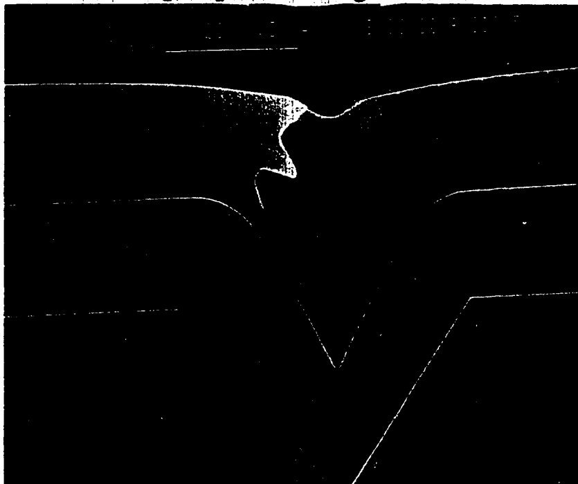
(b) Silicon V-groove with 3.8 mm silicon dioxide, 3.8 mm phosphosilicate glass after 30 minutes BOE 10:1 etch.
