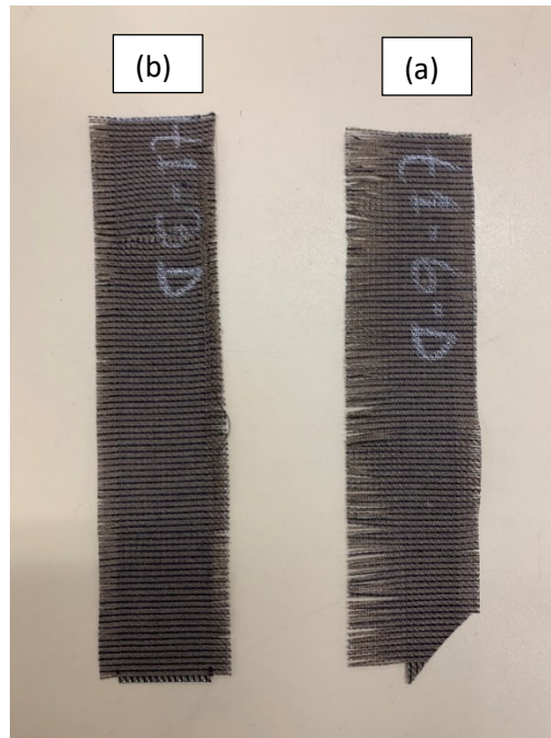
Figure 4.8 Fabric MD specimen (a) before and (b) after testing
