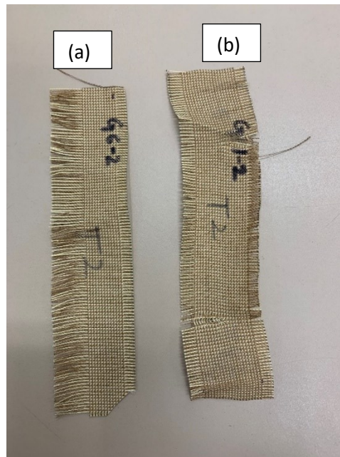
Figure 4.14 Fabric MG specimen (a) before and (b) after testing
