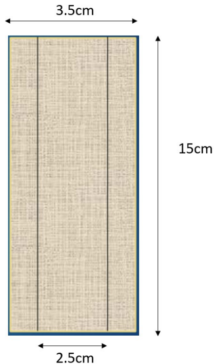
Figure 3.1 Schematic representation of the tensile strength specimen
