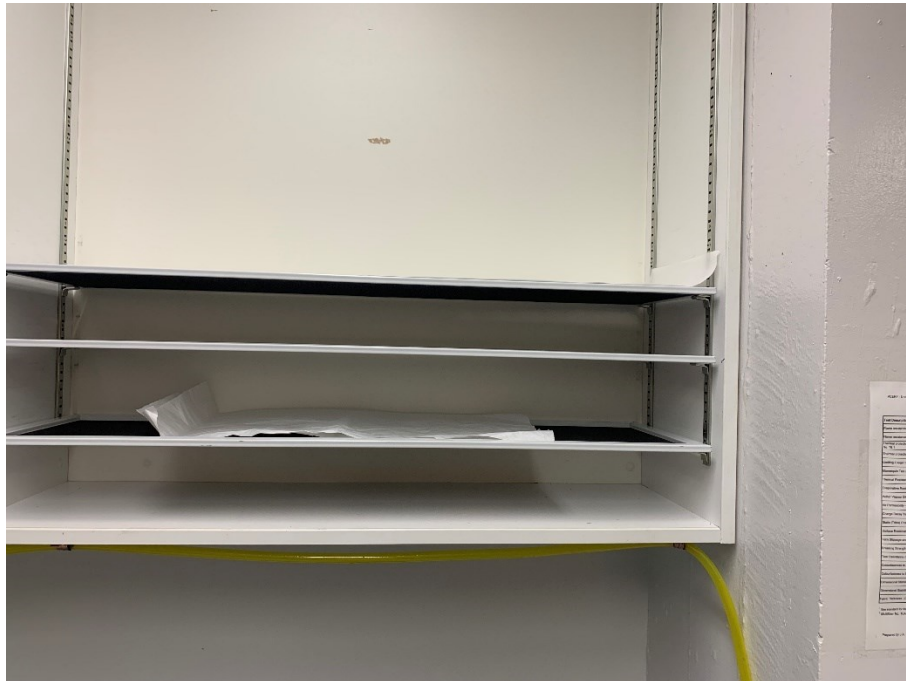
Figure 3.4 Conditioning racks for the fabric specimens
