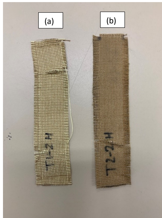
Figure 4.59 Fabric MH specimens (a) before ageing and (b) after ageing for 50 days at 90 C
