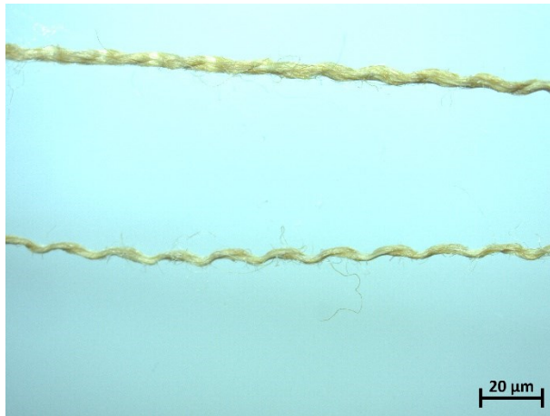
Figure 4.25 Optical microscope image of examples of yarns of Fabric ME having a different strength
