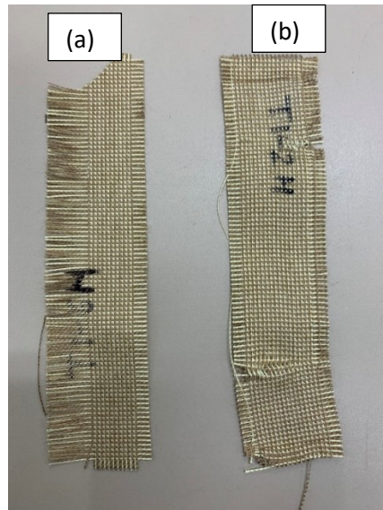
Figure 4.16 Fabric MH specimen before and after testing
