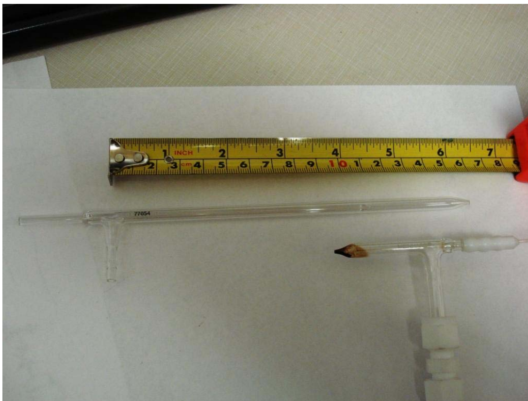
Figure 5. 2 TR-50-A0.5 (short barrel) vs. DIHEN-170-A0.3 (long barrel) supplied by Meinhard Glass Products
