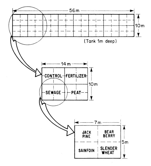
Figure 1. Plan of spoil tank.
