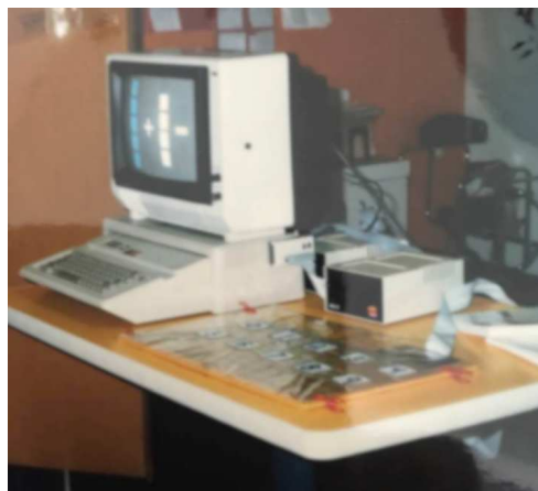
Figure 2. Example of Unicorn Keyboard connected to Apple computer through Adaptive Firmware Card
