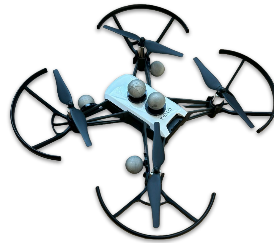
Fig. 3: Tello drone with reflective Vicon markers attached
