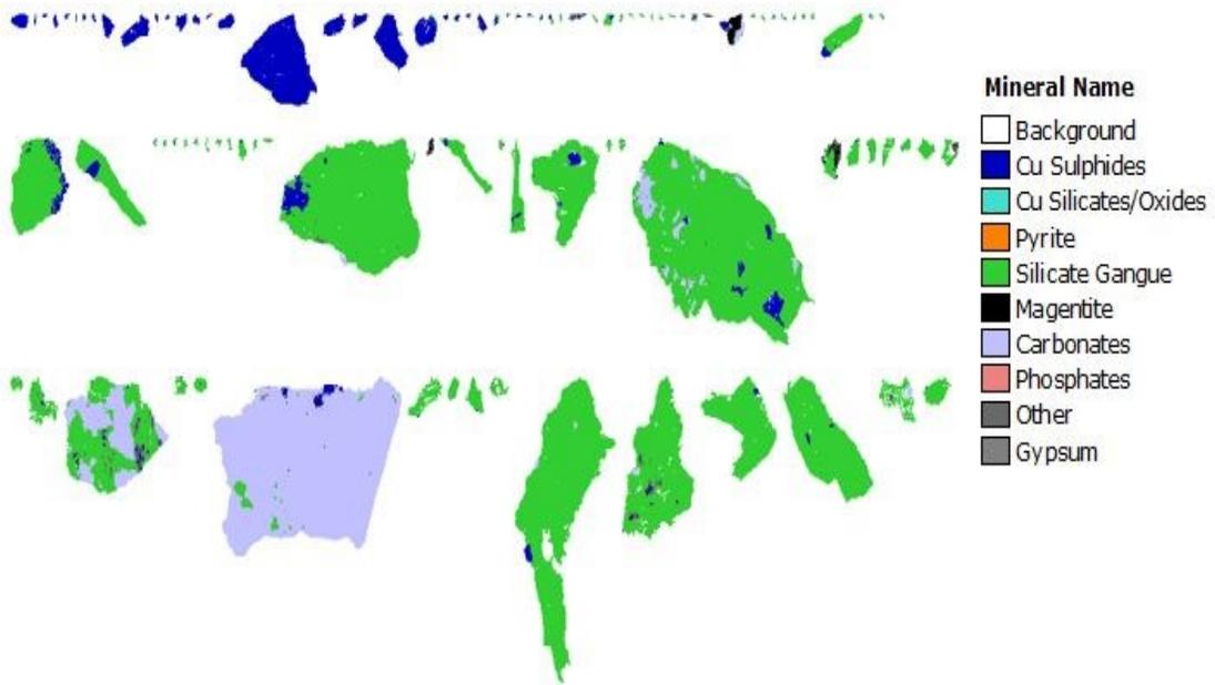
Figure 4-12 Graph illustrating the distribution of mineral phases and their liberation for microwave treated material.
