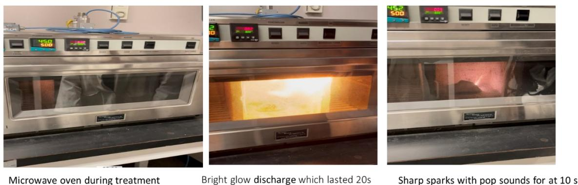
*Figure 4-6 Pictures showing the arcing and discharges experienced during bench scale microwave treatment.*
