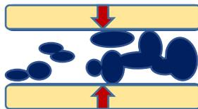
*Figure 2-3 Illustration of compression of particles between two surfaces.*
