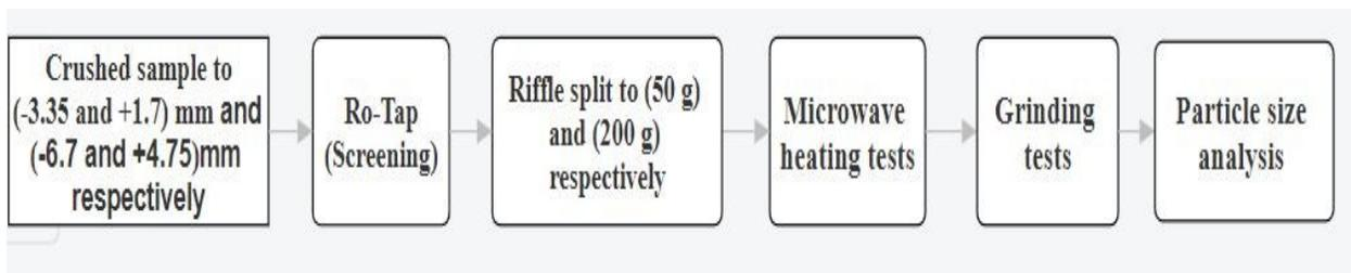
*Figure 3-3 Flowsheet for microwave bench-scale work*
