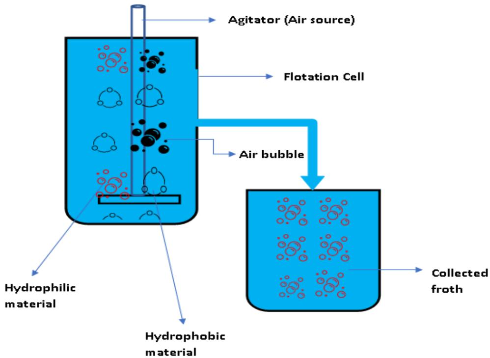
Figure 3-10 Schematic diagram of the froth flotation batch process
