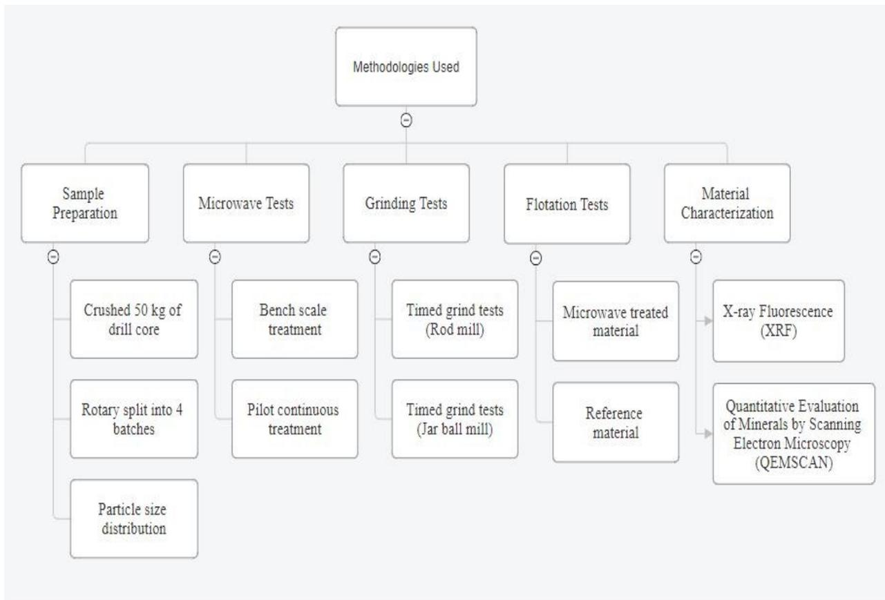
Figure 3-1 shows a flowchart illustrating the methodologies employed and the workflow.
