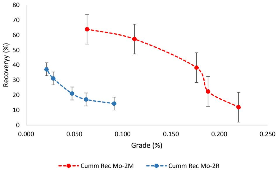
Figure 4-19 Recovery vs grade graph for (Mo) comparison between HVC-2R and HVC-2M (250  $\mu$ m)
