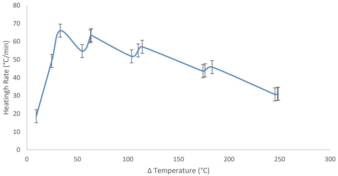
Figure 4-2 Microwave heating rate vs change in temperature for (-3.35 and +1.7) mm 50 g charge
