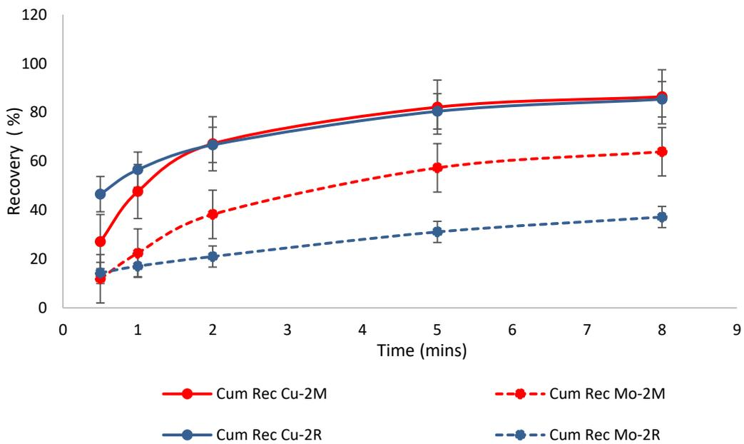
Figure 4-15 Recovery vs time curves comparison between HVC-2R and HVC-2M (250  $\mu\text{m}$ )
