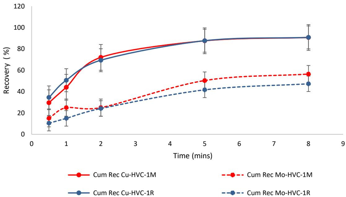
Figure 4-14 Recovery vs time curves comparison between HVC-1R and HVC-1M (200  $\mu\text{m}$ )
