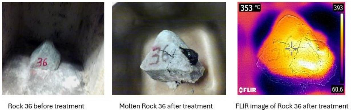
Figure 4-8 Showing the transformation of rock 36 before and after bench-scale microwave treatment.
