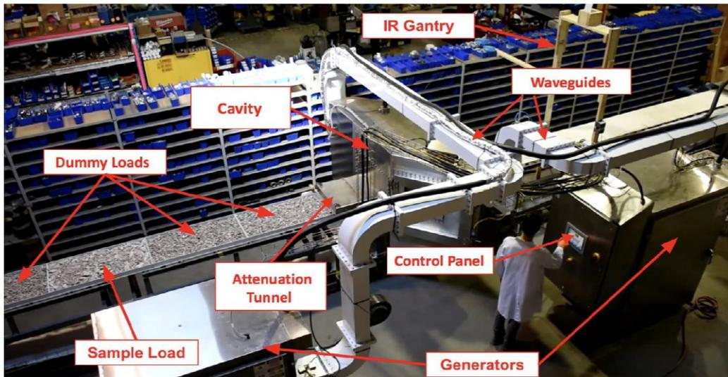
Figure 3-5 Overview of pilot-scale microwave system (Forster 2023)
