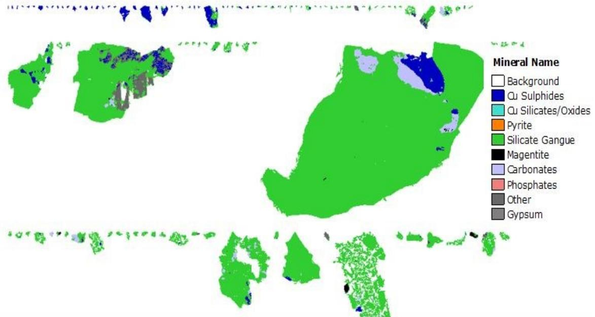
Figure 4-13 Graph illustrating the distribution of mineral phases and their liberation for untreated material.
