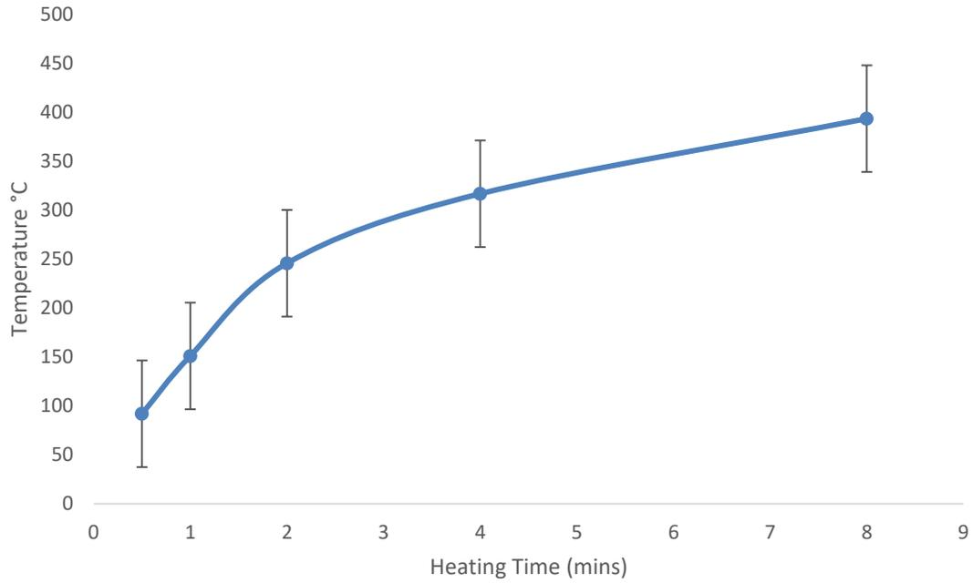
Figure 4-4 Microwave Heating Behaviour Curve for (-6.7 and +4.75) mm 200 g charge
