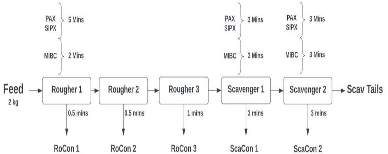
Figure 3-9 Flow chart of the froth flotation batch process.
