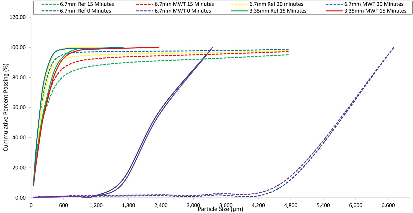
Figure 4-11 A graph showing the comparison between reference & bench microwave treated samples for both finer and coarser size fractions.
