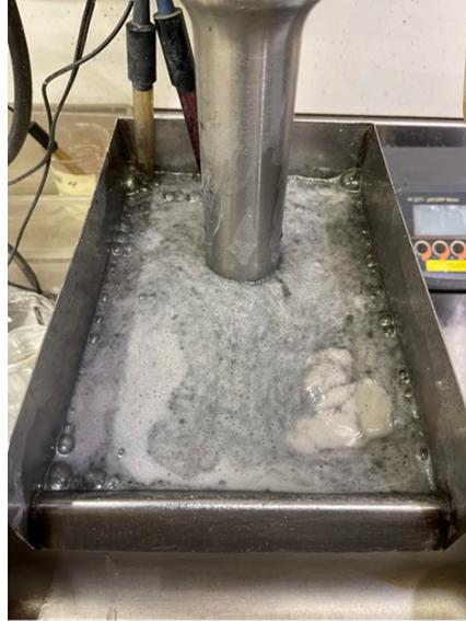
Batch Flotation Cell Setup
