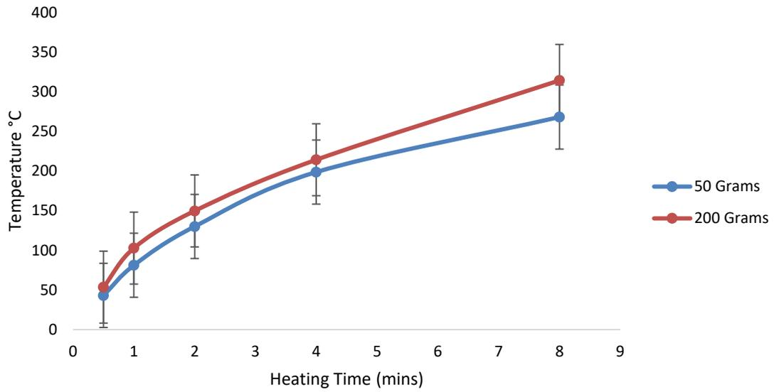
Figure 4-1 Comparison of Microwave heating behaviour curve for (-3.35 and +1.7) mm 50 g and 200 g charge
