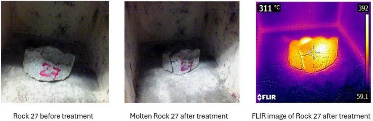
Figure 4-7 Showing the transformation of rock 27 before and after bench-scale microwave treatment.
