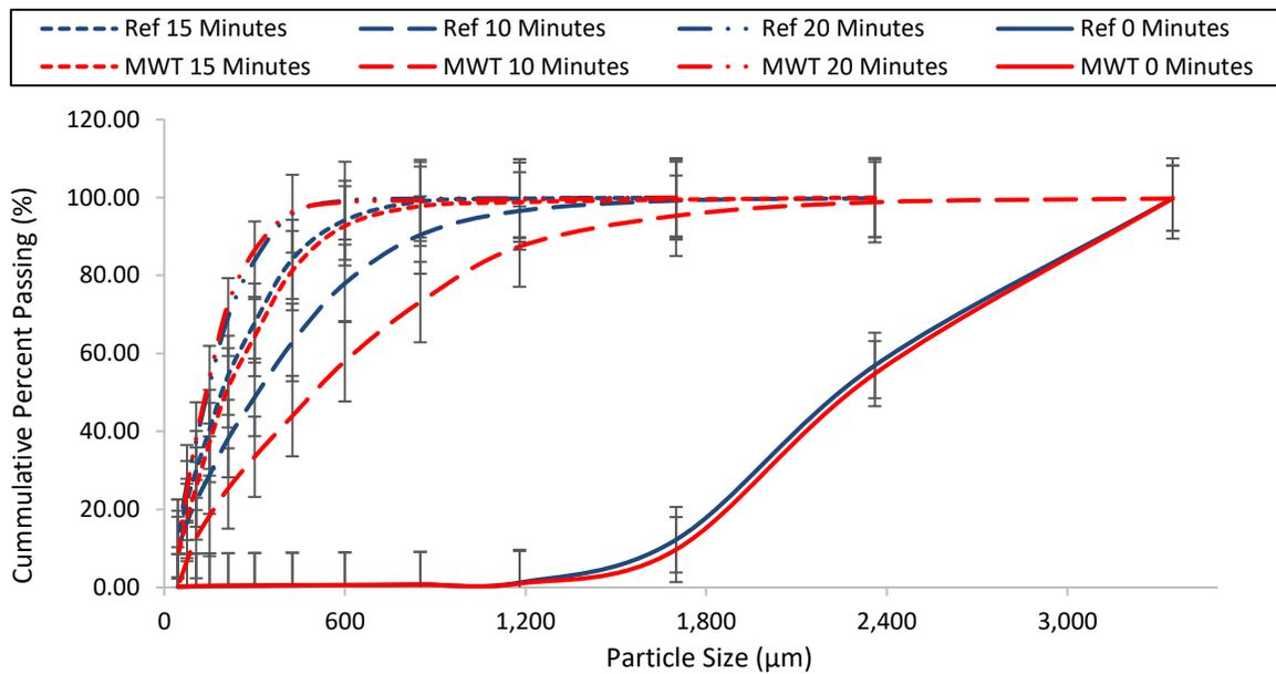
Figure 4-9 A graph showing the PSD comparisons between the MWT and reference material for the (-3.35 and +1.7) mm using a ball jar mill.
