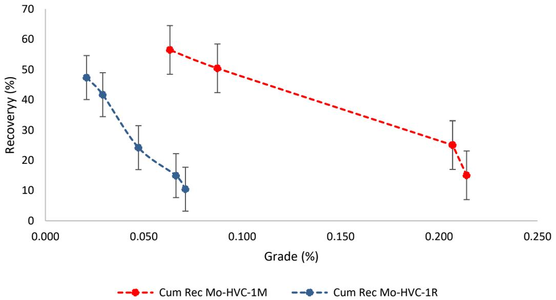
Figure 4-17 Recovery vs grade graph for Mo comparison between HVC-1R and HVC-1M (200  $\mu$ m)
