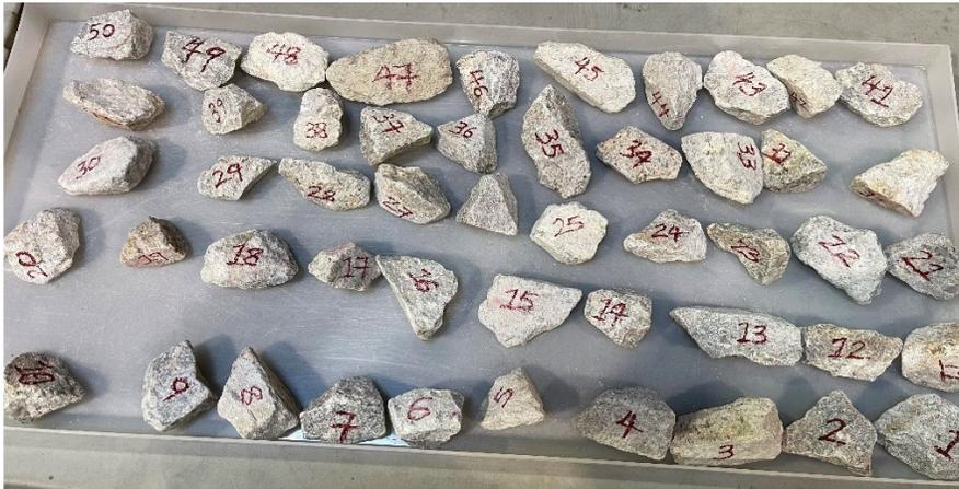
*Figure 3-4 A tray of individually numbered rocks before microwave treatment.*
