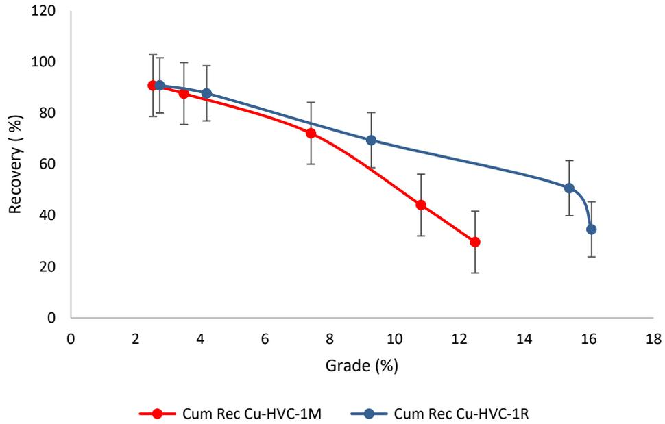
Figure 4-16 Recovery vs grade graph for Cu comparison between HVC-1R and HVC-1M (200  $\mu$ m)
