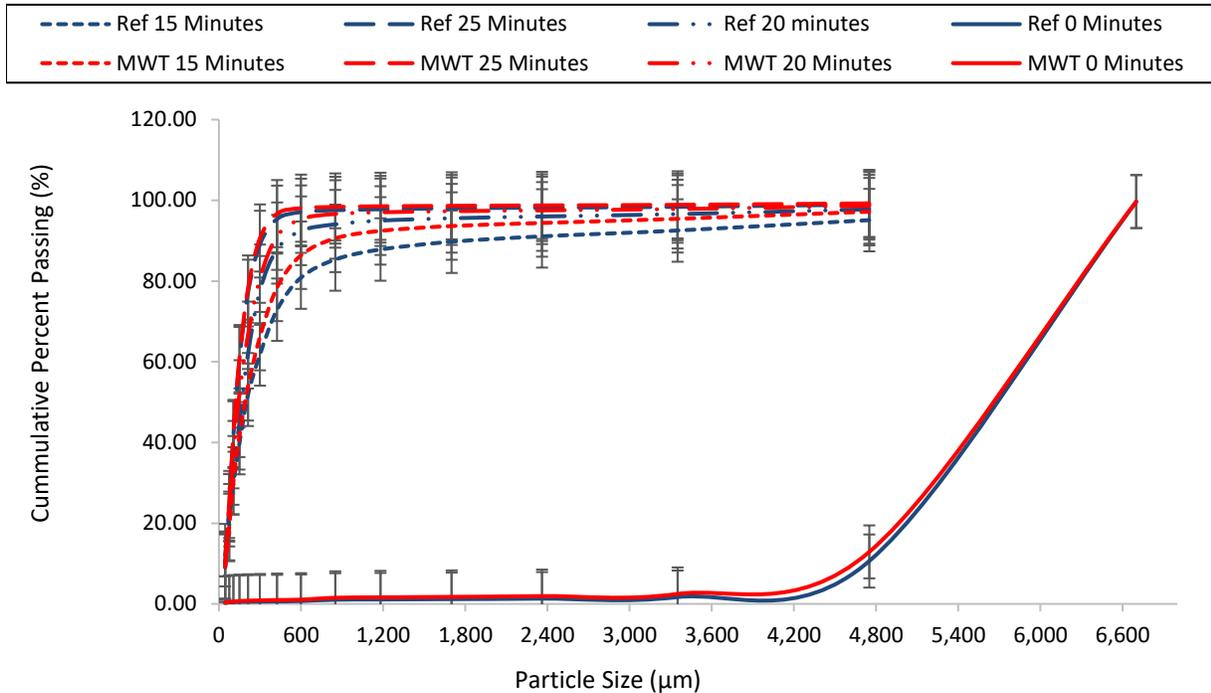
Figure 4-10 A graph showing the PSD comparisons between the MWT and Reference material for the coarser size fraction (-6.7 and +4.75) mm using a ball jar mill.
