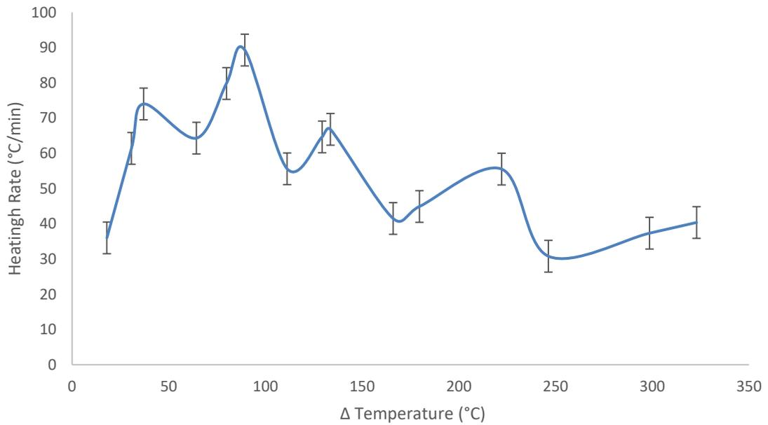
Figure 4-5 Microwave Heating Rate vs Temperature for (-6.7 and +4.75) mm 200 g charge
