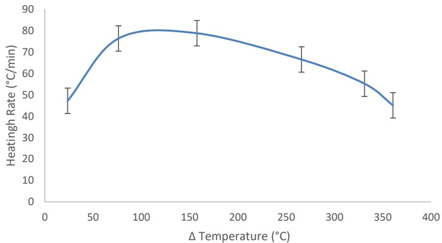
Figure 4-3 Microwave heating rate vs change in temperature for (-3.35 and +1.7) mm 200 g charge
