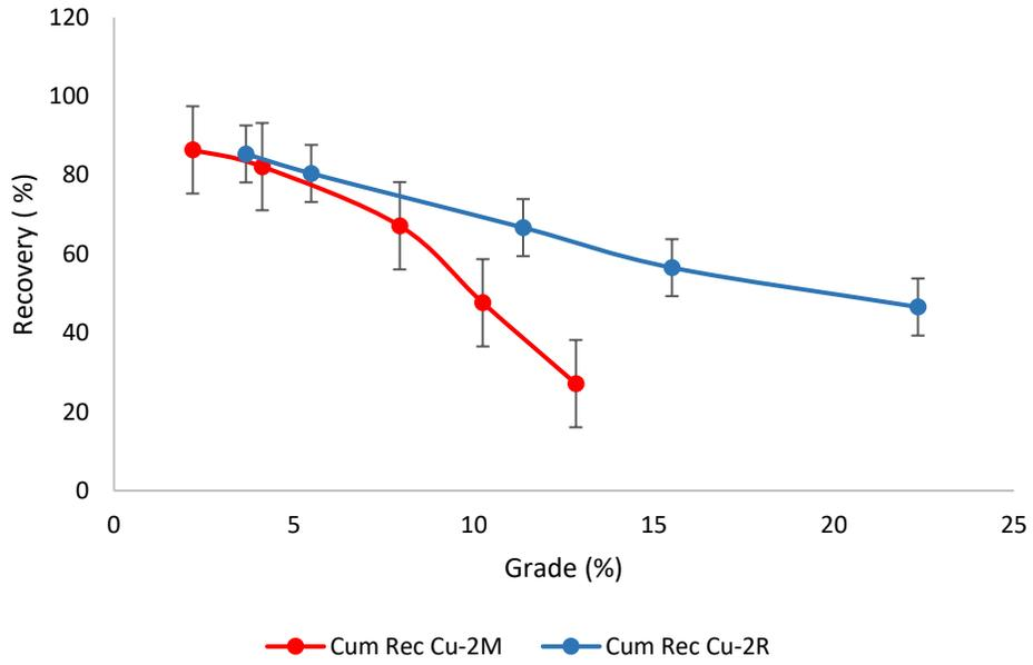
Figure 4-18 Recovery vs grade graph for Cu comparison between HVC-2R and HVC-2M (250  $\mu$ m)
