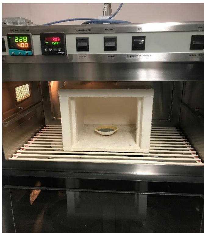
*Figure 3-2 Bench scale microwave oven
