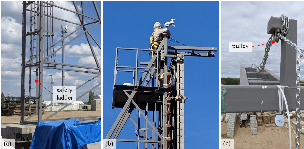
Figure 4.12: Some fixtures included in the test device (a) Safety ladder installed to reach the work platform (b) Work platform close-up (c) Pulley to lift the lever arm.
