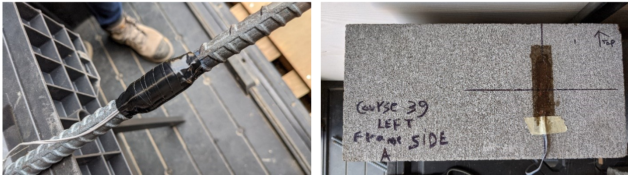
Figure 4.25: Strain gauges installation (a) On rebar and completely coated (b) Installed with adhesive on concrete block.
