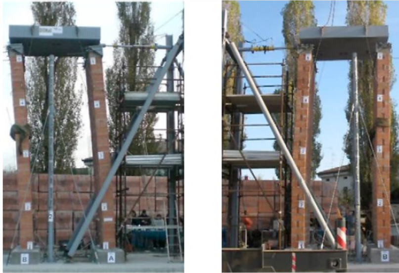
Figure 2.7: Test setup for cyclic out-of-plane testing on RM walls (da Porto, 2011).
