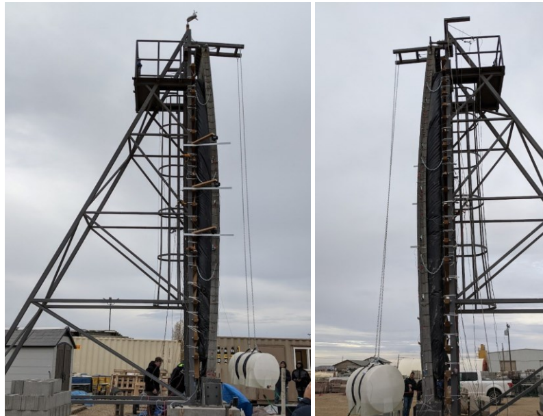
Figure 4.27: Test wall at peak load of cycle 6, taken from left and right sides of the setup.
