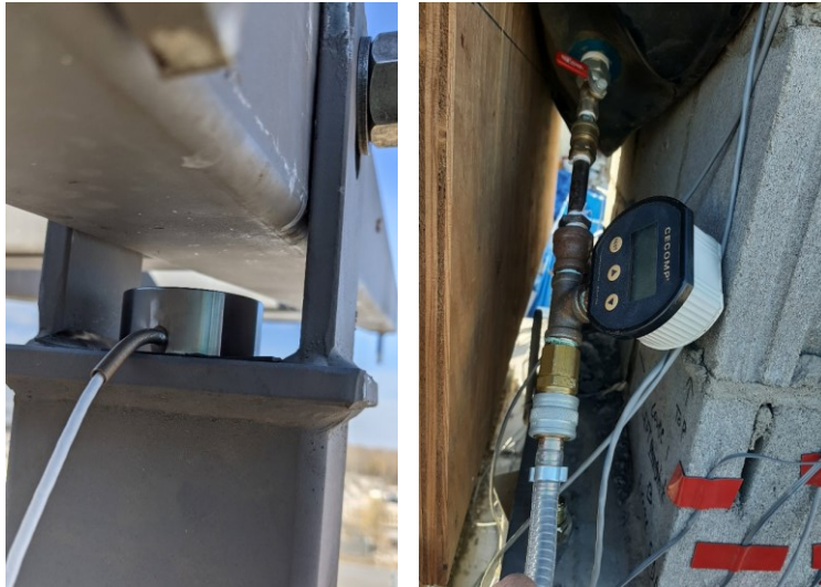
Figure 4.23: Instruments used to read loads applied (a) Load cells (b) Pressure gauge.
