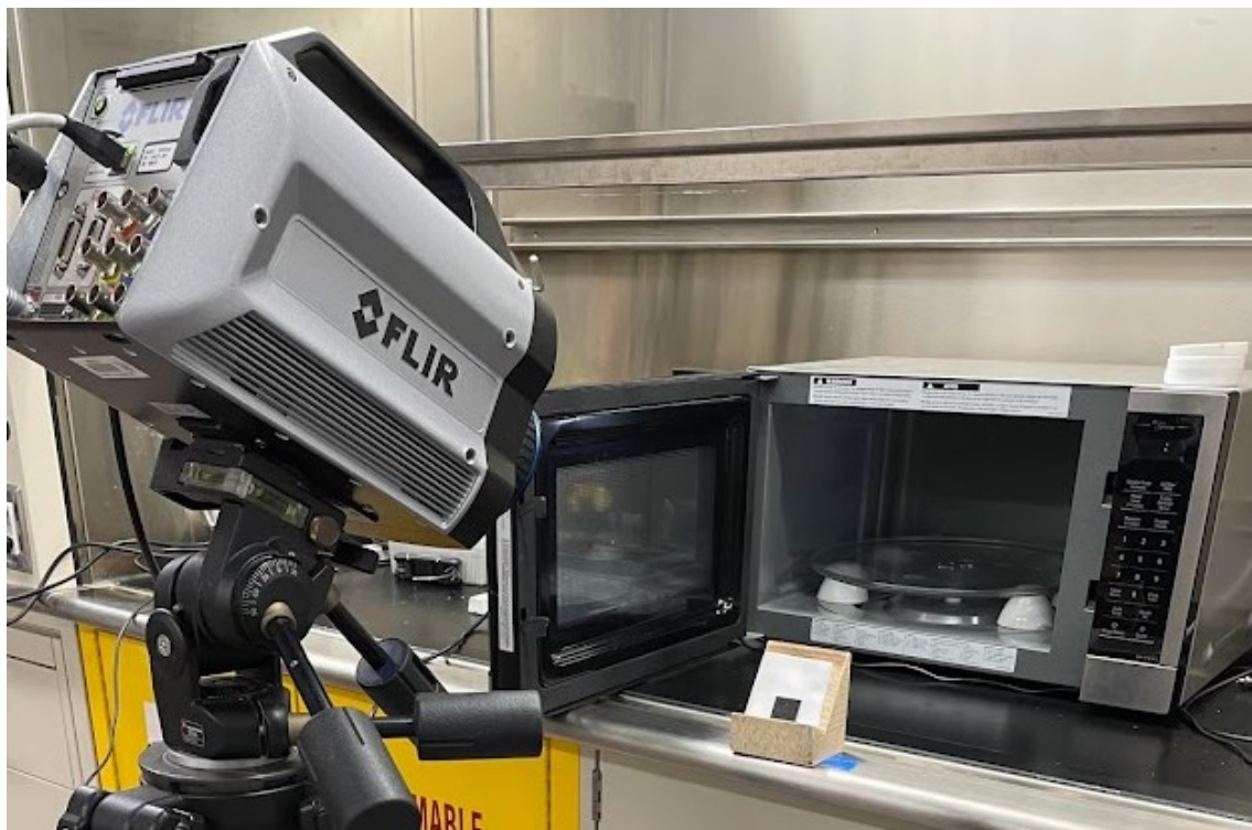
Figure 17: Microwave heating of nanocomposites examined using thermal imaging
