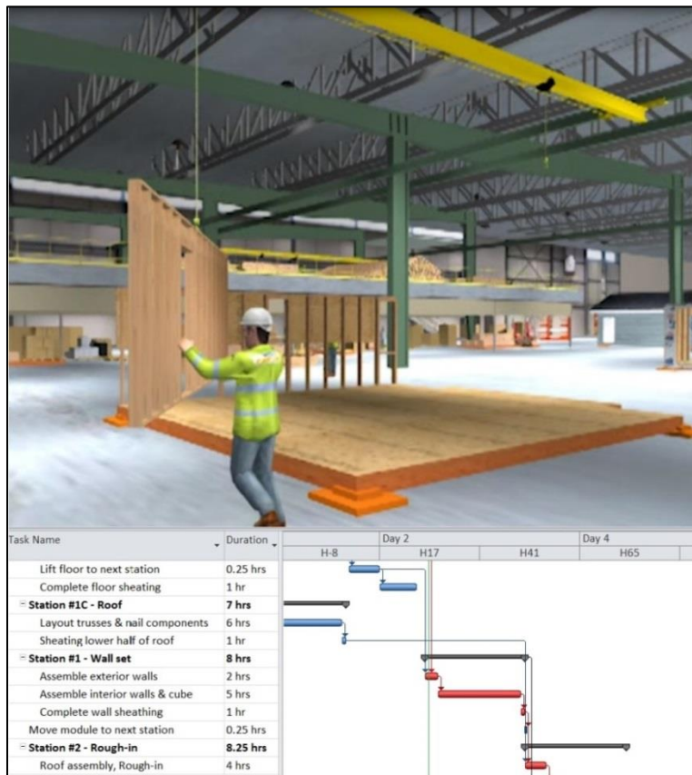
Figure 26: A snapshot of the PSV model developed in 3ds Max
