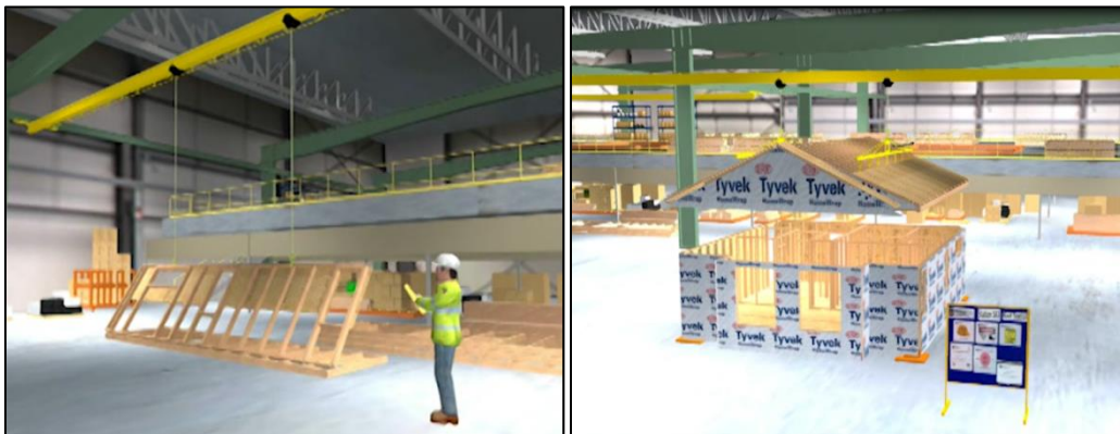
(a) Examination of overhead crane for proper lifting
