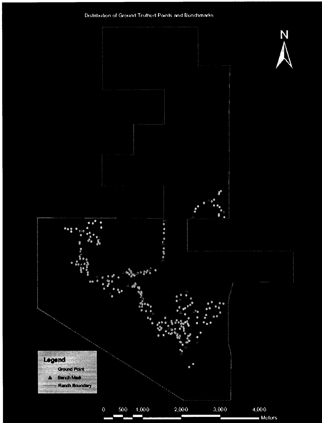
Figure 3-2 The distribution of 27 inter-connected benchmarks and 260 ground truthed data points around those benchmarks.
