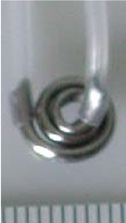
Figure 3.1: Cooling coil (mm scale bar below) with attached tubing through which cold water is flushed. The coil is placed underneath the Temporalis muscle with the flattest face adjacent to the skull. In this case the coil was constructed out of a 20 G needle.
