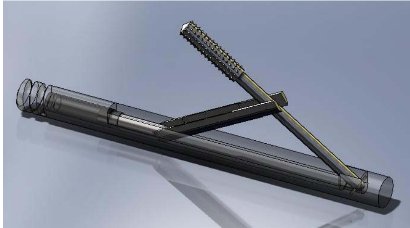
Figure 3-9 CAD model of the cutting tool in its operating position
