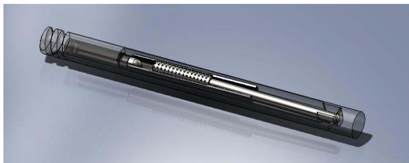
Figure 3-8 CAD model of the cutting tool in its closed position
