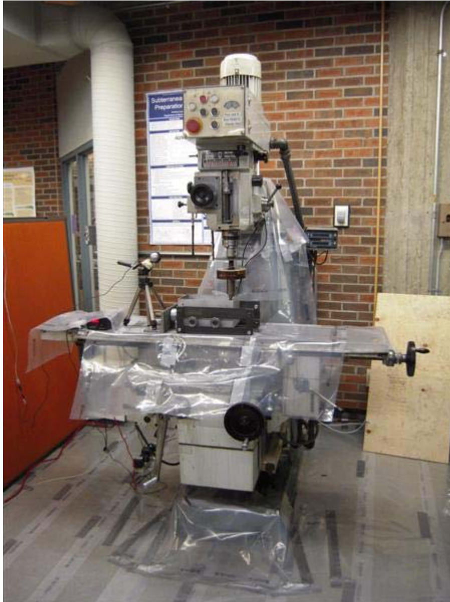
Figure 4-2 Photograph of the instrumented mill
