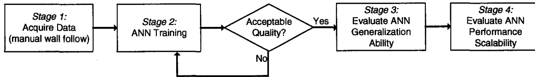
Figure 3.1 – Methodology for behavior synthesis Methodology for behavior synthesis.
