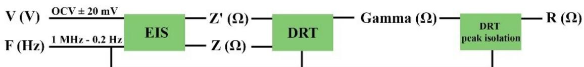
Figure 1-7 The relationship between different variables in measured electrochemical parameters.
