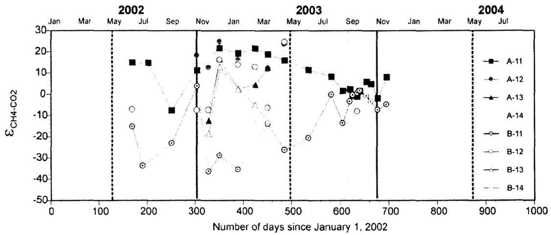
**Figure 3-31** Apparent kinetic isotope effect  $\epsilon_{\text{CH}_4\text{-CO}_2}$  for soil gas samples collected near well A4.
