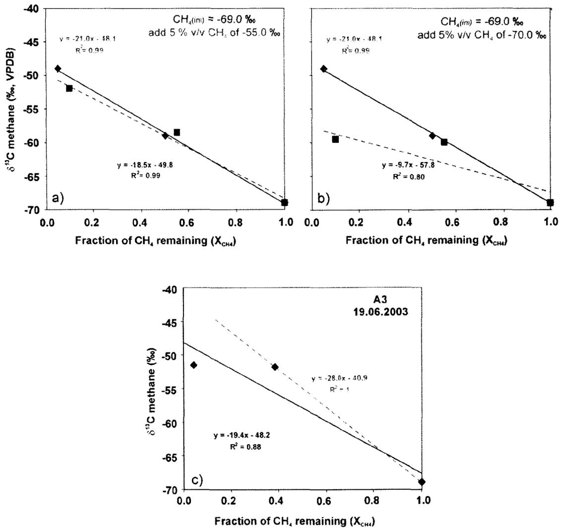
**Figure 3-38** Carbon stable isotope composition of methane vs. the fraction of methane remaining. The addition of 5 % v/v methane having  $\delta^{13}\text{C}$  of  $-55 \text{ ‰}$  (a) and  $-70 \text{ ‰}$  (b) shifts the “original” values (rhombs) to new positions (squares). Figure 3-38(b) mimics well the distribution of measured  $\delta^{13}\text{C}$  compositions and estimated fractions of methane oxidized at wells A3 (c) in the summer.
