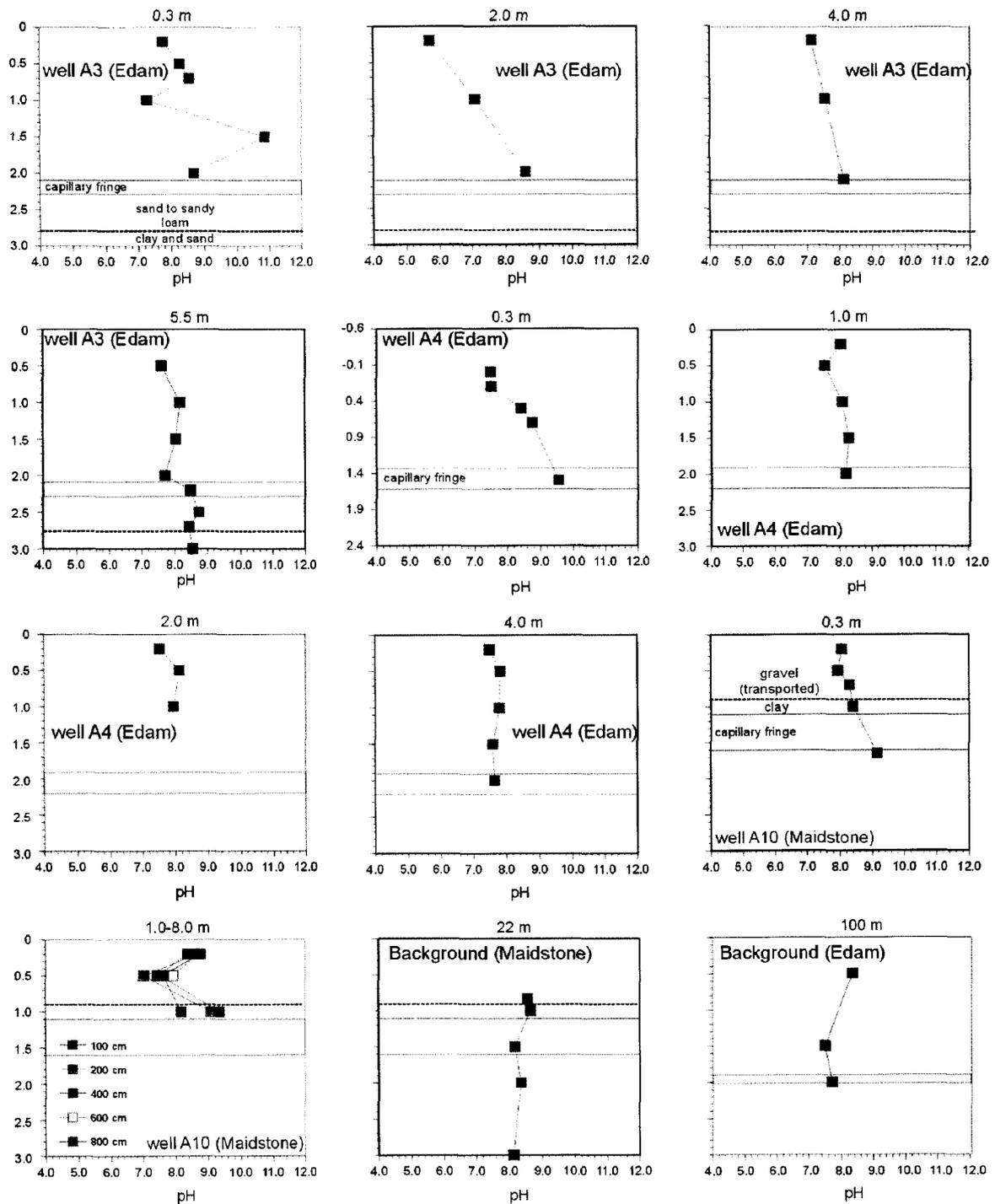
**Figure 6-4** Soil pH of samples collected at different distances and depths from the well bores at the three research sites (i.e. A3, A4, and A10). Also included are the background locations. One at 22 m west from well A10 (Maidstone), and the other at 100 m west from well A3 (Edam).
