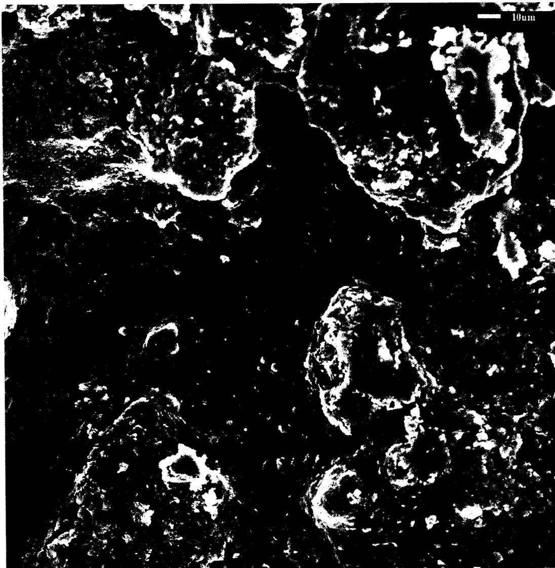
**Figure 4-16** Area of "flat" type II calcite growth in a sample collected at 0.5 mbs, well A3.
