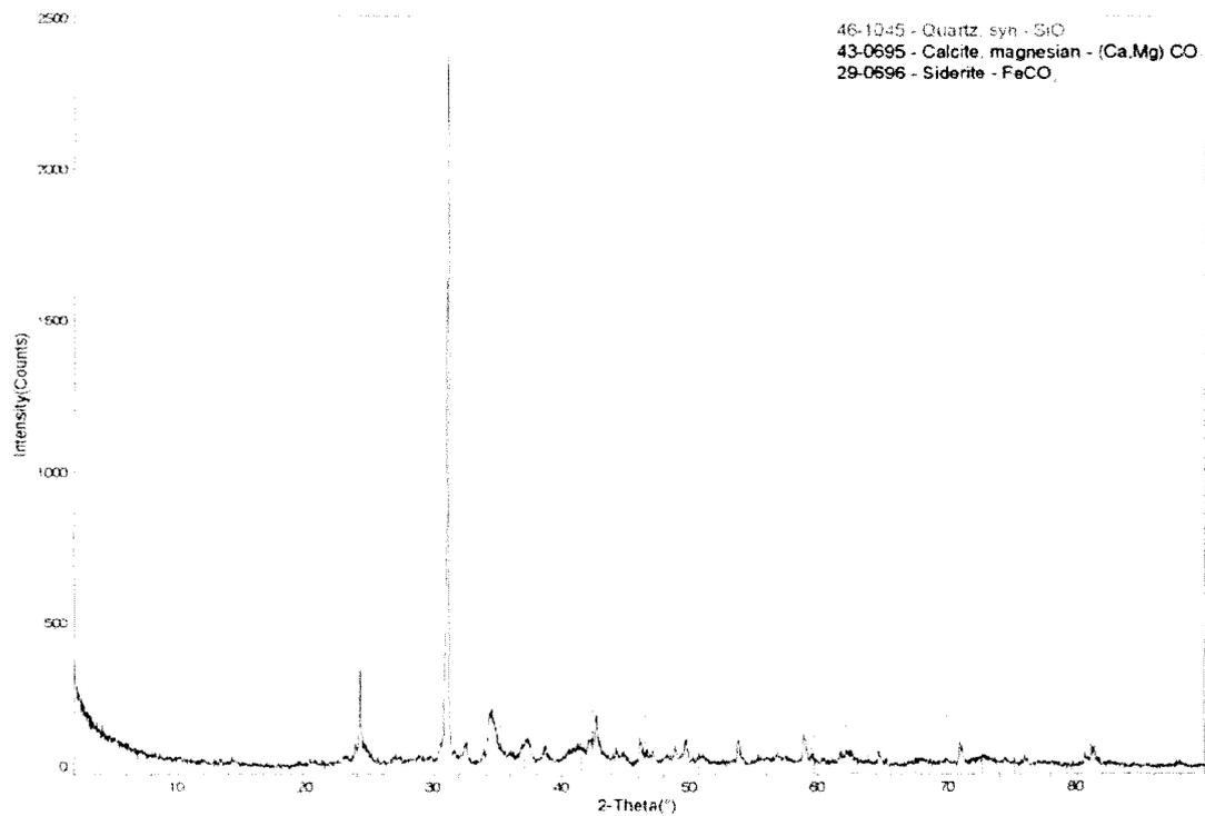
**Figure 4-4** XRD spectra of a sample of carbonate/rust scaling collected at 2.47 mbs from the casing of well A9-17, Aberfeldy oil field. Other mineral phases identified in this sample include Magnesioferrite, Goethite and Anorthite.
