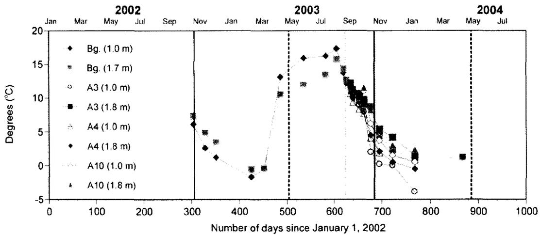
**Figure 3-26** Temperature measurements ( $^{\circ}\text{C}$ ) at different depths in the soil at the background site and the two research sites near wells A3 and A4 at Edam and the site at Maidstone.
