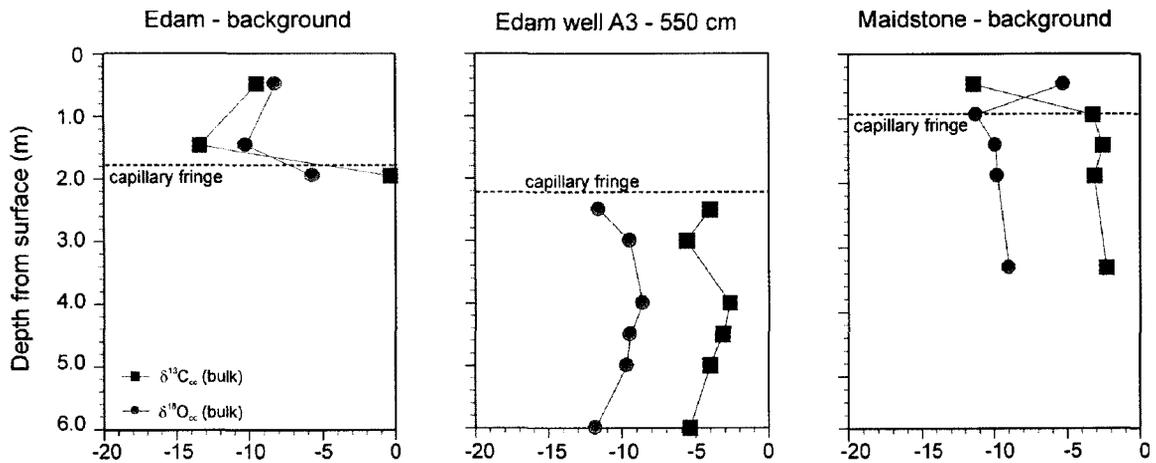
**Figure 5-2** Carbon and oxygen stable isotope compositions of bulk soil carbonate samples from the saturated and unsaturated soil at the background sites at Edam and Maidstone.
