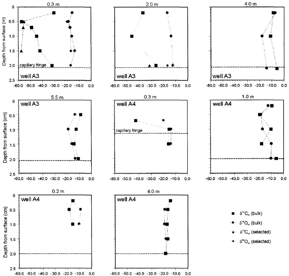
**Figure 6-1** Carbon and oxygen stable isotope compositions (‰, VPDB) of bulk and selected soil carbonate samples collected in microaerophilic and oxygen-rich soil near wells A3 and A4, Edam. The lateral distance (m) of every soil profile from the respective well bore is denoted on the top of each graph.
