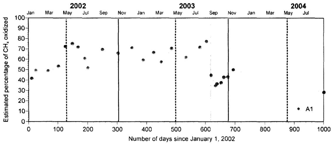
**Figure 3-28** Estimated percentage of methane oxidized in shallow (1.0 m) microaerophilic soil at well A3.
