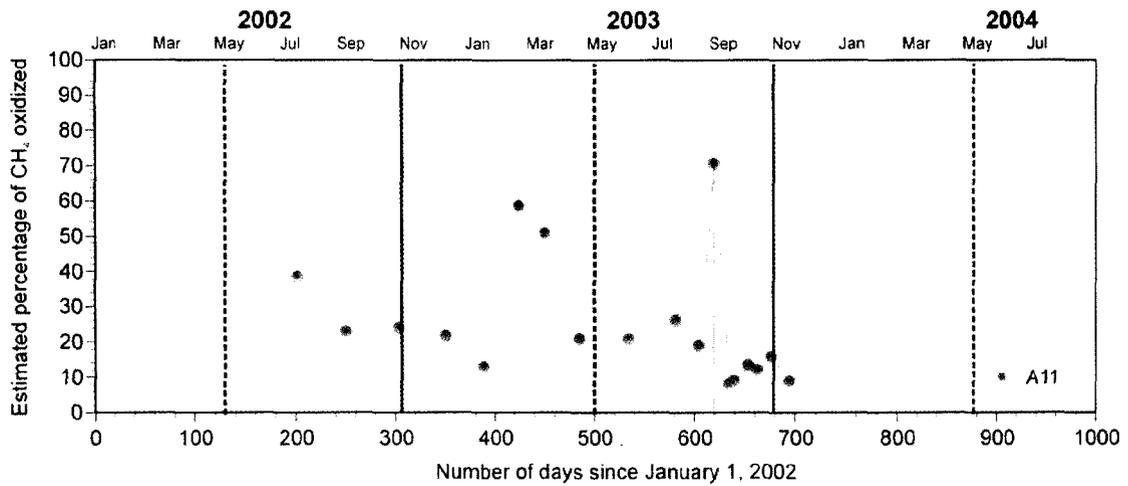
**Figure 3-29** Percentage of methane oxidized in shallow (1.0 m) microaerophilic soil at well A4.
