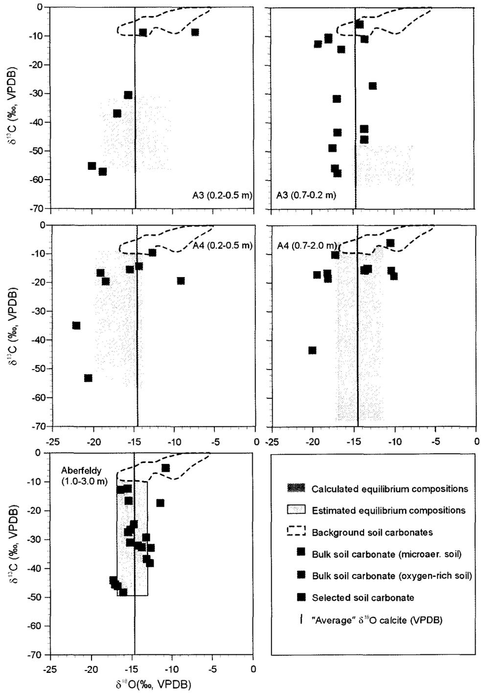
**Figure 6-6** A comparison between calculated/estimated compositions of calcite that would precipitate in equilibrium with soil CO<sub>2</sub> and soil moisture at Edam and Aberfeldy and measured  $\delta^{13}\text{C}$  and  $\delta^{18}\text{O}$  compositions (‰, VPDB) of soil carbonate samples collected at these sites.
