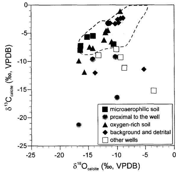
**Figure 6-7** Oxygen and carbon stable isotope compositions of soil carbonates from the microaerophilic and oxygen-rich soils and also from detrital and background soil carbonates at well A10 at Maidstone. The compositions of samples from the rest of the wells at Maidstone are also plotted on the diagram.
