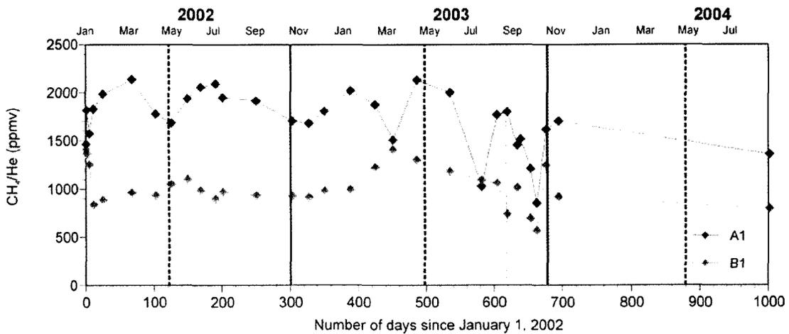
**Figure 3-27** Ratio of the concentrations of methane to helium in gas samples collected from the proximal probe and probe A1 at well A3. The difference between the ratios measured at the two sampling points, separated by 0.85 m of sandy soil, reaches factor of two.
