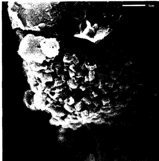
**Figure 4-5** Framboid pyrite in close association with authigenic calcite (type II). The sample was collected at 0.5 mbs and 0.3 m away from the well bore of well A3, and provides evidence for the existence of anaerobic conditions in parts of the soil.
