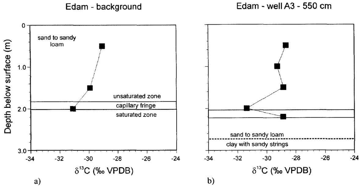
**Figure 5-4** (a) Carbon stable isotopic composition of soil organic matter from the background site at Edam, and (b) in a profile 5.5 m away from well A3, Edam.
