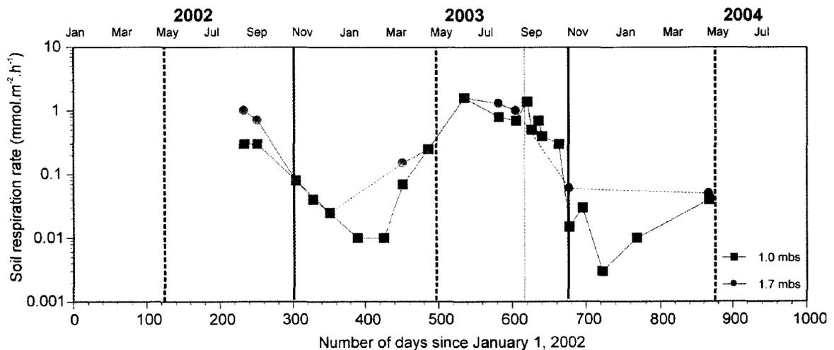
**Figure 5-7** Soil respiration rates (mmol.m<sup>-2</sup>.h<sup>-1</sup>) calculated with the diffusion model using measured concentrations of soil CO<sub>2</sub> from samples collected at 1.0 and 1.7 mbs at the background site at Edam. The dashed lines on the graph connect points where analytical results from the deep probe are missing due to flooding and/or freezing of the probe. The vertical solid and dashed lines correspond to the onset of freezing and complete soil thawing, respectively.
