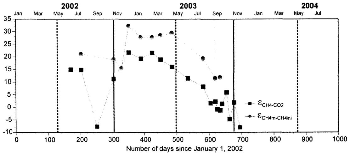
**Figure 3-35** A comparison between  $\epsilon_{\text{CH}_4\text{-CH}_4\text{ini}}$  and  $\epsilon_{\text{CH}_4\text{-CO}_2}$  values estimated for samples collected from the shallow probe A11 at the research site near well A4.
