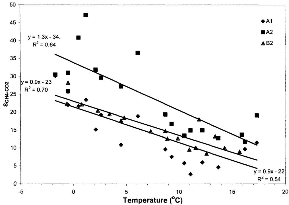
**Figure 3-32** Apparent kinetic isotope effect,  $\epsilon_{\text{CH}_4\text{-CO}_2}$  vs. temperature for gas samples collected from different domains of the microaerophilic soil near well A3.
