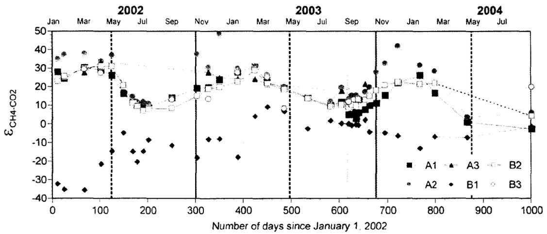
**Figure 3-30** Apparent kinetic isotope effect  $\epsilon_{\text{CH}_4\text{-CO}_2}$  for samples collected from the microaerophilic (solid symbols) and oxygen-rich (hollow symbols) soil near well A3.
