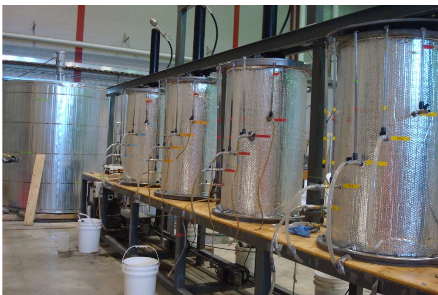
Figure 4-3. Showing leachate inflow port at the base of the columns
