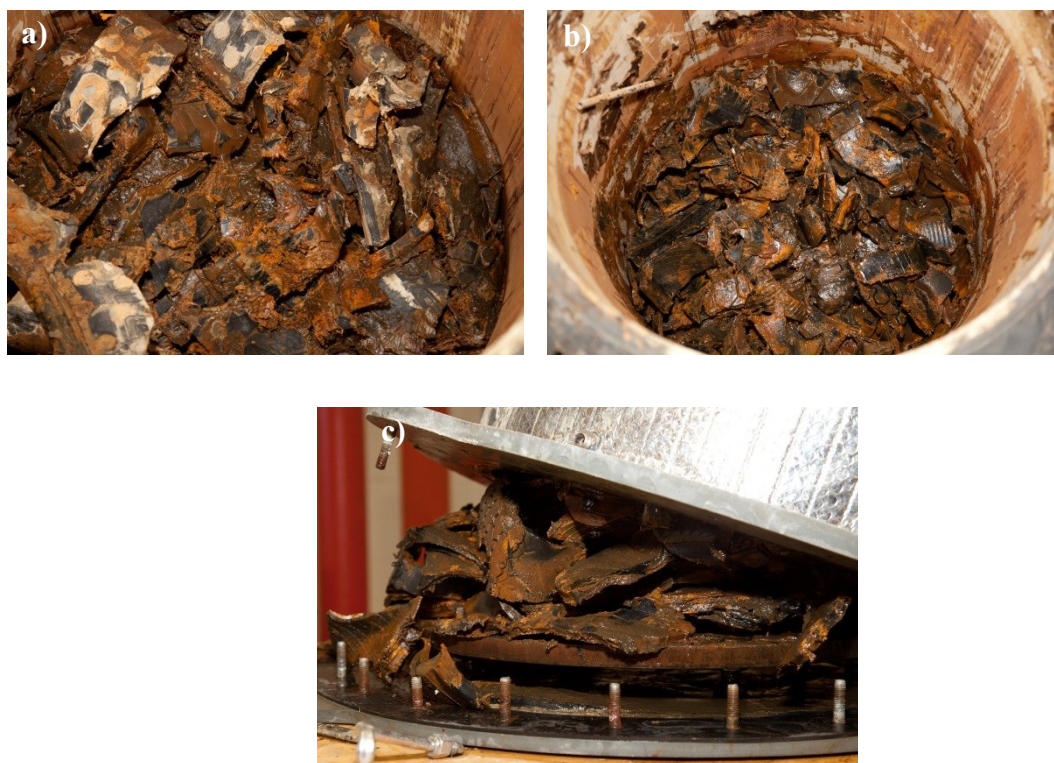
Figure 4-28. Visual examination of clogging in the PLTT column: a) top of the media, b) middle of the media and c) bottom of the media.
