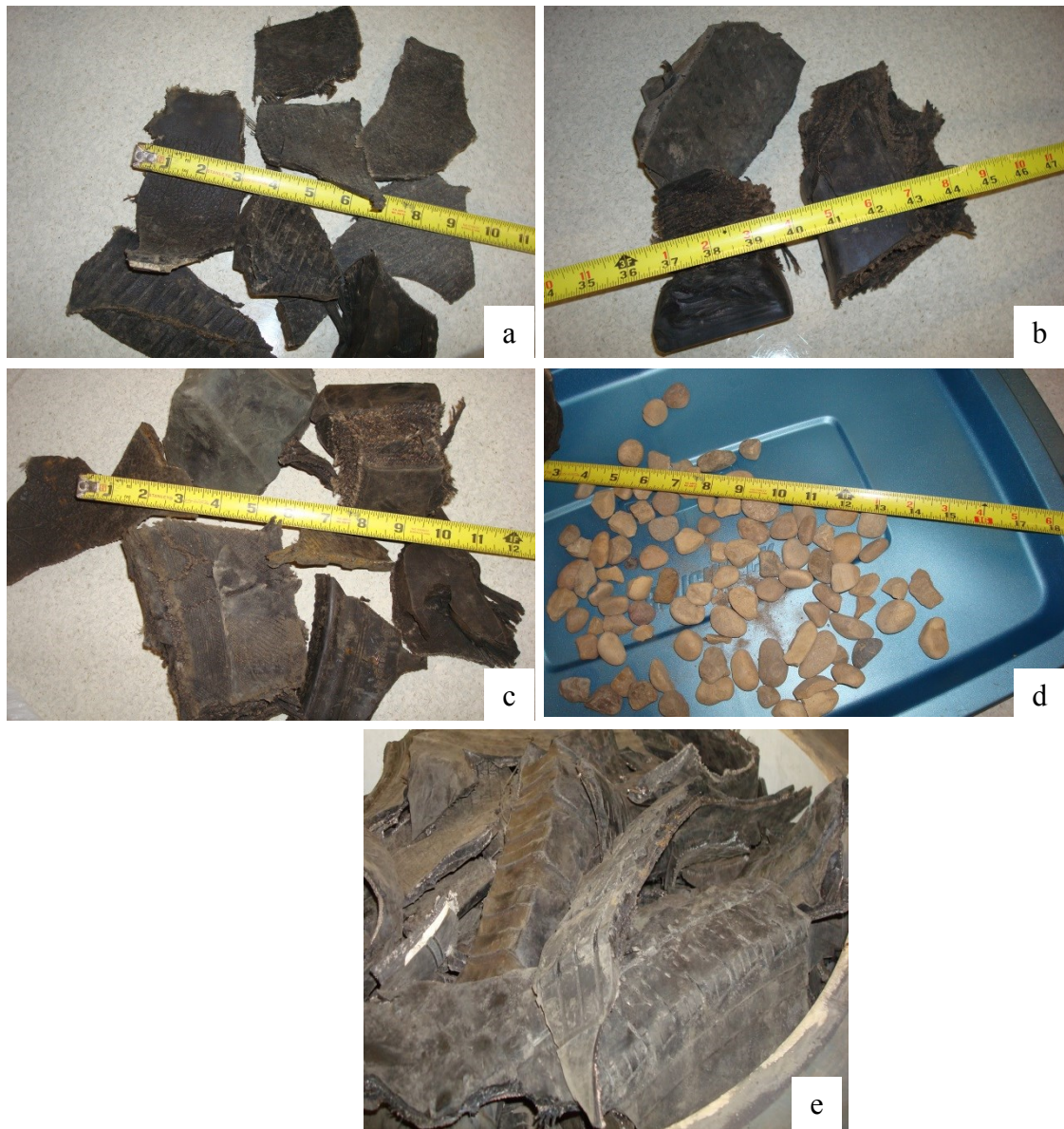
Figure 3-1. Photographs of the test materials: a) PLTT-flat and elongated shape and clean cut edges, b) OTR-block shape and roughly cut edges, c) OTR+PLTT -a mixture of OTR and PLTT on 50:50 by weight basis, d) gravel (clean river bed gravel), e) MTT-flat and elongated shape and clean cut edges.
