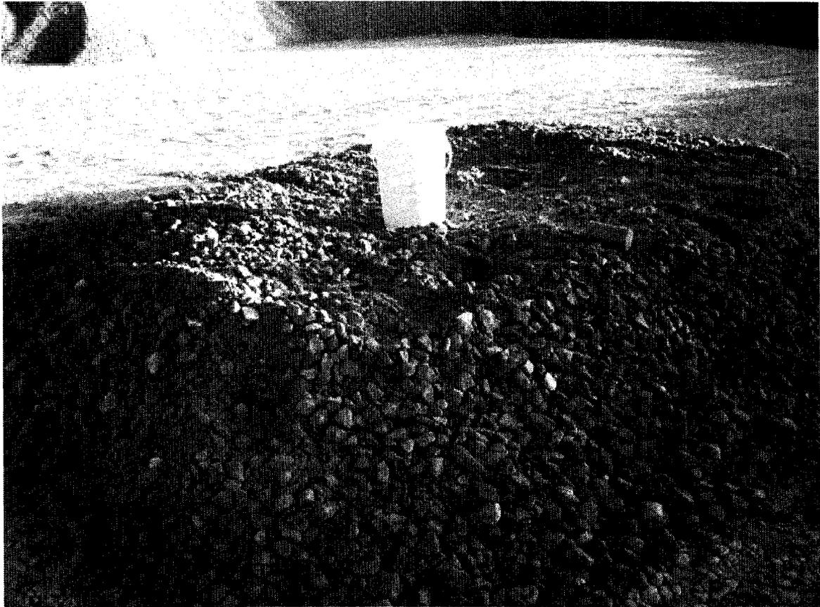
Figure 4.27 Sampling pad of CRF aggregate for its gradation
