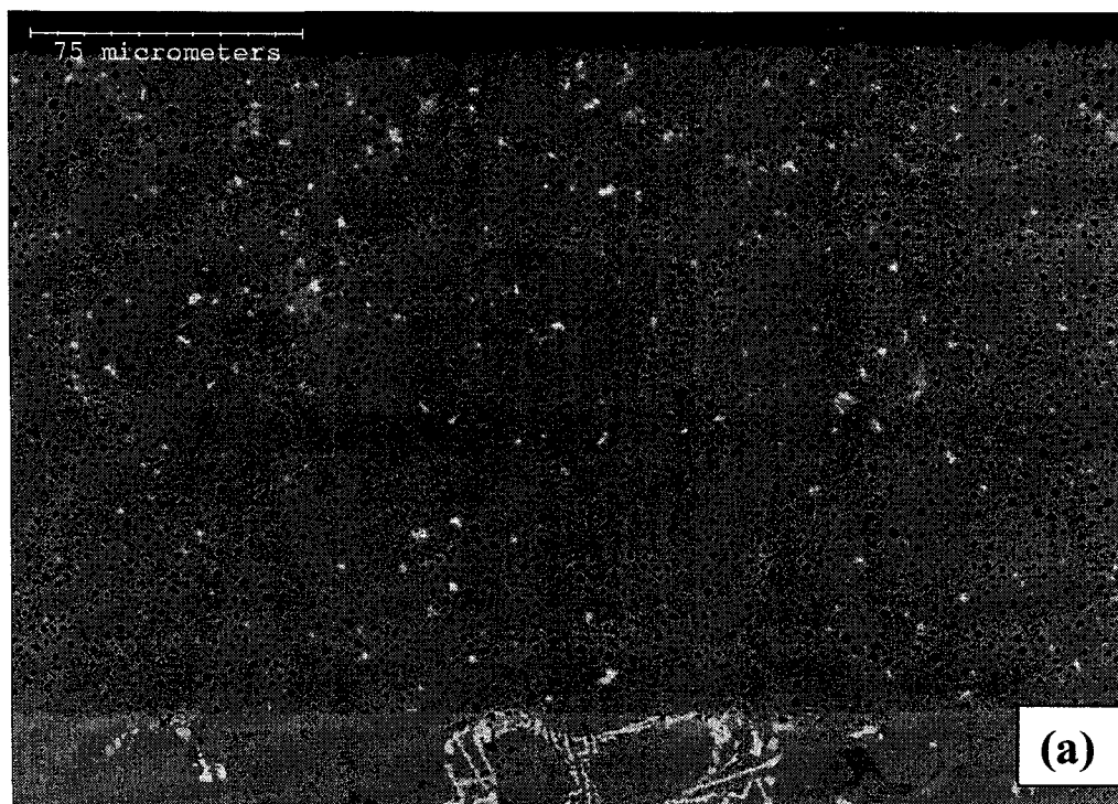
Figure 4-1. The typical morphologies of annealed Ni-Al and Ni-Al-CeO 2 composite coatings: (a) the pure Ni 3 Al coating (80+0); (b) the 80+5 (5 μm) coating.
