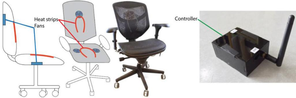
Figure 2.1: This image from [86] shows heating and cooling elements of the personal comfort system (left side) and the controller with wireless connectivity (right side).
