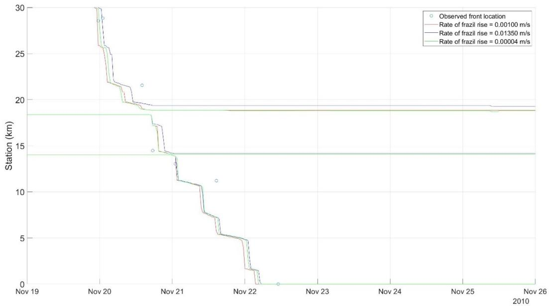
Figure 3-57. Ice front propagation sensitivity analysis: rate of frazil rise.
