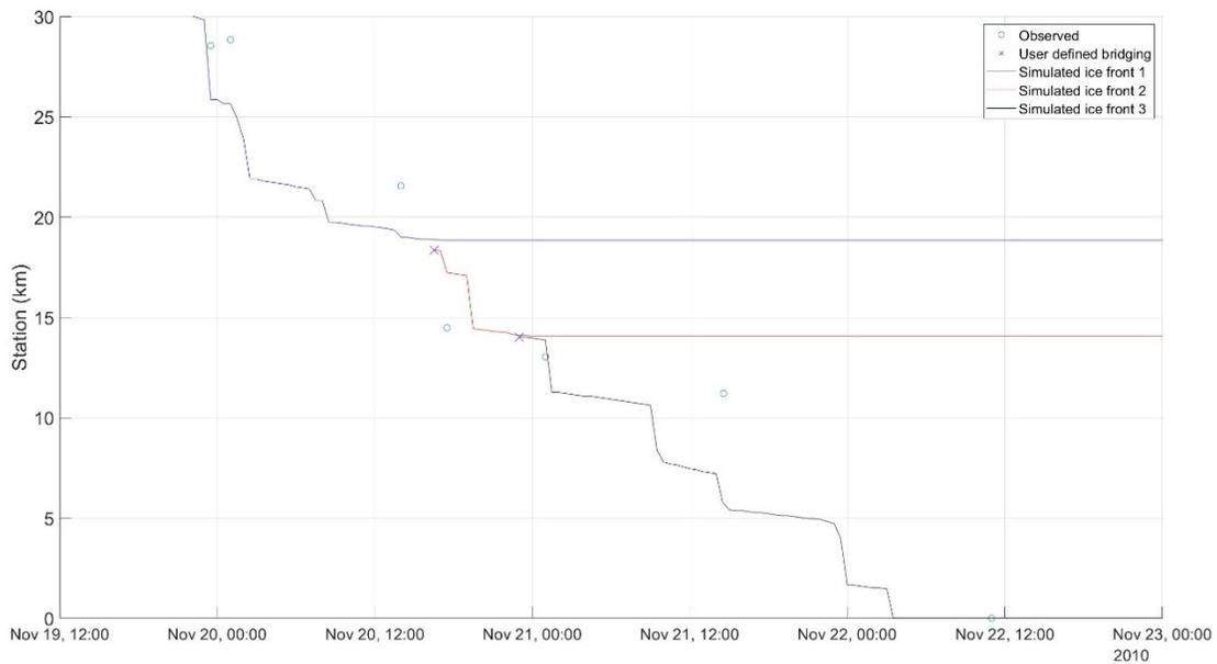
Figure 3-14. Simulated ice front propagation, freeze-up 2010-11.
