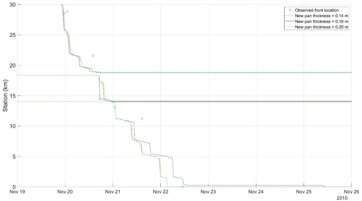
Figure 3-55. Ice front propagation sensitivity analysis: thickness of newly formed ice pans.
