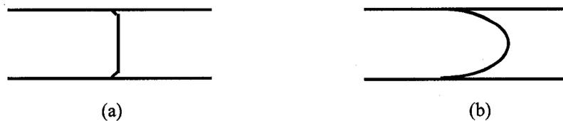
Fig. 1.2 Flow profile of EOF (a) compared to pressure driven flow (b)
