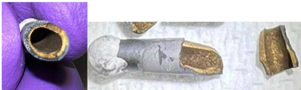
Figure 5-7 Fractured cell after electrochemical reduction
