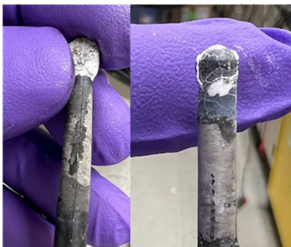
Figure 5-4 Some failures during electrochemical reduction.
