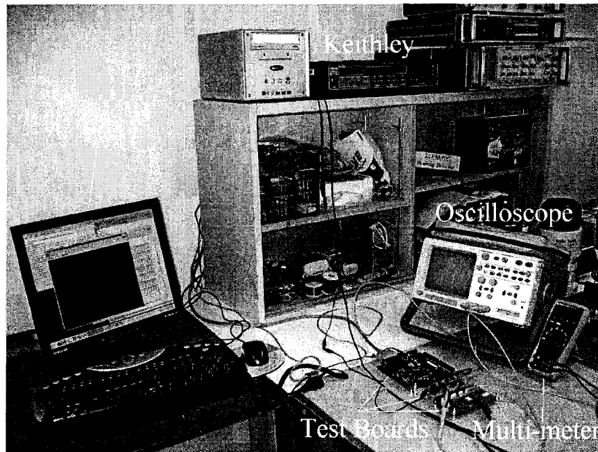
Figure 6.2 Picture of test set-up: PC, Keithley unit, FPGA board, test support board, PCB, multi-meter, and oscilloscope
