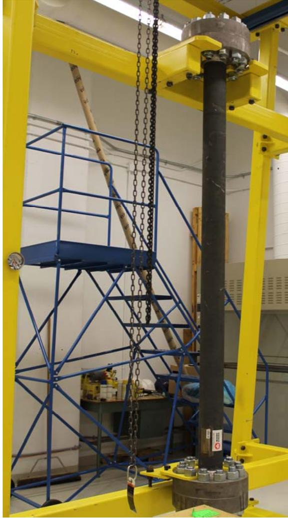
**Figure 3.3. The extraction vessel of the SFE process (Length: 2.45 m, Inner diameter: 0.0833 m)**
