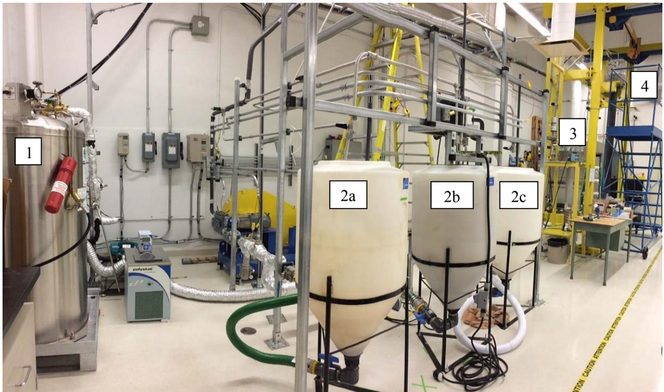
**Figure 3.2.** The pilot scale SFE process for treatment of drill cuttings (1) CO<sub>2</sub> tank, (2a) rinse water tank, (2b) slurry feed tank, (2c) treated slurry tank, (3) separator and (4) extraction vessel
