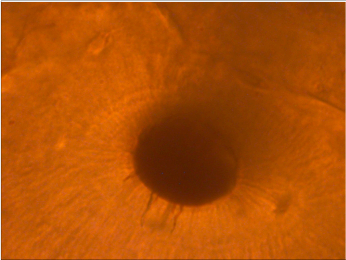
Figure 6: A Haversian canal showing several cracks at its periphery from the initial exploratory study involving pig femora and freeze and thaw cycles. (Source: from this study. Light microscopy. Original magnification: 630x)
