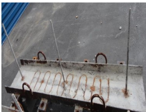
Figure 3.34 – Footing details in Hoque’s experimental study (Hoque 2013)
