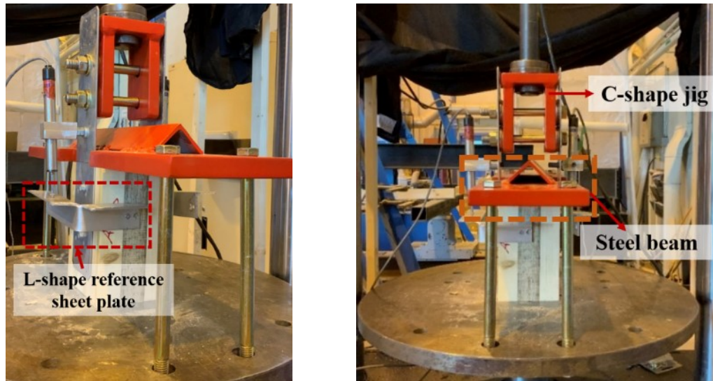
Figure 3.4 Connection test setup
