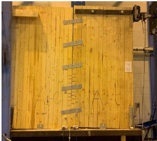
c) Kinematic wall behaviour (SW)
