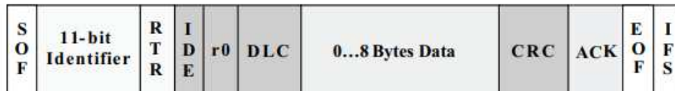
Figure 9 Standard CAN structure (CAN 2.0A): 11-Bit Identifier (Corrigan, 2016)
