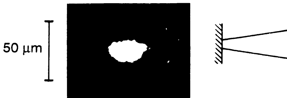
Figure 6.4. X-ray pinhole picture of the plasma produced by the laser at normal incidence from reference 62.
