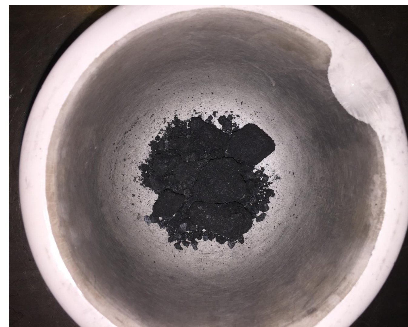
Figure 1 – Sample being ground in mortar and pestle to get particle sizes between 2mm and 0.3mm in diameter
