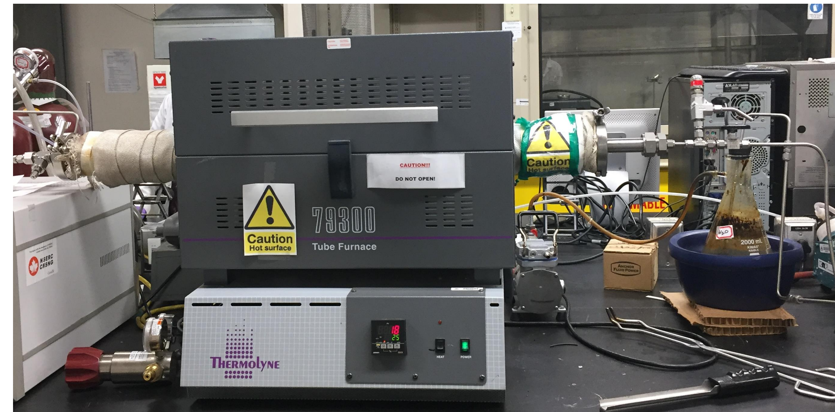
Figure 4 – Lab scale Furnace (Thermolyne 79300 Tube Furnace); the samples are placed inside on the furnace through the side tube. The tube is then sealed and nitrogen gas is passed through. After the nitrogen passes through the furnace it goes through the tubing into the water bath before venting into fume hood.
