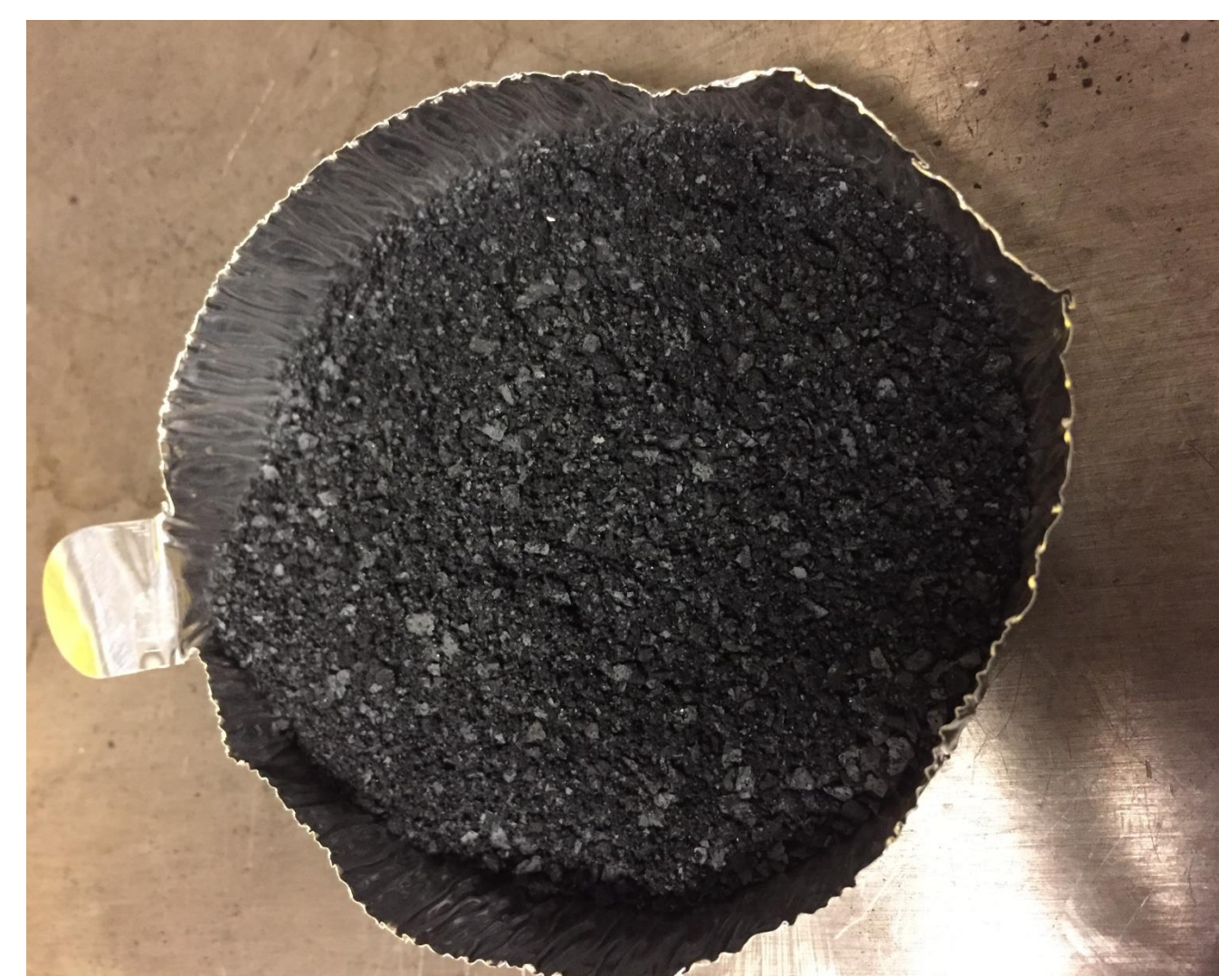
Figure 2 – Sample after being dried in the furnace for 2h at 105°C to remove moisture
