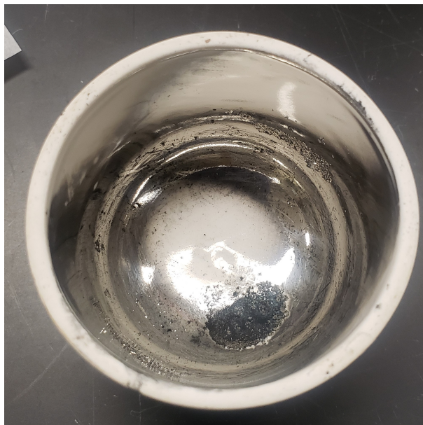
Figure 4.2: Mirror-like finish formed on the walls of the crucible due to evaporation and deposition of Ir when calcined in the furnace directly at 400°C.
