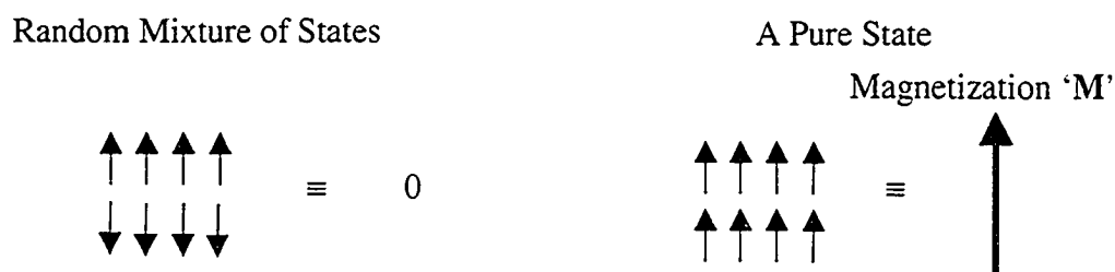
Figure 1-2 An energy level representation of spin \frac{1}{2} thermal equilibrium in a static magnetic field B_0 . The relative contributions from the random mixture and pure states are a function of B_0 , the system temperature, T , and the spin gyromagnetic ratio, \gamma .
