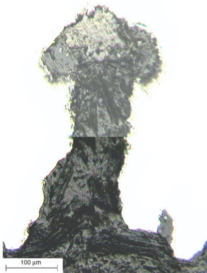
Figure 2.23 Blunted, the balloon-shaped crack propagated in the NNpH environment [45]
