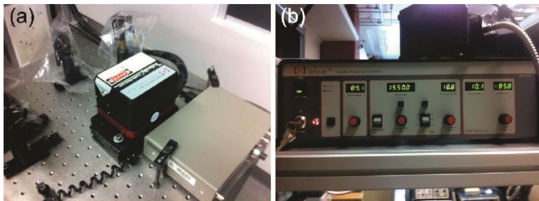
Figure 2.3: (a) Velocity™ Tunable Diode Laser and (b) laser controller.
