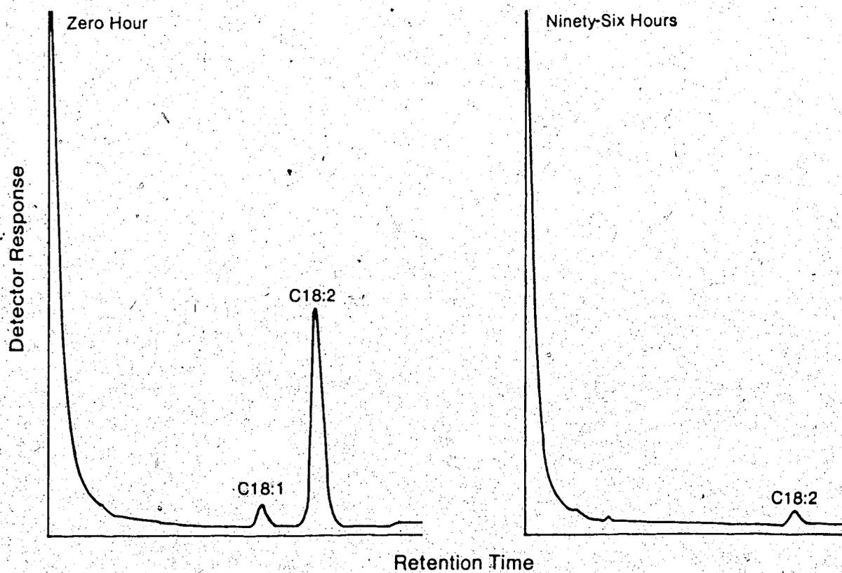
Figure 3.5. Chromatograms of 95 Percent Linoleic Acid Toxicity Test at the Zero Hour and Ninety-six Hour Period at a pH of 8.79 (Sample diluted to 5 ml in Isooctane)
