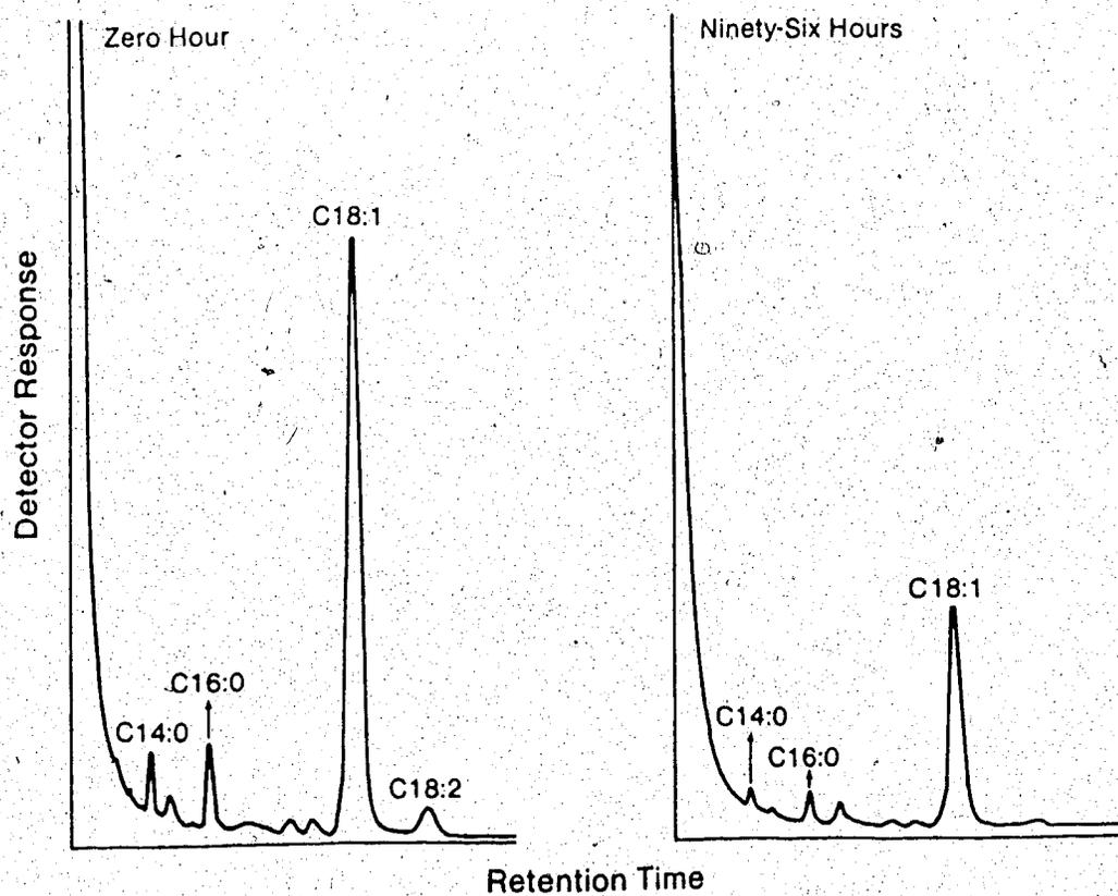
Figure 3.3 Chromatograms of Oleic Acid Toxicity Test at the Zero Hour and Ninety-Six Hour Period at a pH of 8.69 (Sample diluted to 10 ml in Isooctane)
