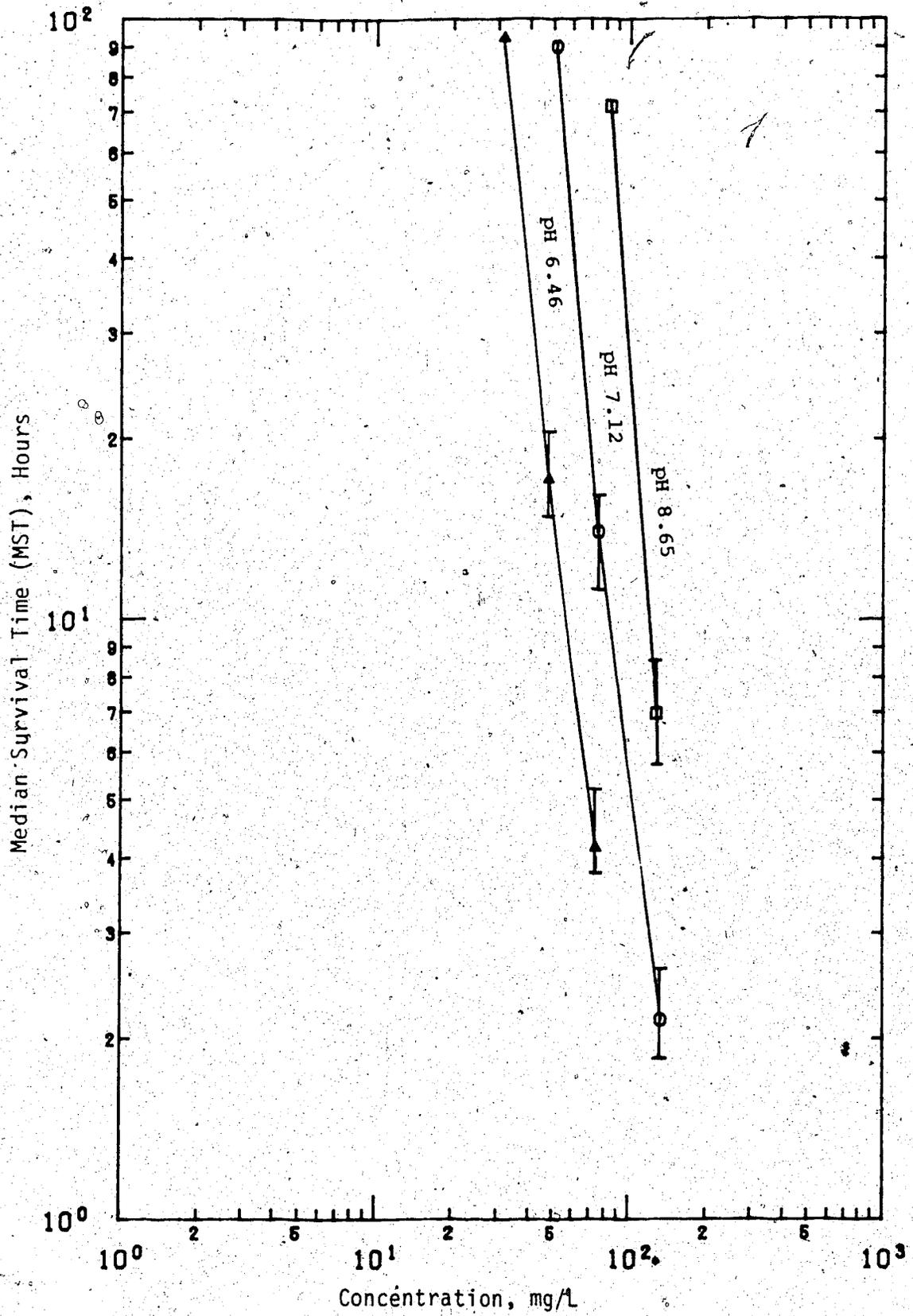
Figure 3.6 Mortality Curves of Oleic Acid to Rainbow Trout Fingerlings (Vertical Bars represent 95 percent confidence intervals)
