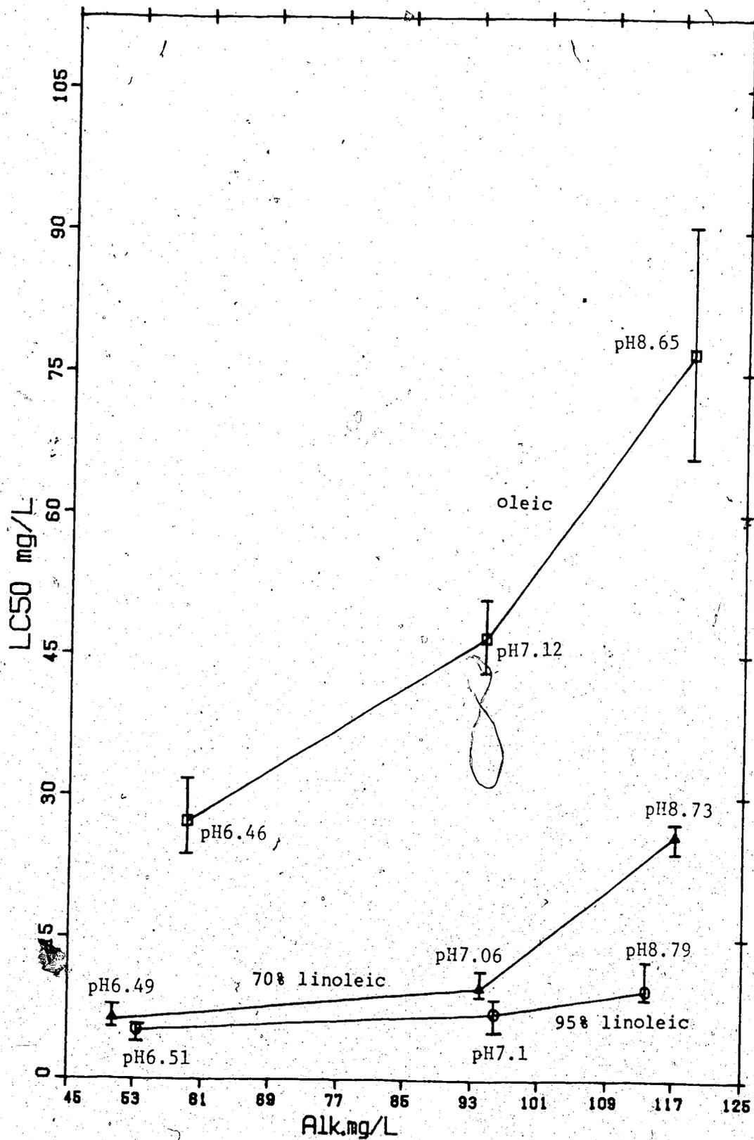
Figure 3.11 Relationship of Alkalinity Values of Test Water to LC50 Geometric Mean Values of Oleic and Linoleic Acids with Rainbow Trout Fingerlings (Vertical bars represent standard deviation for oleic acid and ranges for linoleic acid)
