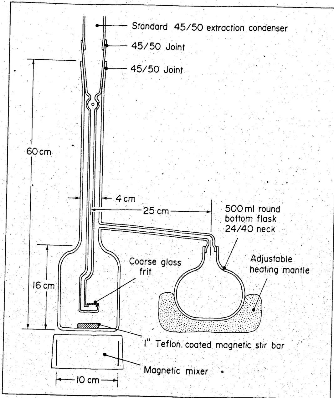
Figure 2.1 Continuous Liquid-Liquid Extraction Apparatus
