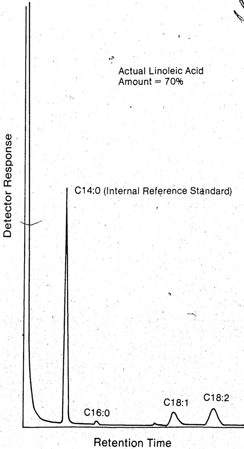
Figure 3.2 Chromatograms of 70 Percent Test Linoleic Acid Composition
