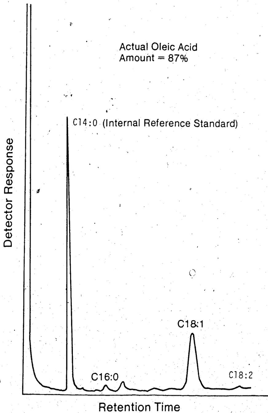
Figure 3.1 Chromatograms of Test Oleic Acid Composition
