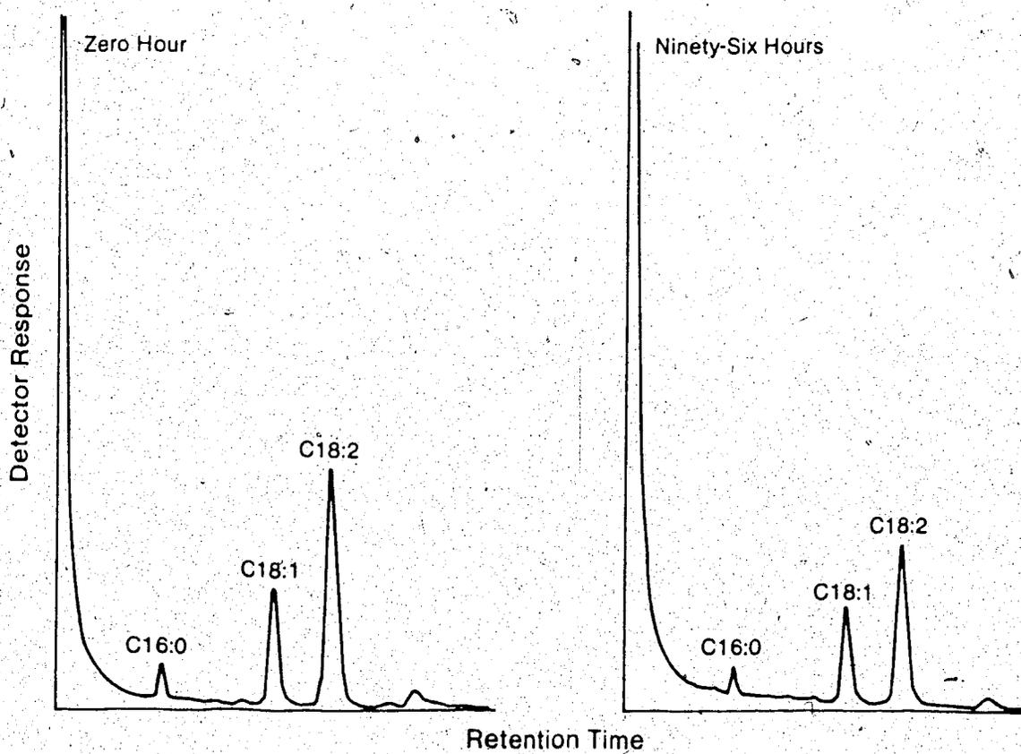
Figure 3.4 Chromatograms of 70 Percent Linoleic Acid Toxicity Test at the Zero Hour and Ninety-six Hour Period at a pH of 8.74 (Sample diluted to 10 ml in Isooctane)
