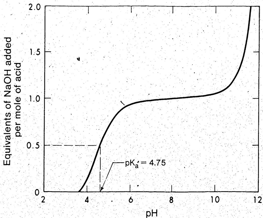
Figure 1.5 Titration of 0.004M Acetic Acid with Sodium Hydroxide at 25°C (Daniels and Alberty, 1966)
