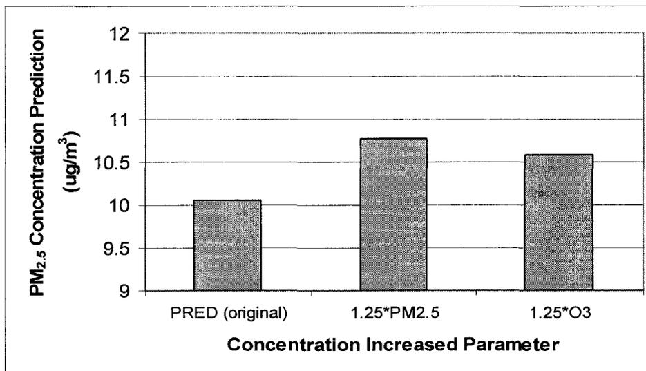
**Figure 25** Predicted mean hourly PM<sub>2.5</sub> concentration at the Fort McKay station using ANN sub-model based on category #2 data for 25% increase in PM<sub>2.5</sub> and O<sub>3</sub> concentration at AMS #13.
