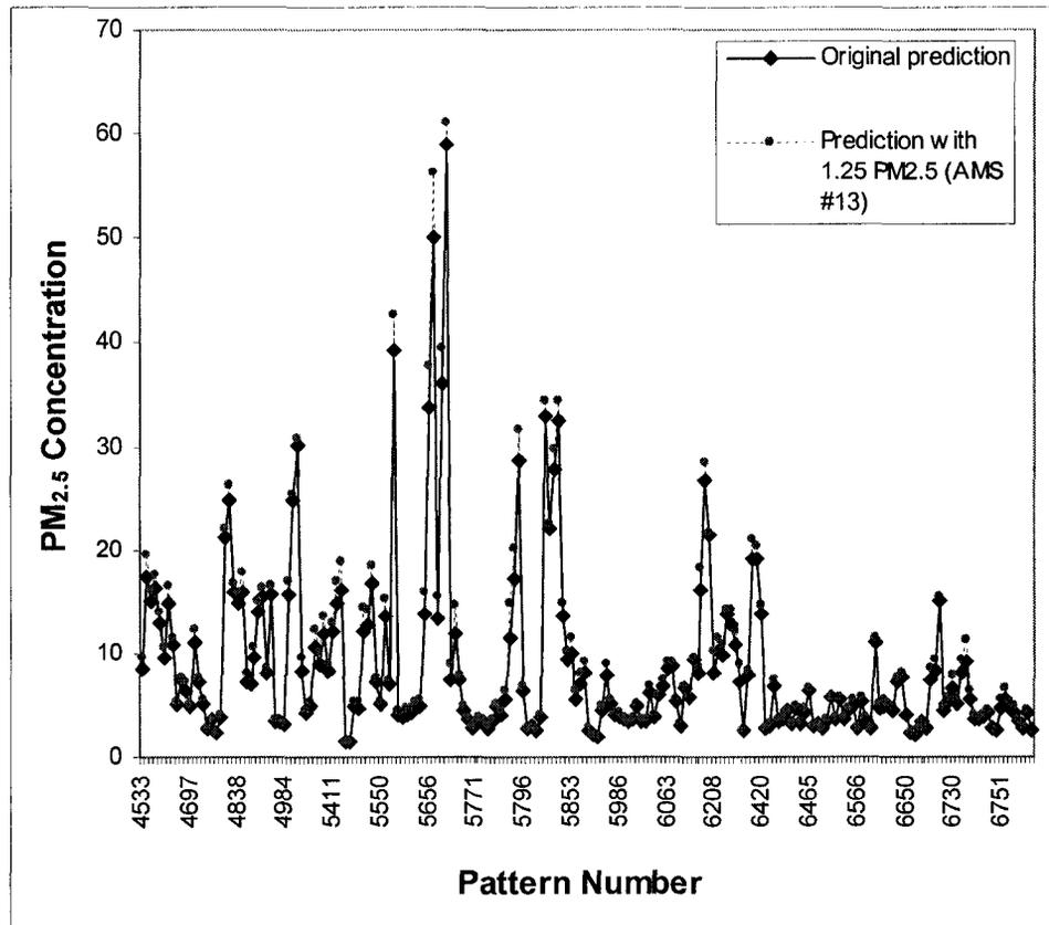
**Figure A28. PM<sub>2.5</sub> concentrations at Fort McKay station [µg/m<sup>3</sup>] based on sensitivity analysis of ANN sub-model using category #1 data (205 data patterns) – original prediction versus simulated 25% increase in PM<sub>2.5</sub> concentrations at AMS #13 for peak events at AMS #1.**
