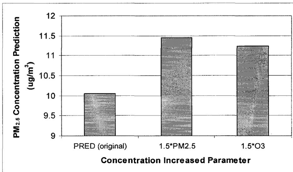
**Figure 26** Predicted mean hourly PM<sub>2.5</sub> concentration at the Fort McKay station using ANN sub-model based on category #2 data for 50% increase in PM<sub>2.5</sub> and O<sub>3</sub> concentration at AMS #13.
