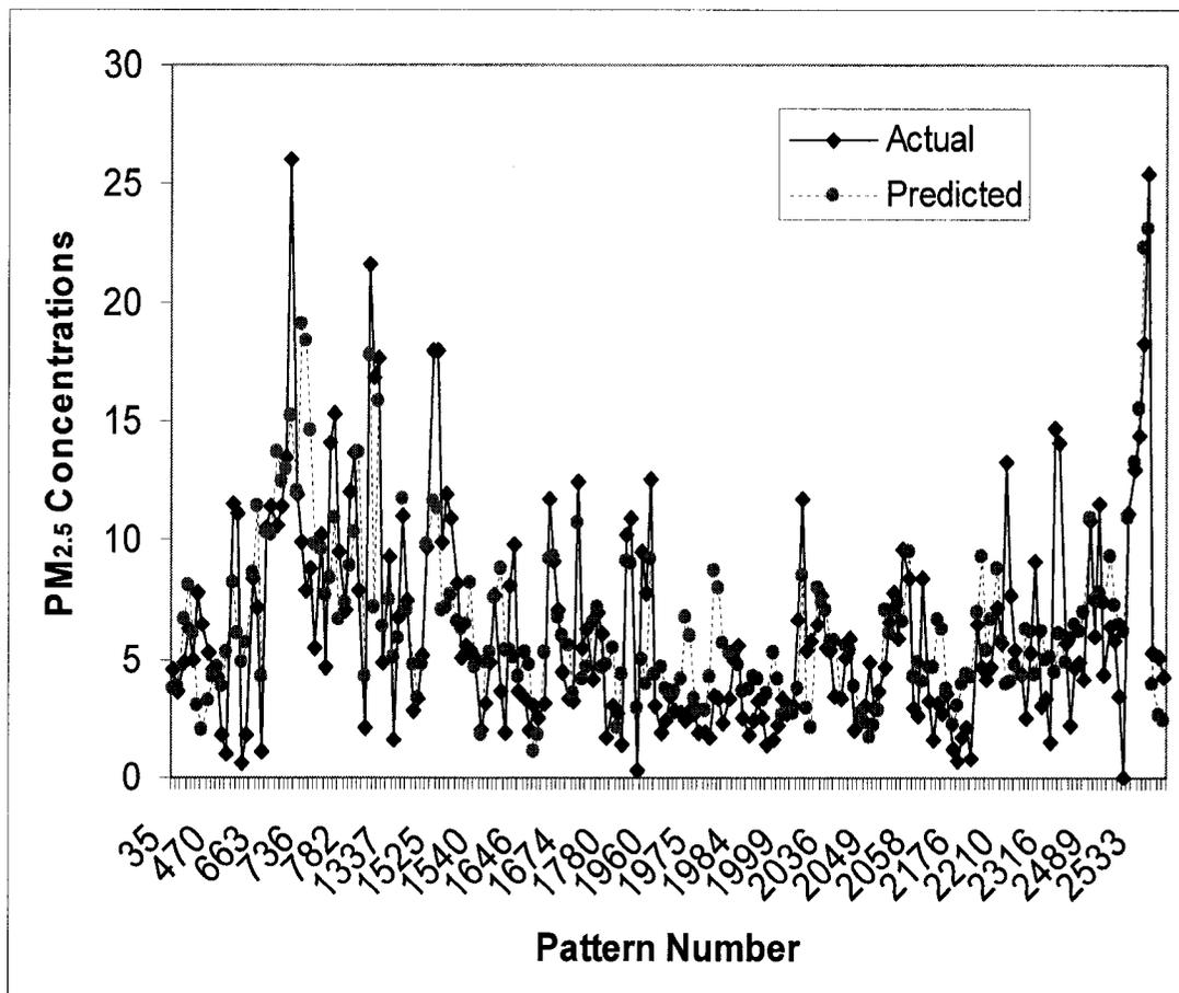
**Figure 19** Actual versus predicted hourly PM<sub>2.5</sub> concentrations at Fort McKay [µg/m<sup>3</sup>] for ANN model using category #2 data (205 data patterns) corresponding to typical range of fluctuation observed in PM<sub>2.5</sub> levels.
