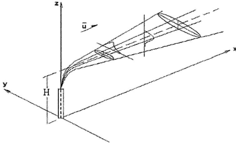
**Figure 5. Gaussian dispersion of a point source located at  $(0, 0, H)$  in a wind-oriented coordinate system (adapted from Dobbins, 1976).**
