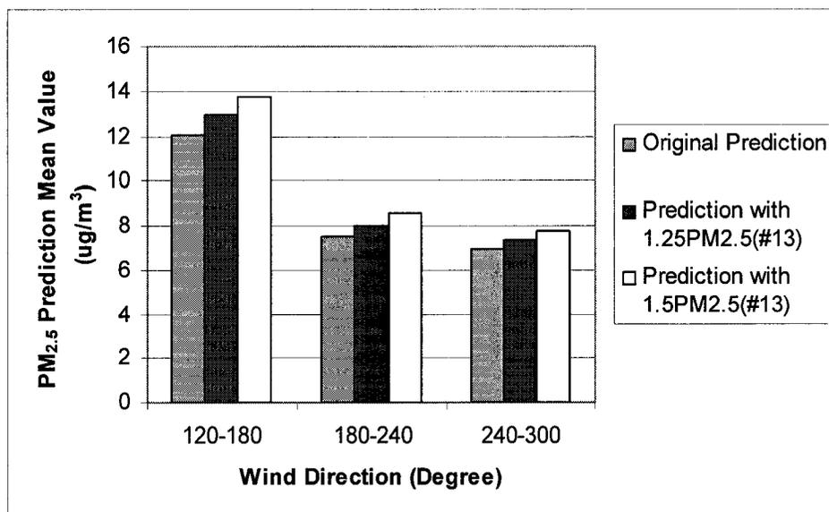
**Figure 33** Predicted mean hourly PM<sub>2.5</sub> concentration at the Fort McKay station using ANN sub-model based on category #2 data for 25% and 50% increase in PM<sub>2.5</sub> concentration at AMS #13 and for winds originating from three 60°-angles ranges.
