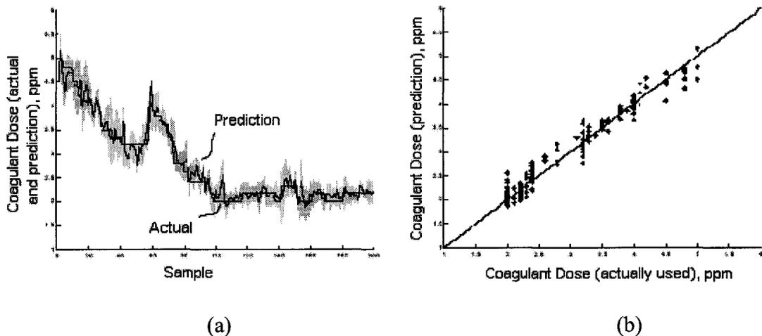
**Figure 7. Result from the ANN model - Actual vs. Prediction for a water treatment application (adapted from Valentin et al., 1999).**
