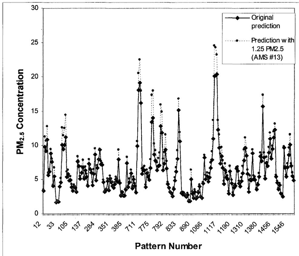
**Figure A27. PM<sub>2.5</sub> concentrations at Fort McKay station [ $\mu\text{g}/\text{m}^3$ ] based on sensitivity analysis of ANN sub-model using category #1 data (205 data patterns) – original prediction versus simulated 25% increase in PM<sub>2.5</sub> concentrations at AMS #13 for typical conditions at AMS #1.**
