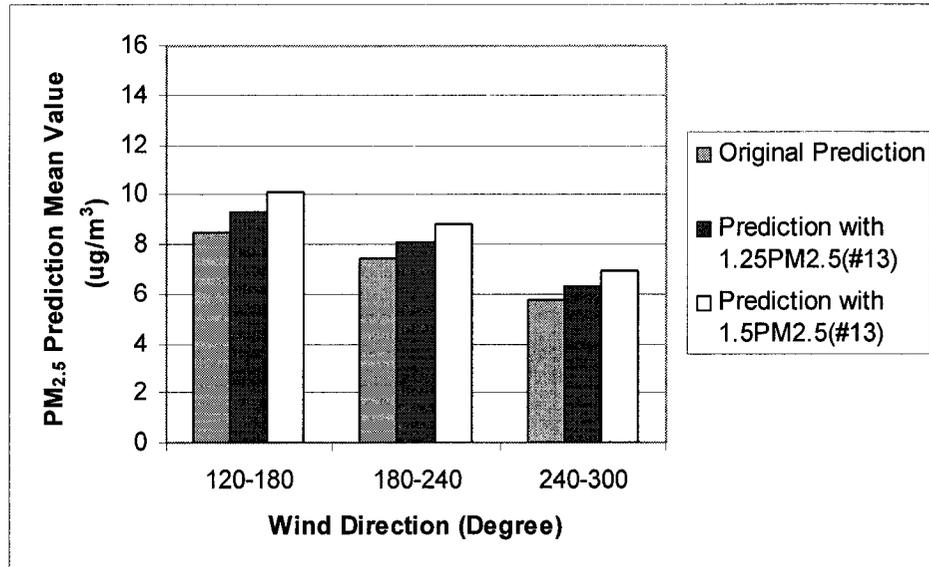
**Figure 32** Predicted mean hourly  $PM_{2.5}$  concentration at the Fort McKay station using ANN sub-model based on category #1 data for 25% and 50% increase in  $PM_{2.5}$  concentration at AMS #13 and for winds originating from three 60°-angles ranges.
