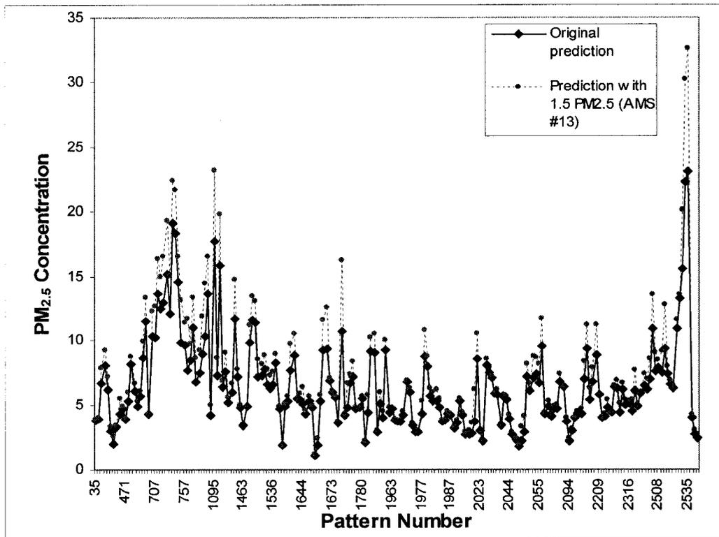
**Figure 27** PM<sub>2.5</sub> concentrations at Fort McKay station [µg/m<sup>3</sup>] based on sensitivity analysis of ANN sub-model using category #2 data (205 data patterns) – original prediction versus simulated 50% increase in PM<sub>2.5</sub> concentrations at AMS #13 for typical conditions at AMS #1.
