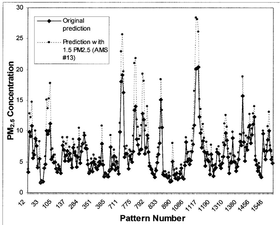
**Figure 23** PM<sub>2.5</sub> concentrations at Fort McKay station [µg/m<sup>3</sup>] based on sensitivity analysis of ANN sub-model using category #1 data (205 data patterns) – original prediction versus simulated 50% increase in PM<sub>2.5</sub> concentrations at AMS #13 for typical conditions at AMS #1.
