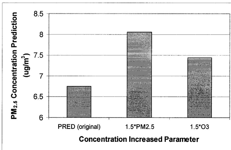
**Figure 22** Predicted mean hourly PM<sub>2.5</sub> concentration at the Fort McKay station using ANN sub-model based on category #1 data for 50% increase in PM<sub>2.5</sub> and O<sub>3</sub> concentration at AMS #13.
