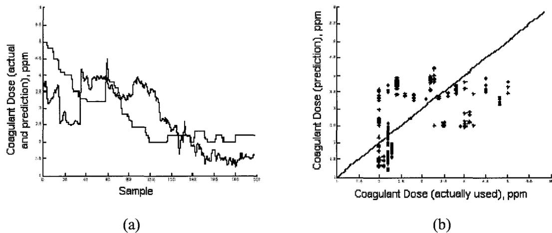
**Figure 8. Result from the linear regression model- Actual vs. Prediction for a water treatment application (adapted from Valentin et al., 1999).**
