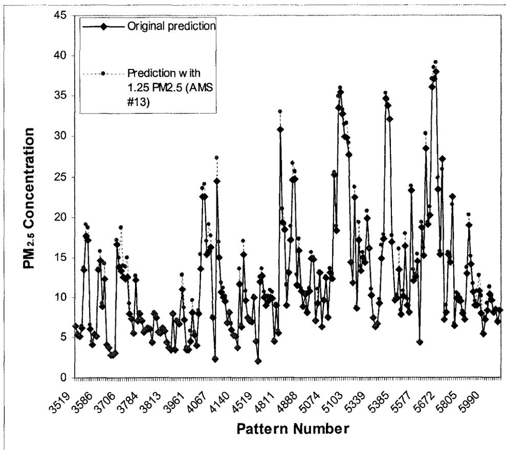
**Figure A30. PM<sub>2.5</sub> concentrations at Fort McKay station [ $\mu\text{g}/\text{m}^3$ ] based on sensitivity analysis of ANN sub-model using category #2 data (205 data patterns) – original prediction versus simulated 25% increase in PM<sub>2.5</sub> concentrations at AMS #13 for peak events at AMS #1.**
