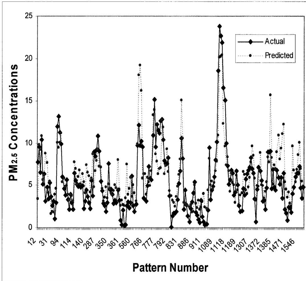
**Figure 17. Actual versus predicted hourly PM<sub>2.5</sub> concentrations at Fort McKay [ $\mu\text{g}/\text{m}^3$ ] for ANN sub-model using category #1 data (205 data patterns) corresponding to typical range of fluctuation observed in PM<sub>2.5</sub> levels.**
