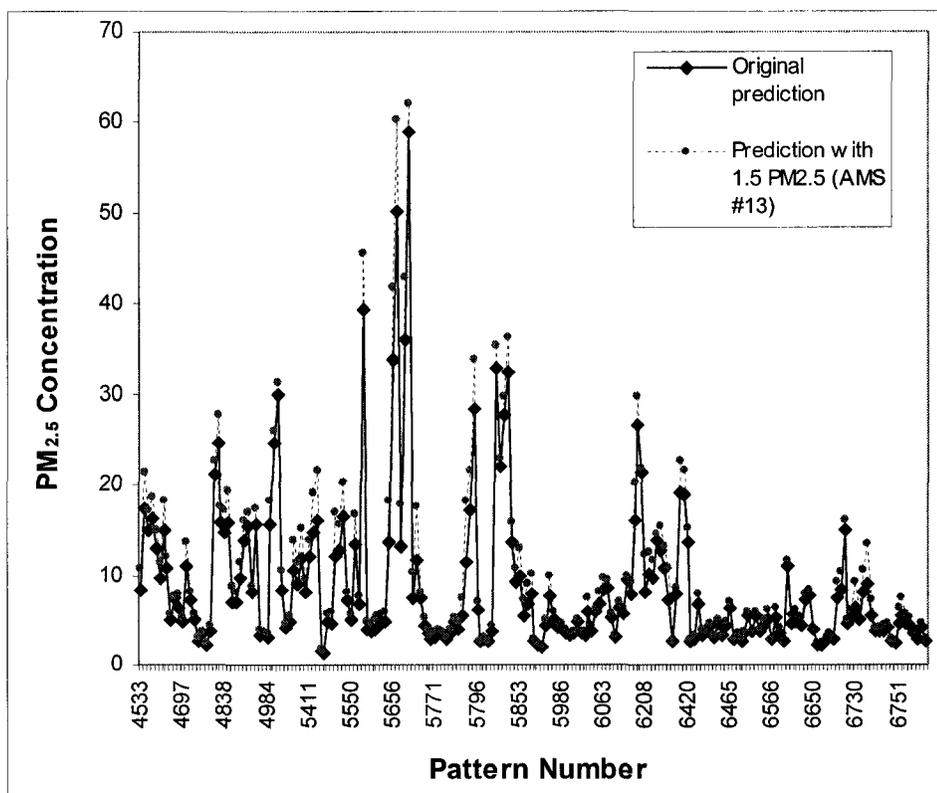
**Figure 24** **PM<sub>2.5</sub> concentrations at Fort McKay station [µg/m<sup>3</sup>] based on sensitivity analysis of ANN sub-model using category #1 data (205 data patterns) – original prediction versus simulated 50% increase in PM<sub>2.5</sub> concentrations at AMS #13 for peak events at AMS #1.**
