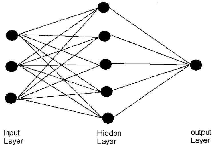
**Figure 6. Basic structure for a multilayer perceptron ANN.**
