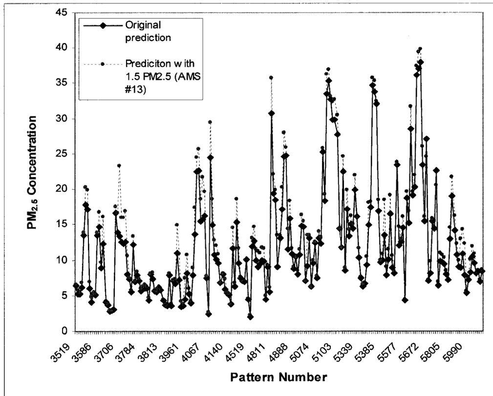
**Figure 28**  $PM_{2.5}$  concentrations at Fort McKay station [ $\mu\text{g}/\text{m}^3$ ] based on sensitivity analysis of ANN sub-model using category #2 data (205 data patterns) – original prediction versus simulated 50% increase in  $PM_{2.5}$  concentrations at AMS #13 for peak events at AMS #1.
