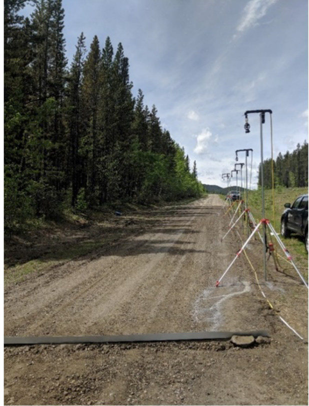
Figure 3-4 Large rainfall simulation setup with I-WOB nozzles attached to PVC pipe that rests on 3m tall steel rods supported by survey tripods spaced 5m apart. a) Trail setup b) Road setup
