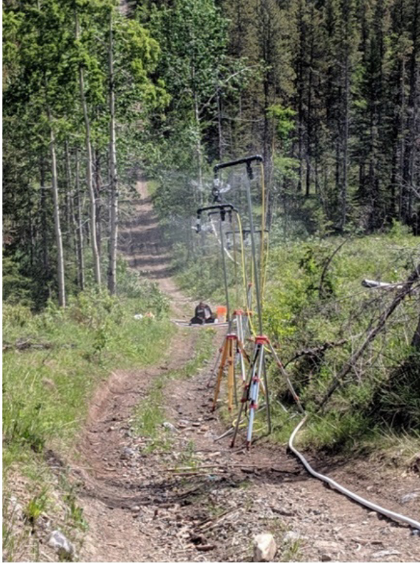
Figure 3-4 Large rainfall simulation setup with I-WOB nozzles attached to PVC pipe that rests on 3m tall steel rods supported by survey tripods spaced 5m apart. a) Trail setup b) Road setup
