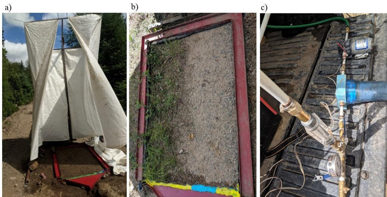
Figure 2-3 Small Rainfall Simulator set up including the a) frame with wind guards, plot frame, and collection pan, b) the plot frame connected to the pan with modelling clay and petroleum jelly, and c) the pump and filtration system.
