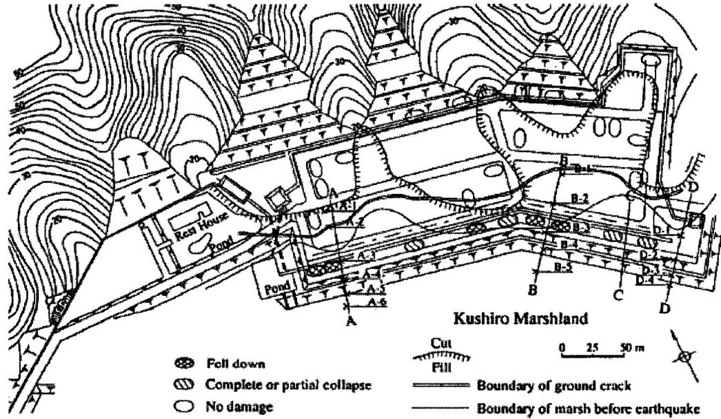
Figure B.63 Damage of the embankment during the Kushiro-Oki earthquake (After Olson 2001)
