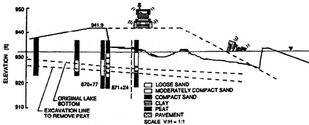
Figure B.33 Pre- and post-failure cross section of the embankment on Ackerman Lake
