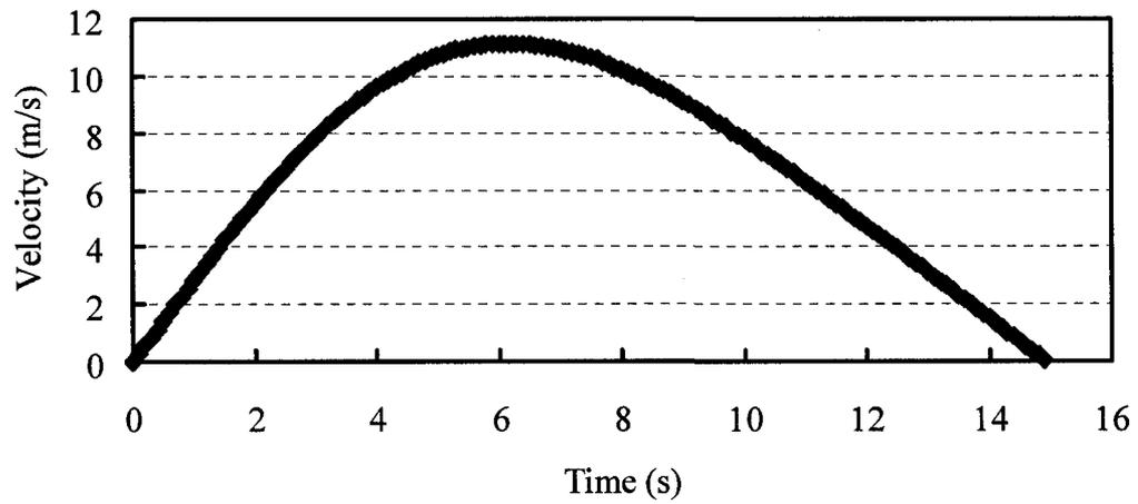
Figure B.22 Centroid velocity versus time for the Calaveras flow slide
