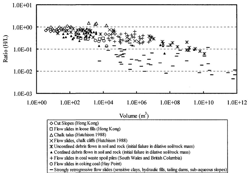
Figure 4-2 Tangent of travel angle ( $H/L$ ) versus landslide volume
