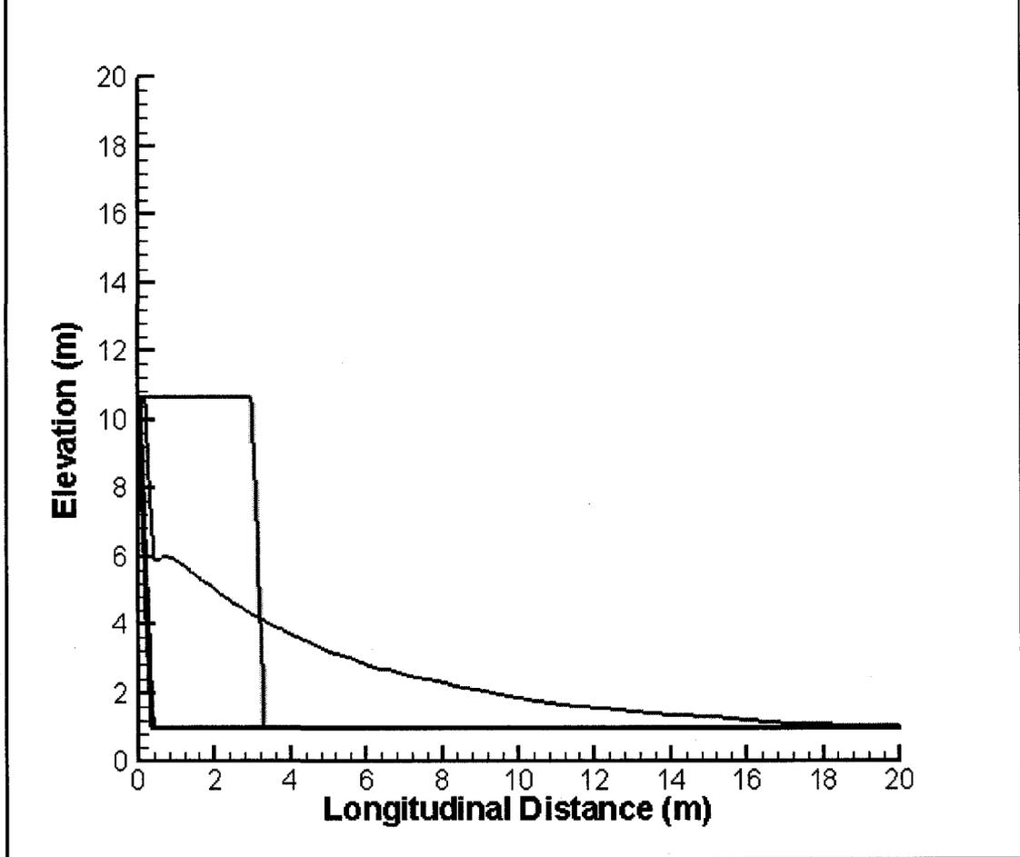
Figure A.15 Simulation of granular spreading mass with initial aspect ratio of 3.2 and height of 9.6 m
