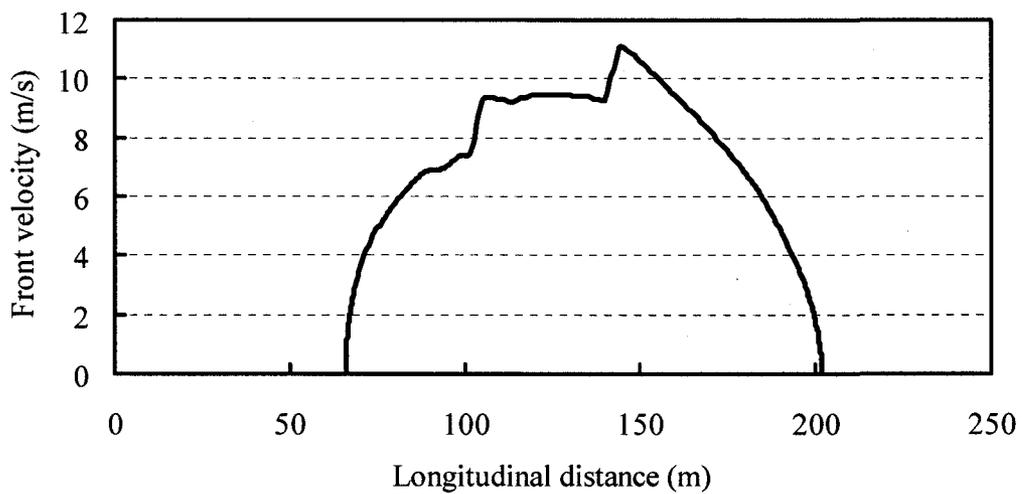
Figure 7-16 Front velocity profile of the Tsukidate landslide based on dynamic analysis
