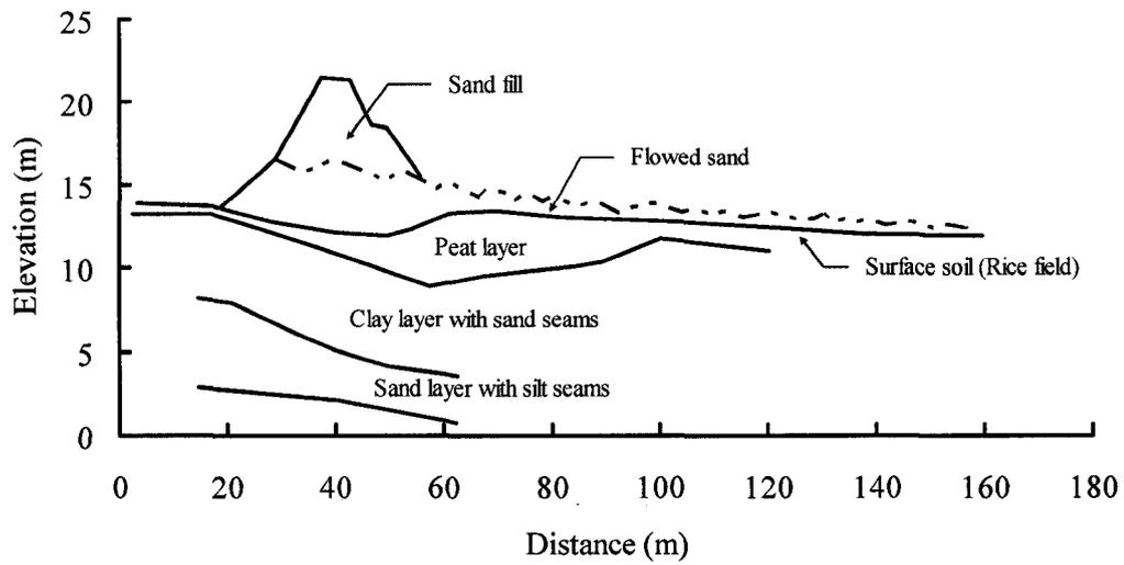
Figure B.53 Pre- and post-failure cross section of the embankment of the Uetsu-Line
