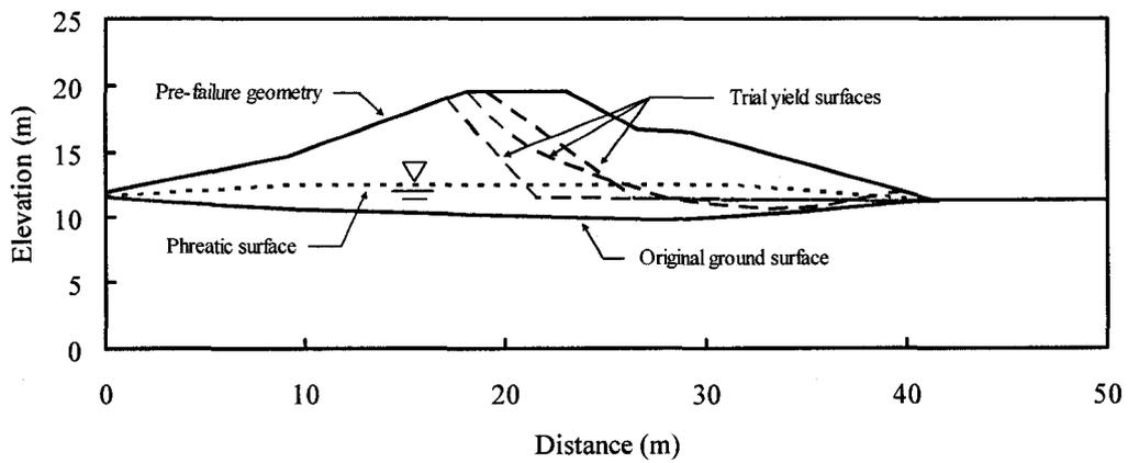
Figure B.54 Pre-failure geometries of the Uetsu-Line embankment used for yield
