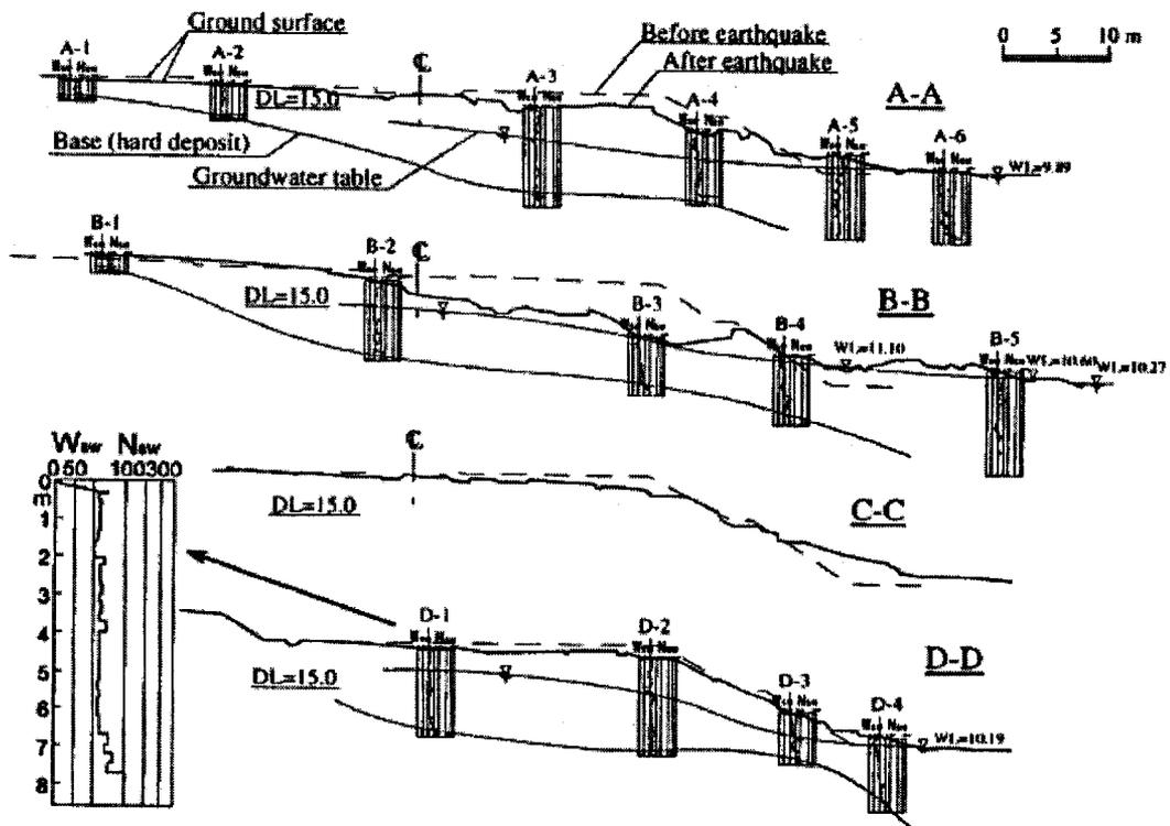
Figure B.64 Cross sections along four profiles in Figure B.63 (After Olson 2001)
