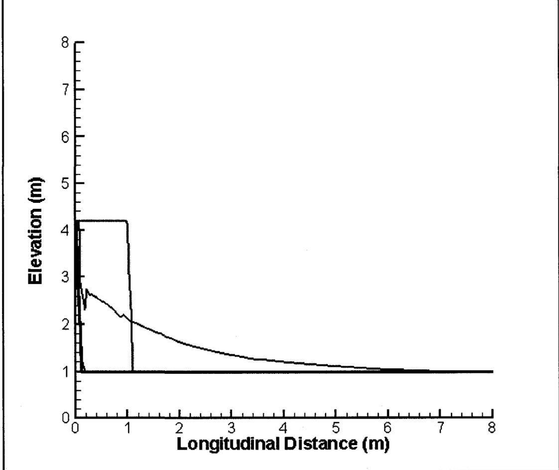
Figure A.13 Simulation of granular spreading mass with initial aspect ratio of 3.2 and height of 3.2 m
