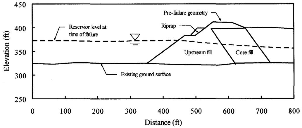
Figure B.9 Pre-failure cross section of the North Dike of the Wachusett Dam
