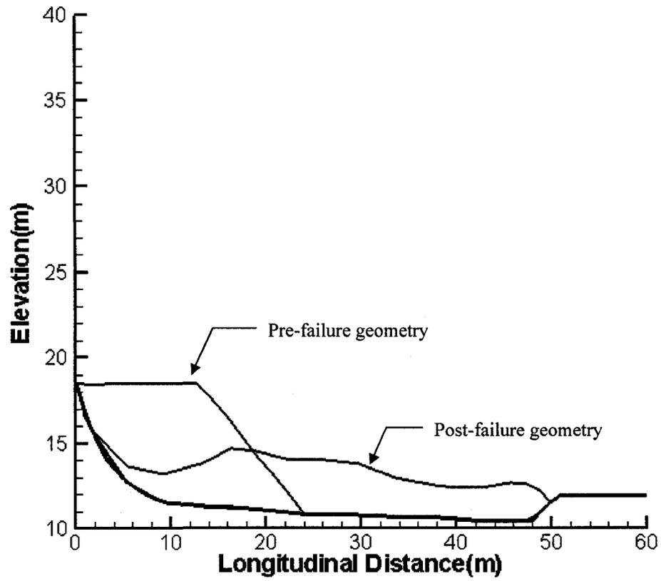
Figure B.79 Geometries of the Route 272 flow slide based on dynamic analysis with the cohesive model
