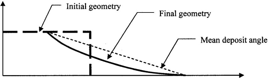
Figure A.12 Definition of the mean angle of dispose
