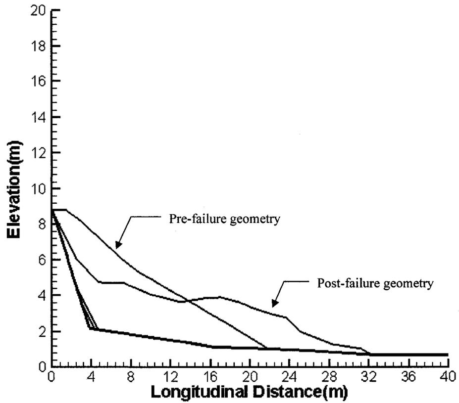
Figure B.38 Geometries of the Lake Ackerman flow slide based on dynamic analysis with the cohesive model
