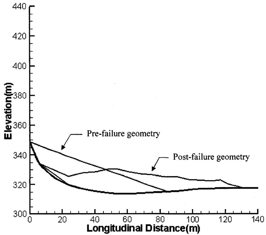
Figure B.4 Geometries of the Lower San Fernando flow slide based on dynamic analysis with the cohesive model
