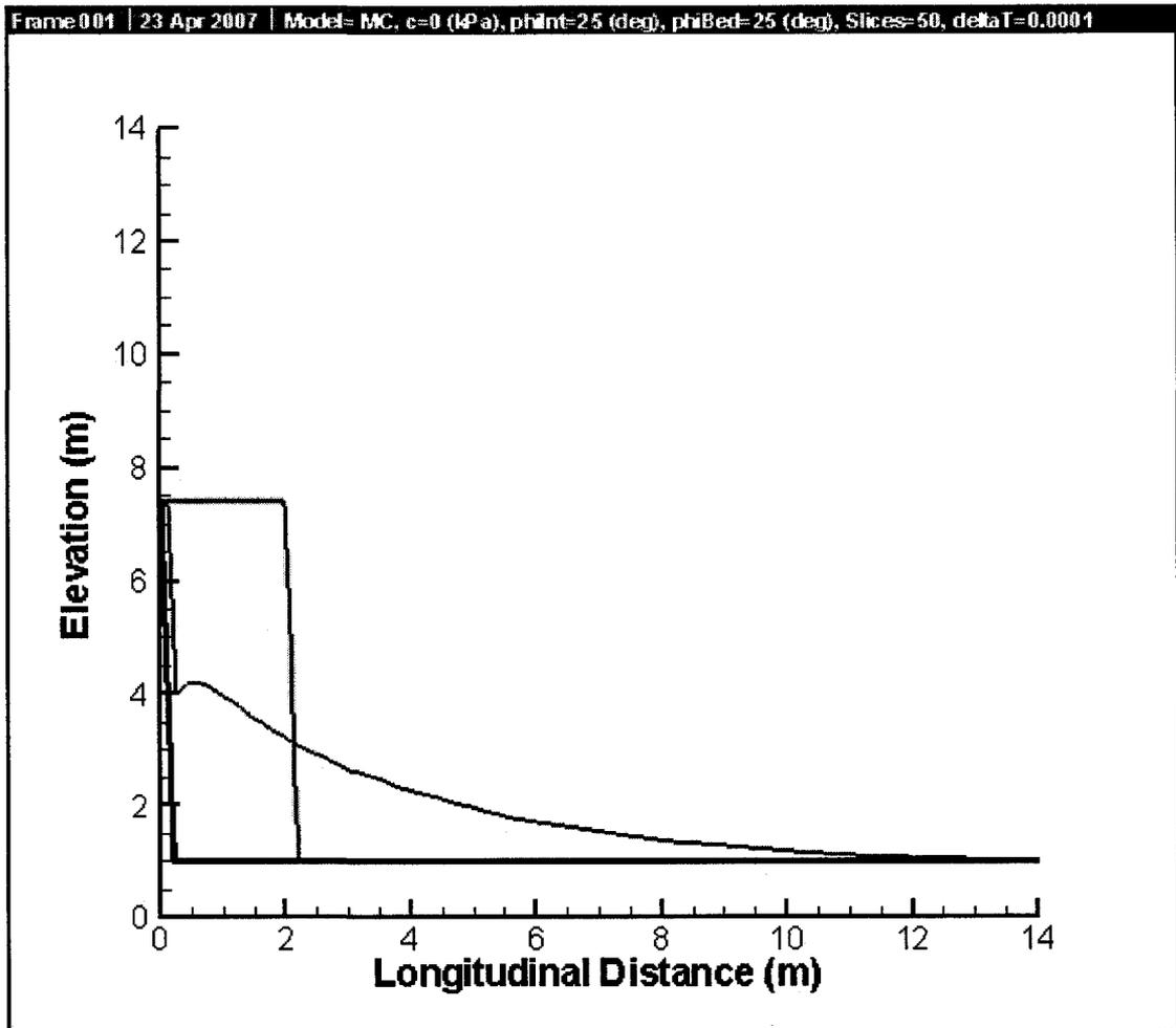
Figure A.14 Simulation of granular spreading mass with initial aspect ratio of 3.2 and height of 6.4 m
