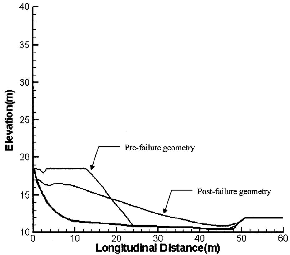
Figure B.80 Geometries of the Route 272 flow slide based on dynamic analysis with the friction model
