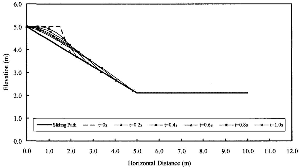
Figure A.3 Flow profiles at 0.2 s interval from hand calculation
