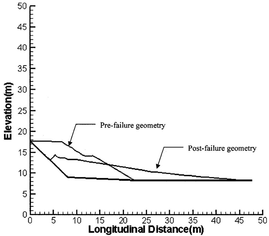
Figure B.70 Geometries of the Shibecha-Cho flow slide based on dynamic analysis with the friction model
