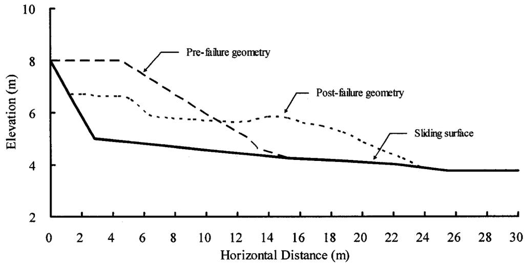
Figure B.88 Geometries of the Hachiro-Gata flow slide used for dynamic analysis
