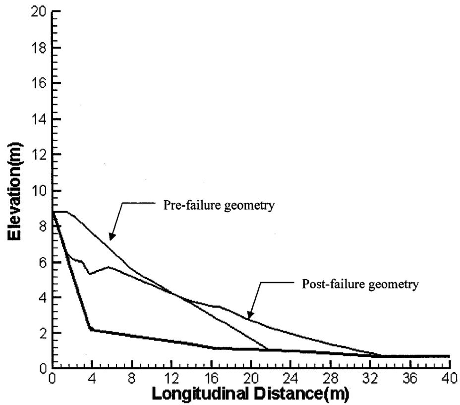
Figure B.39 Geometries of the Lake Ackerman flow slide based on dynamic analysis with the friction model
