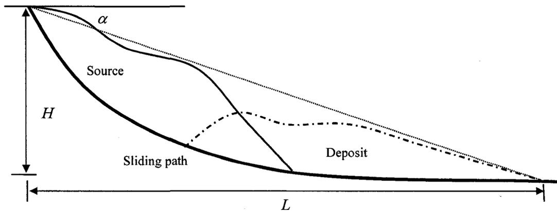
Figure 4-1 Definitions of travel angle and travel distance
