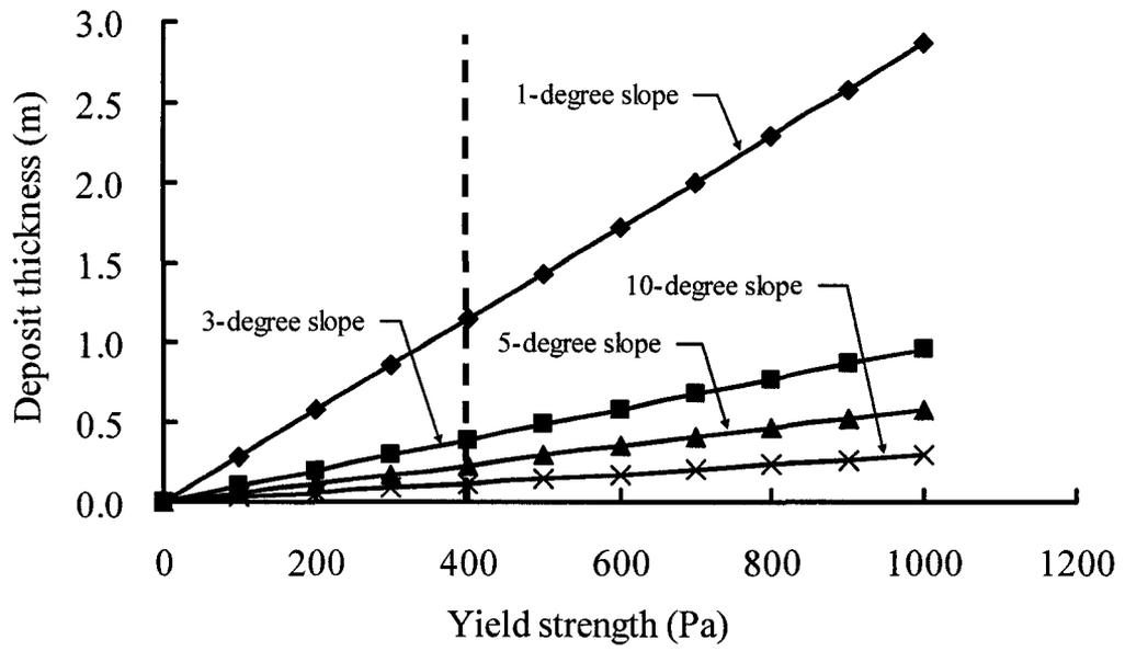
Figure 3-3 Debris flow deposit thickness versus yield strength for different slopes
