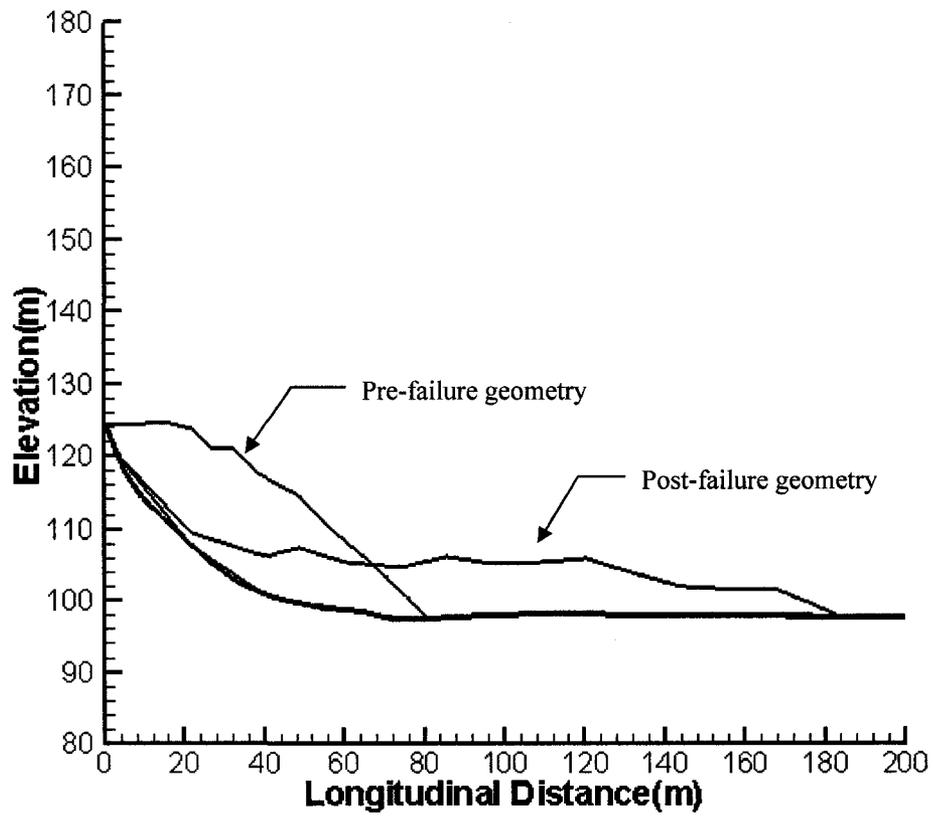
Figure B.12 Geometries of the Wachusett flow slide based on dynamic analysis with the cohesive model
