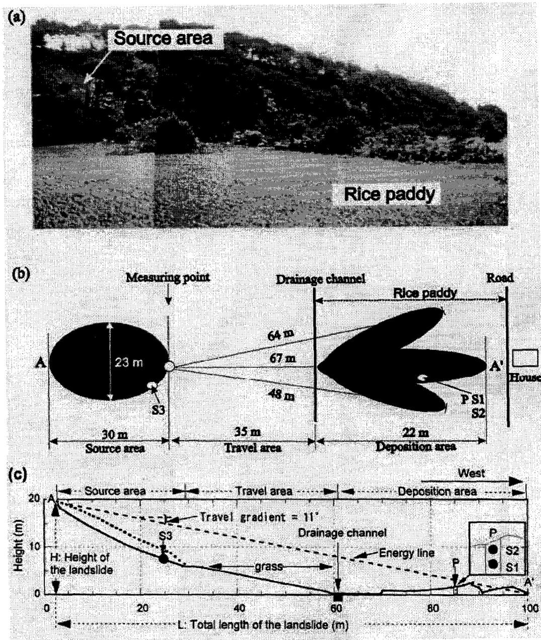
Figure 7-21 The Hiegaesi landslide (After Sassa 2000): (a) Photograph of the landslide; (b) Sketch of the landslide in plan; (c) Longitudinal cross section of the landslide. P: observation pit; S1, S2 and S3: sampling sites.
