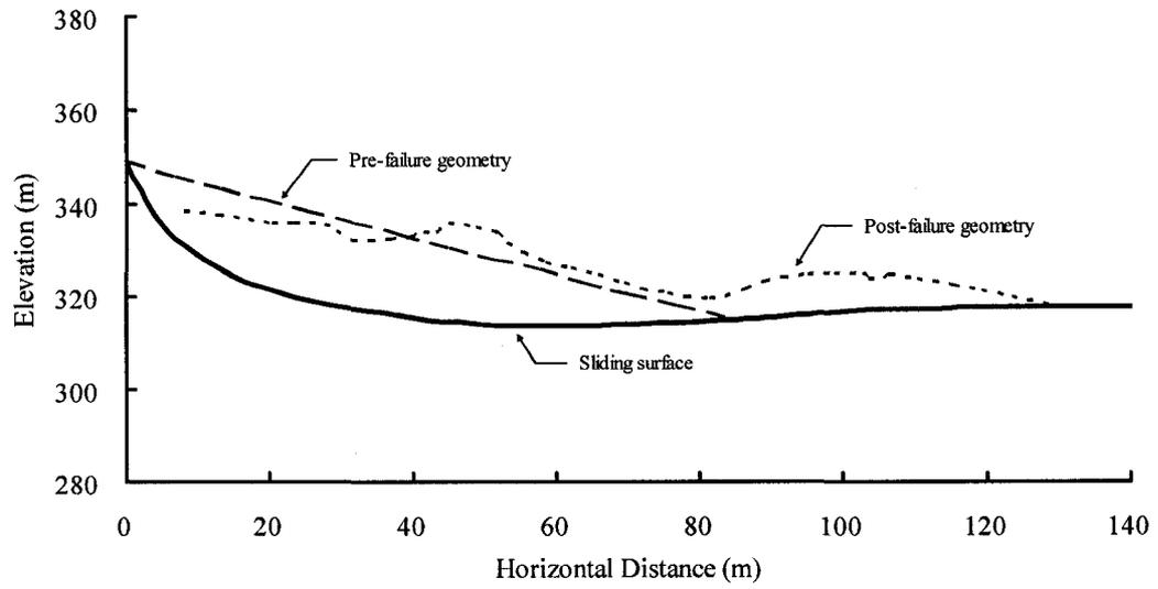
Figure B.3 Geometries of the Lower San Fernando flow slide based on field observations
