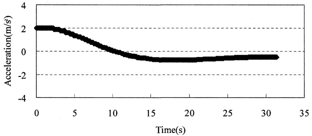
Figure 6-3 Acceleration versus time in analysis with the sliding block model
