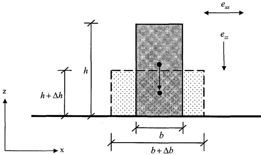
Figure 5-3 Uniform deformation assumed
