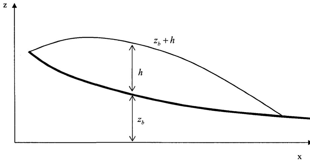
Figure 4-7 Two-dimensional debris flow with Cartesian coordinates
