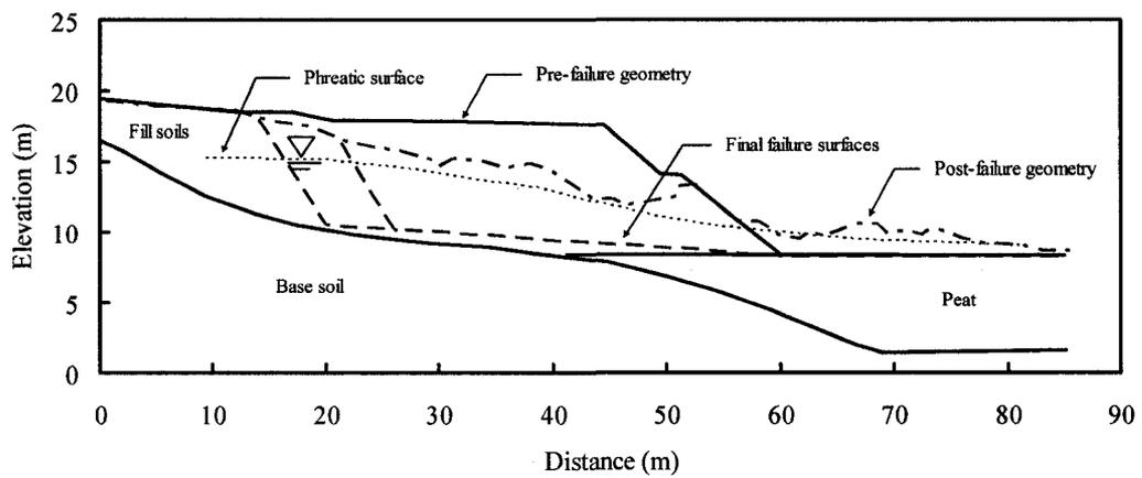
Figure B.66 Post-failure geometries of the Shibecha-Cho embankment used for liquefied shear strength analyses (Modified from Olson 2001)
