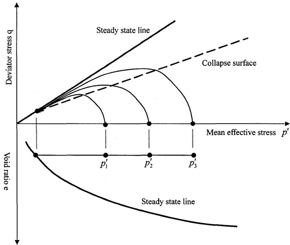
Figure 7-1 Typical isotropically consolidated undrained test on loose sand (Modified from Sladen et al. 1985a)
