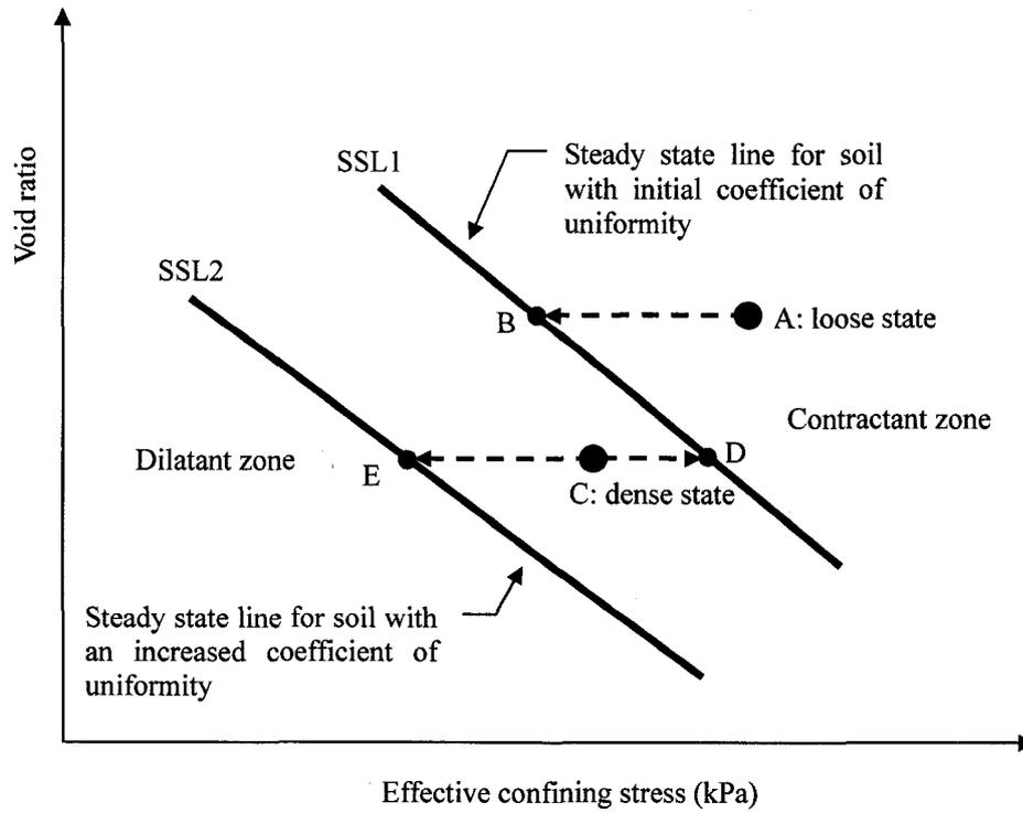
Figure 7-5 Changes in steady-state line associated with natural comminution
