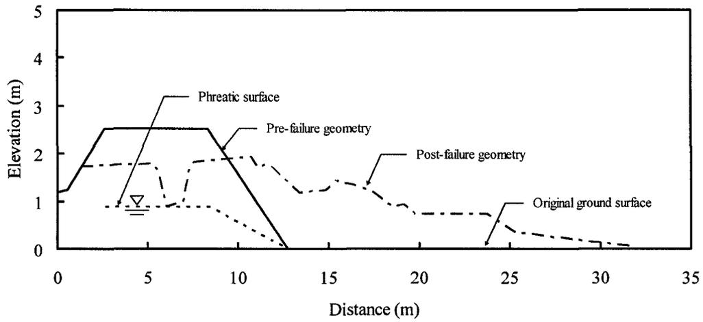
Figure B.43 Pre- and post-failure cross section of the embankment at Koda Numa
