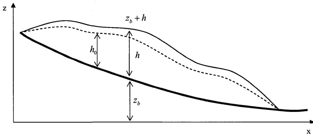
Figure 4-8 Two-dimensional non-Newtonian flow with Cartesian coordinates
