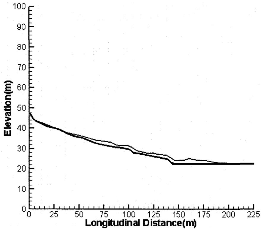
Figure 7-15 Post-failure profile of the Tsukidate landslide based on dynamic analysis
