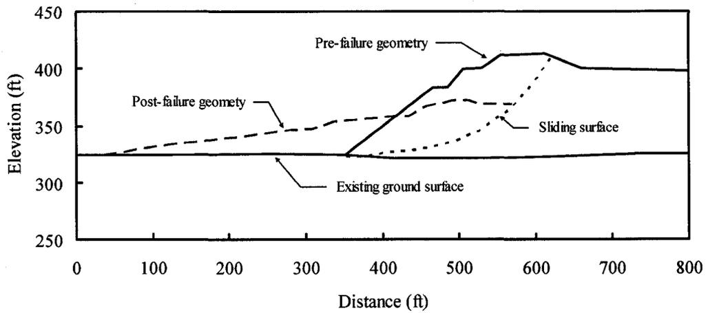
Figure B.10 Pre- and post-failure geometries of the North Dike of the Wachusett Dam
