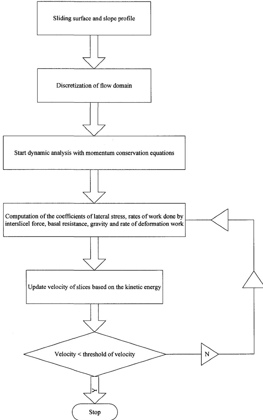
Figure A.1 Flow chart of dynamic analysis based on energy consideration
