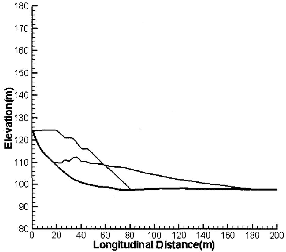
Figure 6-8 Geometries of the North Dike flow slide based on dynamic analysis with the friction model
