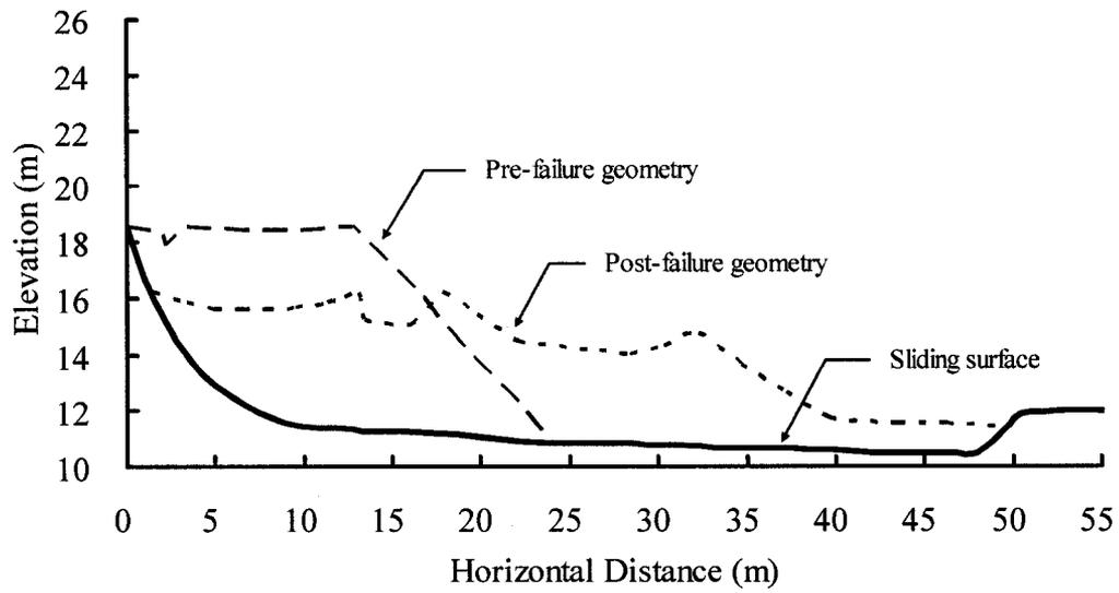
Figure B.78 Geometries of the Route 272 flow slide used for dynamic analysis
