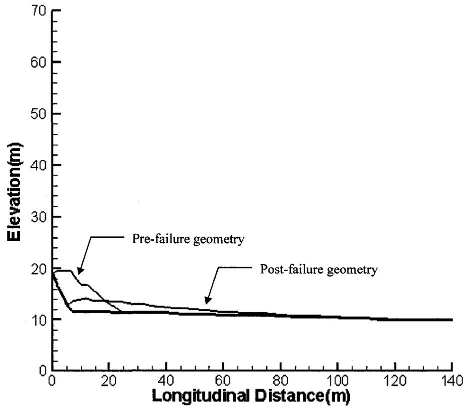
Figure B.59 Geometries of the Uetsu-Line flow slide based on dynamic analysis with the friction model
