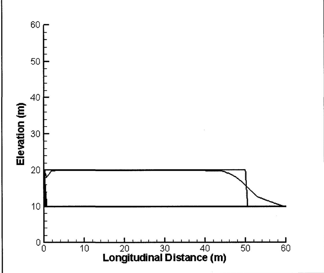
Figure A.9 Simulation of dam-break sand flow with friction model ( $\phi = \phi_b = 30^\circ$ )
