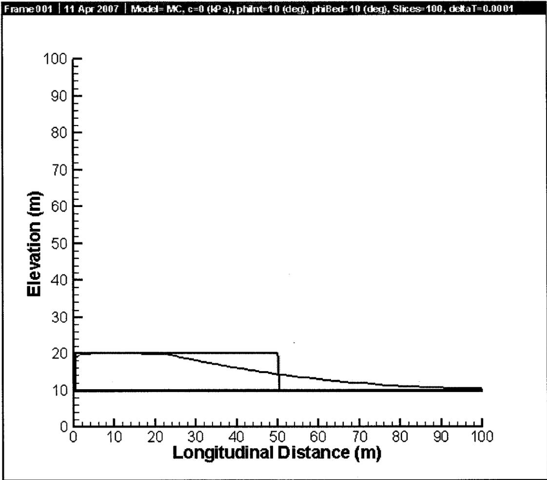
Figure A.11 Simulation of dam-break sand flow with friction model ( $\phi = \phi_b = 10^\circ$ )
