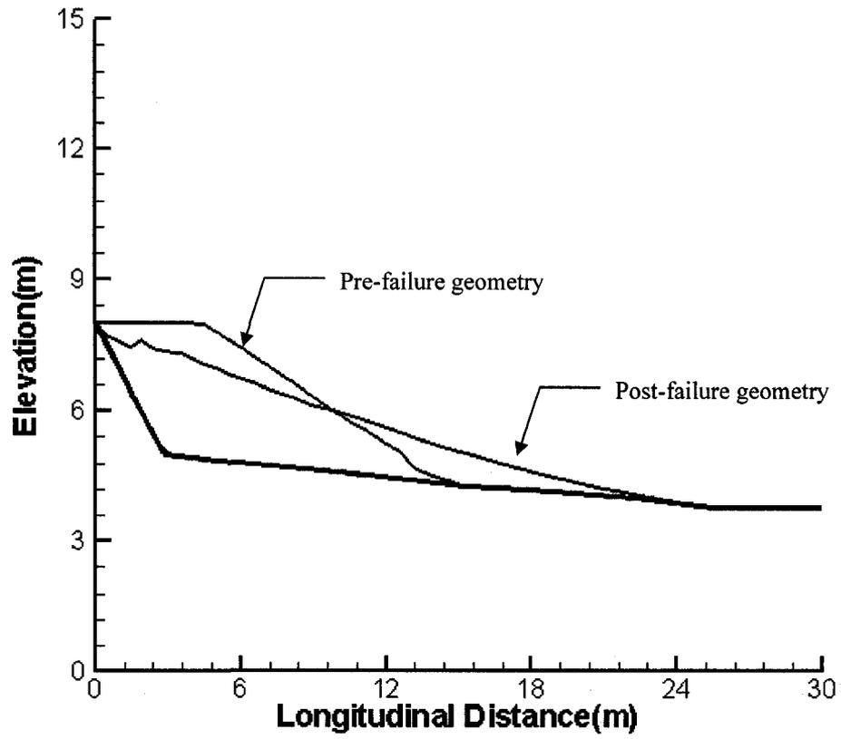
Figure B.90 Geometries of the Hachiro-Gata flow slide based on dynamic analysis with the friction model
