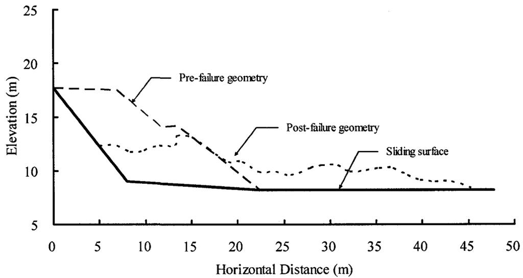
Figure B.68 Geometries of the Shibecha-Cho flow slide used for dynamic analysis
