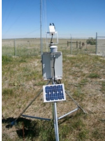
Figure 32 - RSR device for measuring solar radiation [258]
